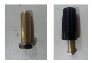
Left: Tighten bolt with washer into the end of the brass bush (note that flanged end at top goes into the reel housing) Next right: drop assembly into handle
