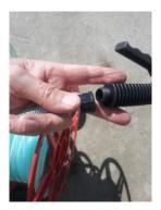
Step 3. Assemble handle – slide handle into holders & secure with threaded bolt
