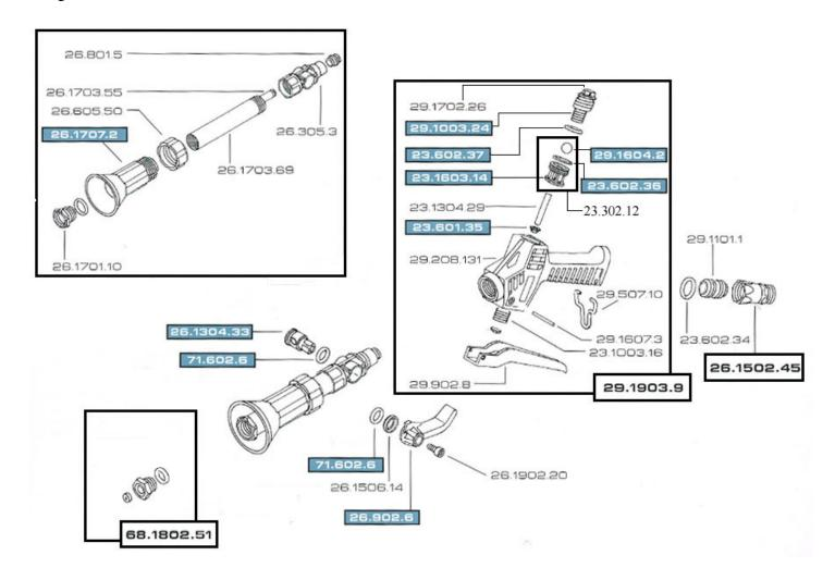
A valve kit for the turbo gun is available for the **B26.901.165** under the following part number **B23.302.6**. A complete repair kit is also available under the following part number **B26.302.6**.
