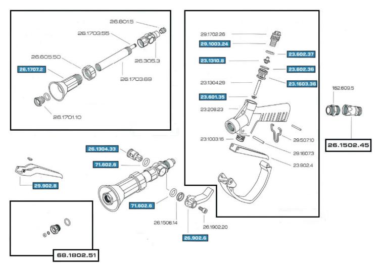
A valve kit for the turbo gun is available for the **B26.901.165MK2** under the following part number **B23.302.6**. A complete repair kit is also available under the following part number **B26.302.6**.
