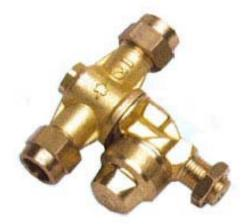
For use on air blast sprayers. Very compact, roll over to select spray tips with two shut off positions. Two open positions at + 15 from vertical. A click point at each position. Check valve assures efficient and long lasting operations at low and high pressures.
