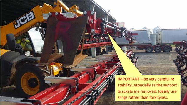
(5) Raise the boom and tow the WEEDit forwards and lower outer boom to a suitable working height.
