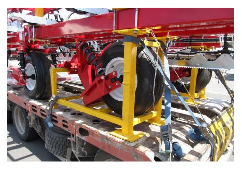
(3) Connect suitable size tractor to WEEDit unit and tow off the truck - **slowly and carefully**. Check the clearance between the spray rails and truck ramps as the machine is unloaded. This is not a 1 man job.
