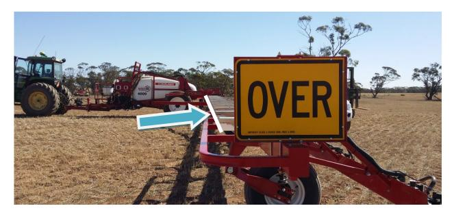
(13) Remove yellow inner pivot brace. Remember to return all "Yellow" Transport kit components, including nuts, bolts and washers to Croplands for credit.
