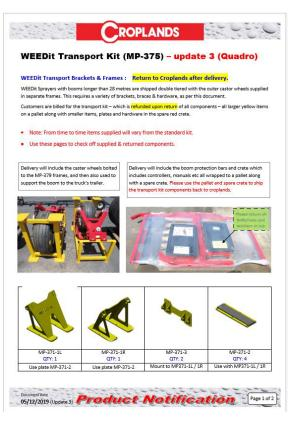
From late 2019 onwards 36m WEED-IT sprayers are being delivered with the castor wheels installed into individual frames which are also used to support the boom to the trailer's bed.
