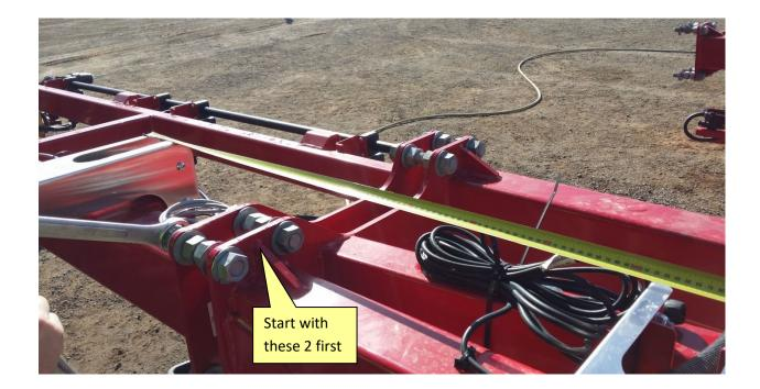
(10) Fit outer castor wheels while outer boom is supported by the forklift. Position as per the diagram below, and is the same for 36, 32 or 30m boom. Note the pivot pin is to the front of the main boom section.
