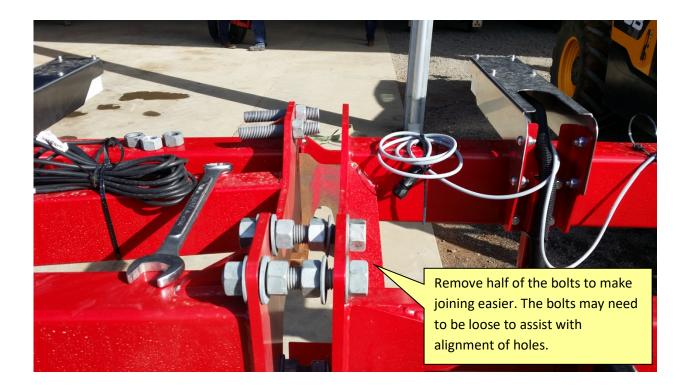
(8) Join boom together. Add all of the bolts and washers leave them loose to assist with the boom alignment.
