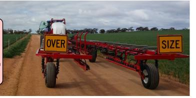
(23) Adjust the drawbar to achieve 1100mm camera height on the central cameras – as a guide, the main chassis sits approximately 6 degrees nose down from horizontal, and the upright tank supports are 90 degrees from horizontal, when correctly adjusted.
