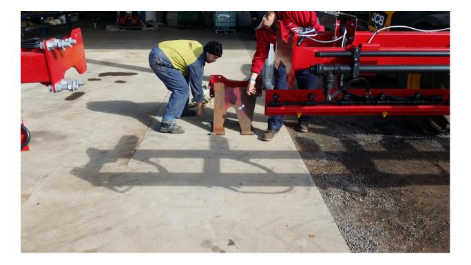
(7) Reverse the WEEDit unit (or very carefully take outer boom to the unit) to connect the booms together.
