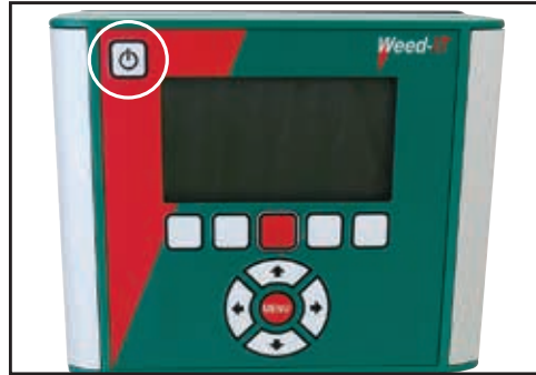
Press WEEDit Controller Power Button to start the air compressor.
