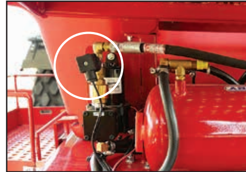
Remove the electrical fitting from the air valve.
