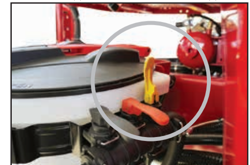
Lift the Hopper Rinse valve to rinse the hopper.
