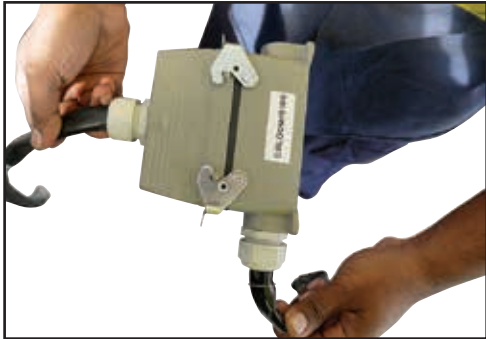
Rotate the clips & lock the connectors in place.
