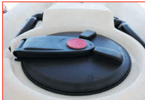
Main tank inspection lid closed & locked.
