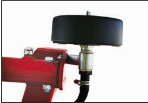
Clean the compressor air filter regularly.
