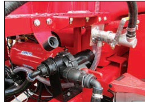
Open the ball valve to fill the hopper.
