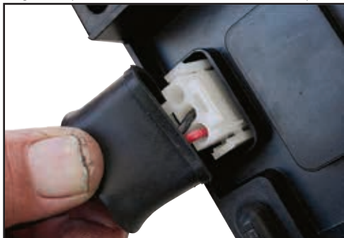
Align, then, push-in the male connector until it clicks in place.
