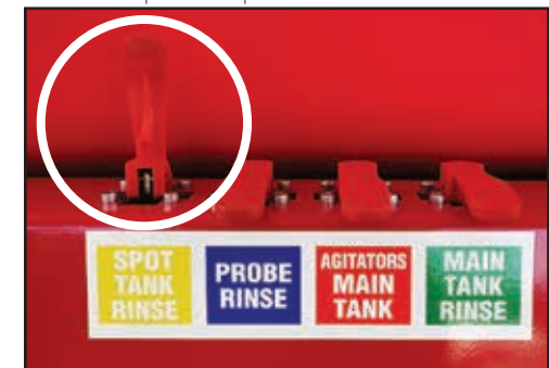
Open the "Spot Tank Rinse" valve.
