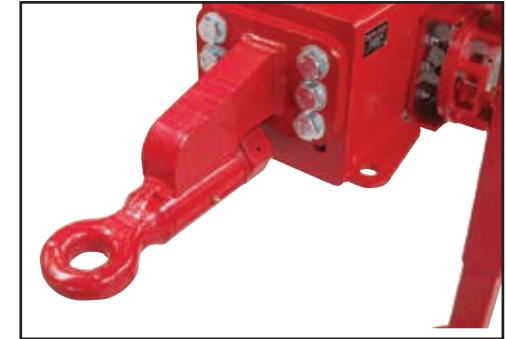
The front drawbar hitch tongue is height adjustable.
