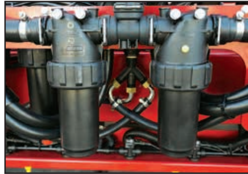
Remove & clean the Spot Sprayline pressure filters.
