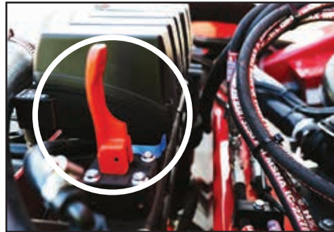
Open the Boom Section Manifold Flush valve.
