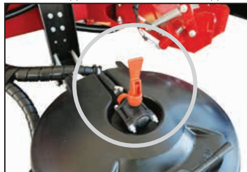
Lift the Hopper Rinse valve to rinse the hopper.
