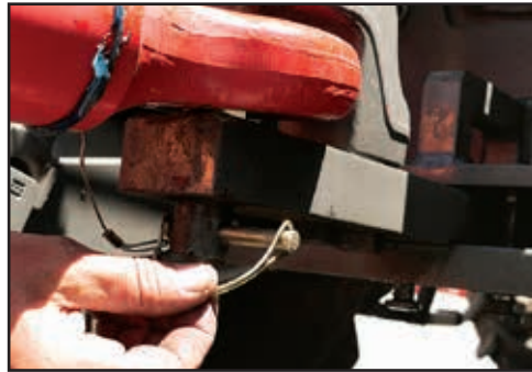
Ensure the drawbar pin is locked-in.
