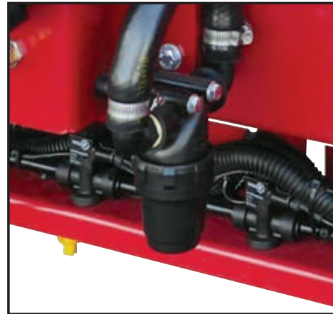
Pressure Filter Blanket Sprayline Centre Boom Section (shown on sprayer)
