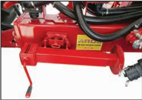
Rotate the hitch jack until it locks into the transport position.
