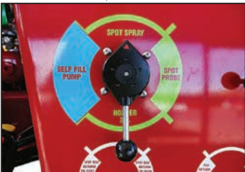
Rotate the Spot Spray valve to the "Spot Spray" position.
