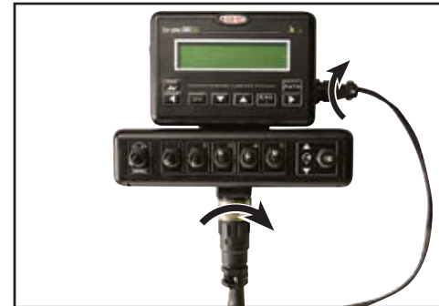
Fit the loom connectors to the Console.
