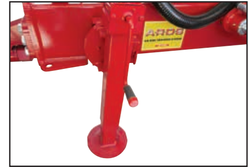
Lock the hitch jack in position, then adjust the hitch height.
