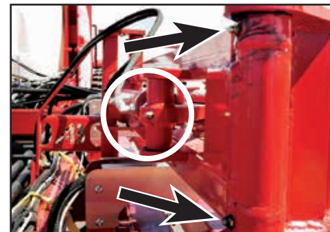
Pivot grease points on the wing stay fold mechanism.
