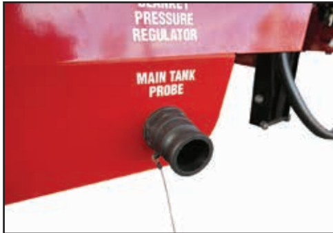
Connect the Probe to the "Main Tank Probe" inlet.
