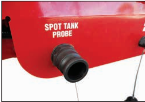
Connect the Probe to the "Spot Tank Probe" inlet.
