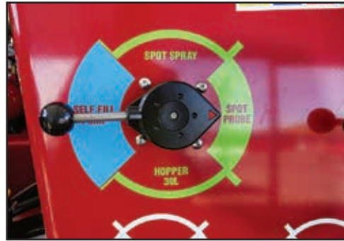
Rotate the Spot Spray valve to the "Spot Probe" position.
