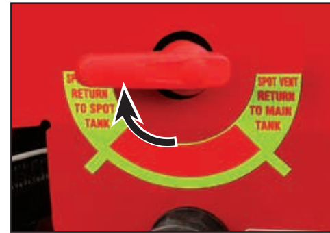
Rotate Spot Vent valve to "Return to Spot Tank" position.
