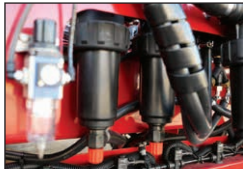
Clean the Blanket Sprayline Pressure filters regularly.
