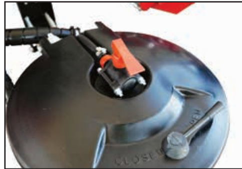
Lower the 60 litre Chem-E-Flush into the filling position.
