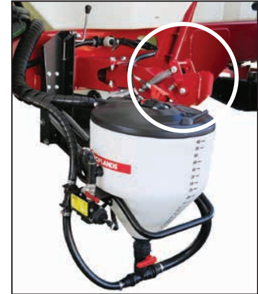
Release & lower the hopper.
