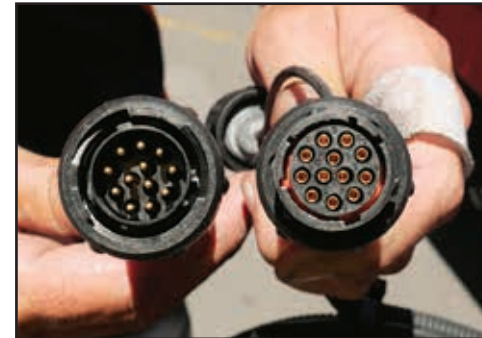
Align the Console loom connectors & push them together.
