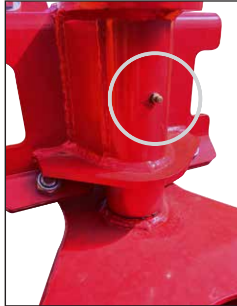
Castor wheel pivot grease point.
