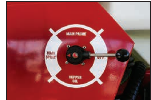
Rotate the Main Spray Valve to Main Spray" position.
