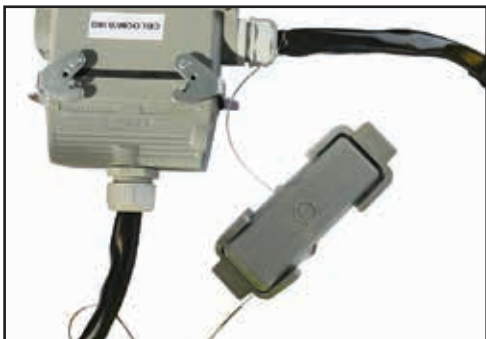
Lock the male & female dust caps together, to keep them clean.
