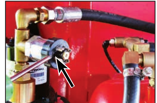
Adjust the level switch (hysteresis) set at 70 psi via the side hole on the valve [shown at end of screwdriver].
