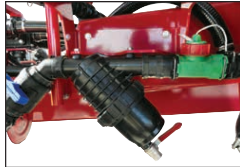
Check the fresh water fill filter is clean.
