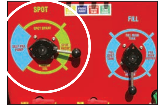
Rotate the Spot valve to "Self-Fill Pump" position.
