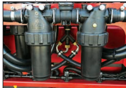
Check the Spot sprayline pressure filters are clean.
