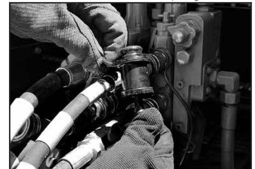
Join the male & female dust caps together.
