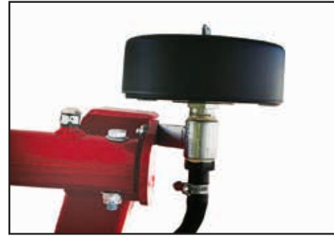
Change the compressor air filter every 200 hours or 6 months.
