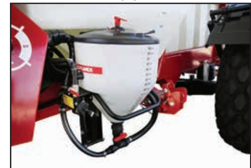
Return the hopper back to its transport position. Push the hopper inwards until the latch mechanism is engaged.
