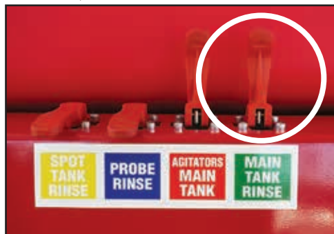
Open the "Main Tank Rinse" valve.
