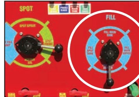
Rotate the Fill valve to "Fill Main Tank" position.
