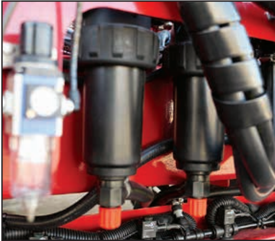
Pressure Filters Optical Spot Sprayline (shown above on sprayer)
