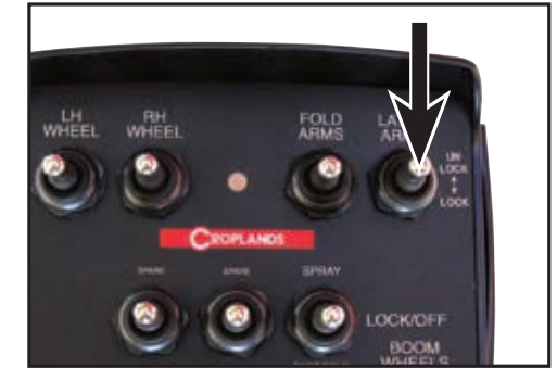
Hold DOWN the LATCH ARMS switch to lock the latches.
