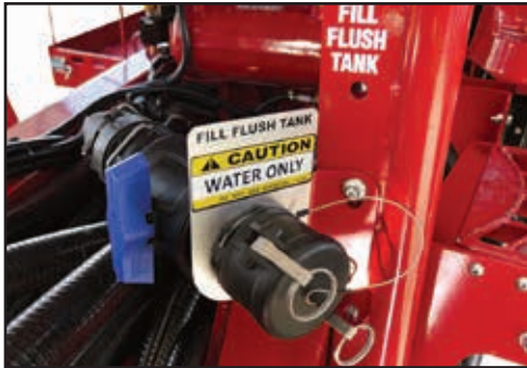
Fill Flush Tank - Water Only connector:
