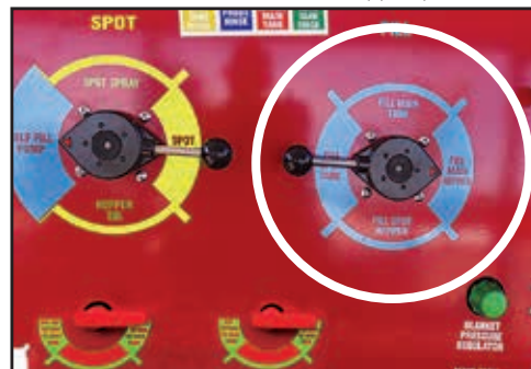
Rotate the Fill valve to "Fill Main Hopper" position.
