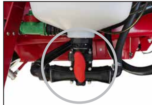
Open the Transfer valve to transfer the mixture.
