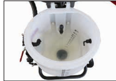
Open hopper lid & add chemical powder/liquid.
