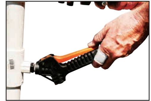
Open the Probe Rinse gun to rinse the container.
