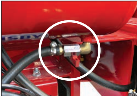
Regularly open the valve to drain water from the air tank & regulators.
