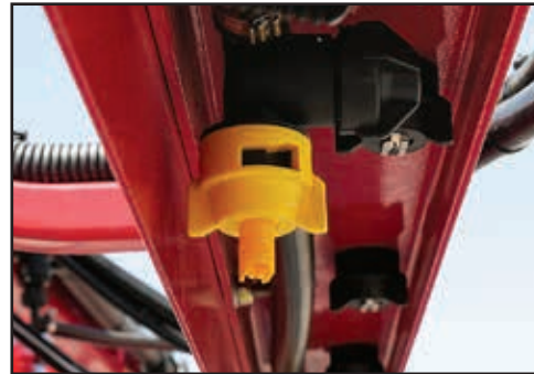
Clean Blanket sprayline nozzle filters regularly.
