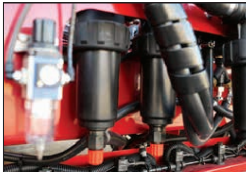
Remove & clean the Blanket sprayline pressure filters.
