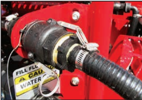
Connect the Envirodrum coupling to the flush fitting.
