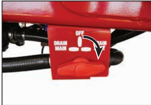
Open the Main Tank Drain valve to drain the tank.
