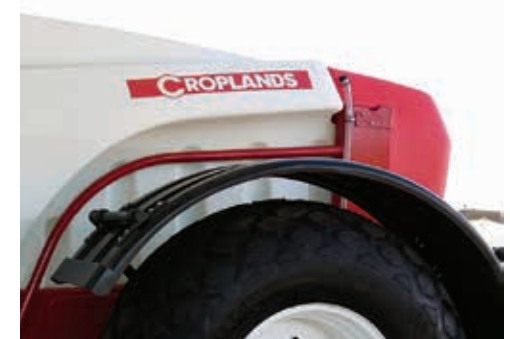
The red coloured Flush tank at the rear of the sprayer.
