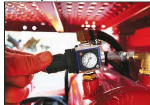
Adjust the ARDS drawbar airbag pressure to 40 psi using the pressure adjustment valve.
