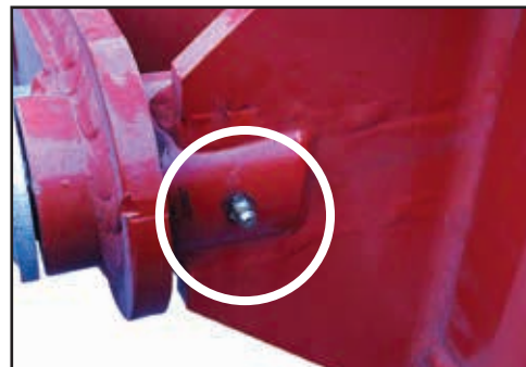
Left grease point of the main boom hinge.
