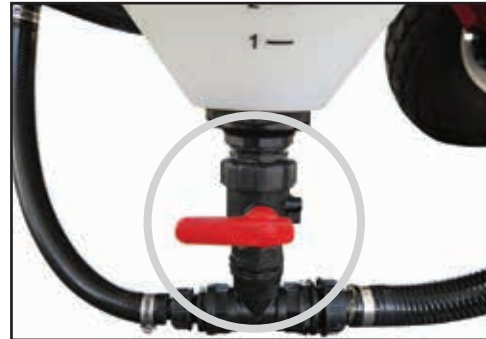
Close the Transfer valve at the base of the hopper.
