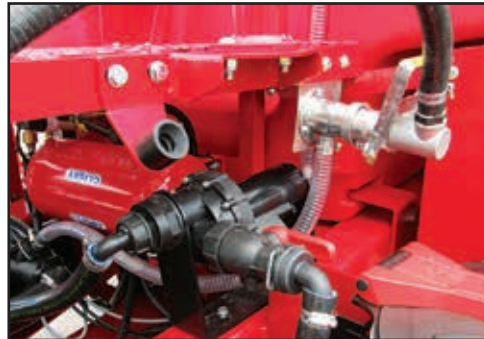
Attach the chemical transfer hose to the Camlock fitting.
