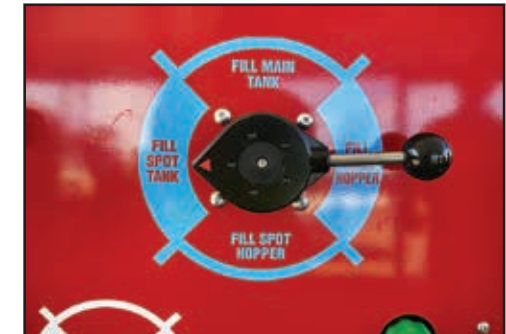
Rotate the Fill valve to "Fill Spot Tank" position.
