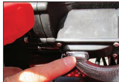
Turn the pump "On" to start & "Off" at completion.
