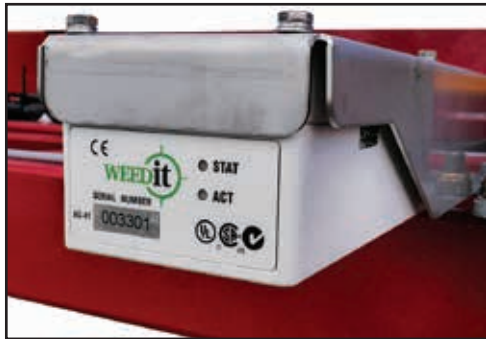
Base of WEEDit camera must be set 1100mm above the ground.
