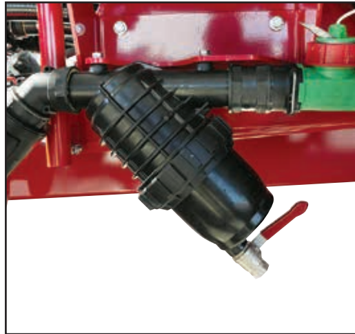
Bottom-Fill Filter (shown above on sprayer)
