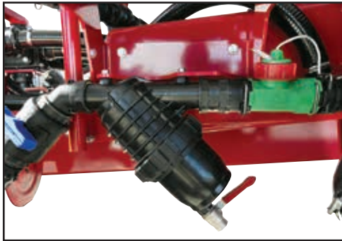
Clean the Fresh Water Fill filter regularly.
