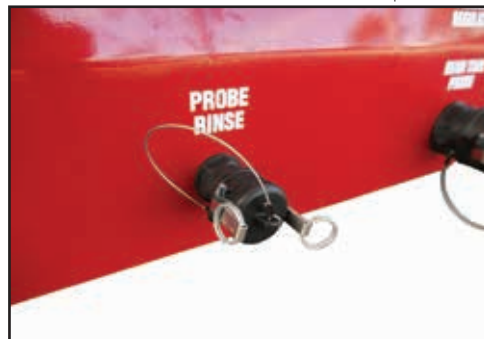
Refit the Probe Rinse connector cap.
