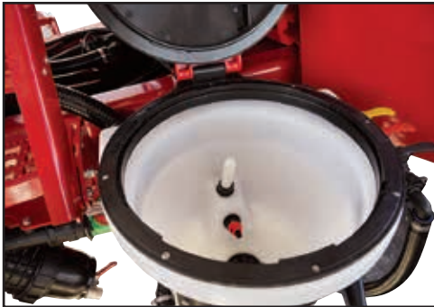
Open hopper lid & add chemical powder/liquid.
