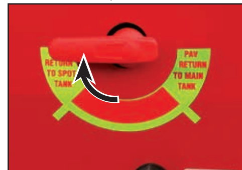
Rotate the PAV valve to the "Return to Spot Tank" position.
