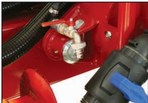
Fresh water tap located at the front of the sprayer.
