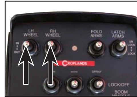
Hold UP both LH & RH WHEEL switches & slowly drive the sprayer forwards.
