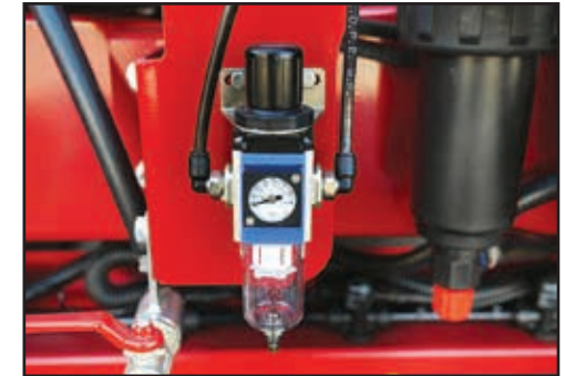
Adjust the air pressure at the rear of the Sprayer.
