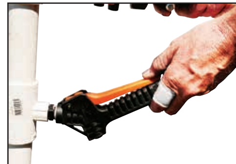
Open the Probe Rinse gun to rinse the container.
