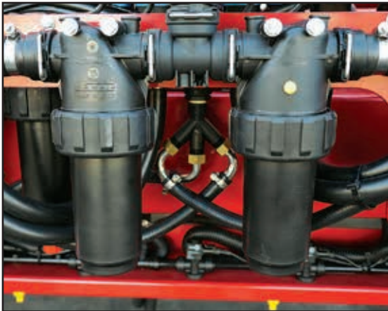
Pressure Filters Blanket Sprayline (shown on sprayer)
