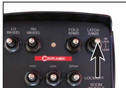
Hold UP the LATCH ARMS switch to unlock the boom stay arm latches.
