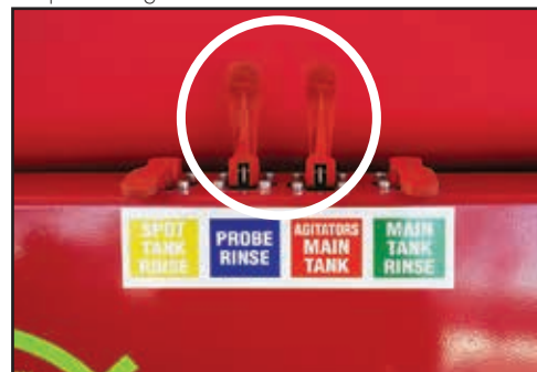
Open the "Agitators Main Tank" & "Probe Rinse" valves.
