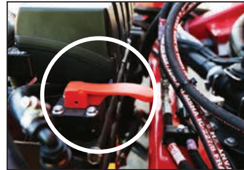
Close the Boom Section Manifold Flush valve.
