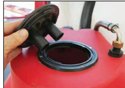
Open the Spot tank lids for inspection.
