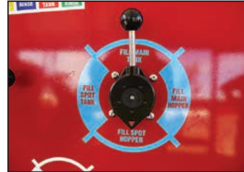
Rotate the Fresh Water Fill Valve to "Fill Spot Hopper" position.
