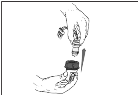
Separate the sensor from the Rapid Check unit.
