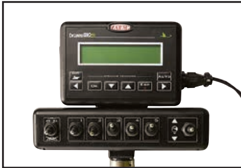
Turn the spray boom sections ON.
