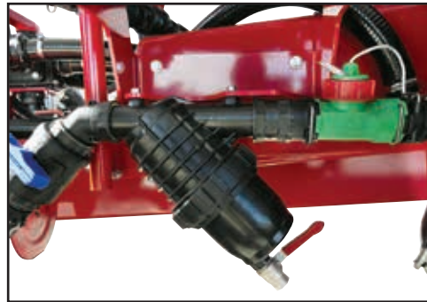
Clean the Fresh Water Fill filter regularly.
