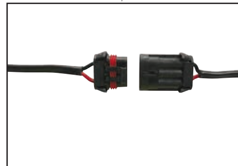
Connect the Console power loom connectors.
