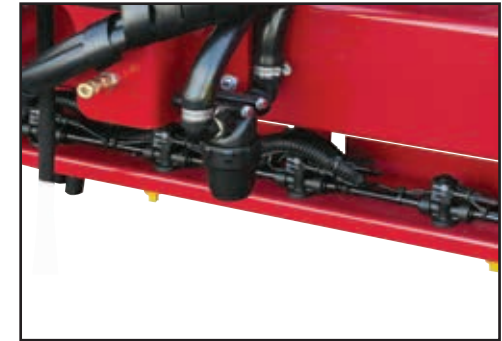
Check the centre-section Spot sprayline pressure filter is clean.
