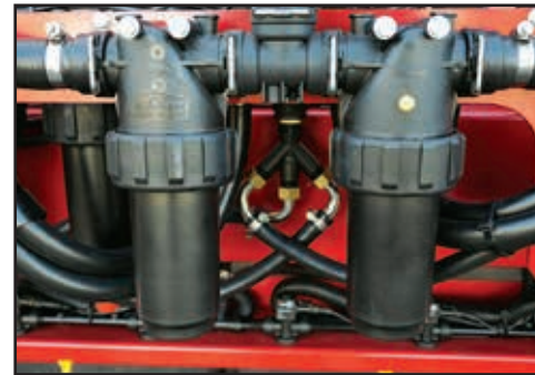
Remove and clean the pressure filters.
