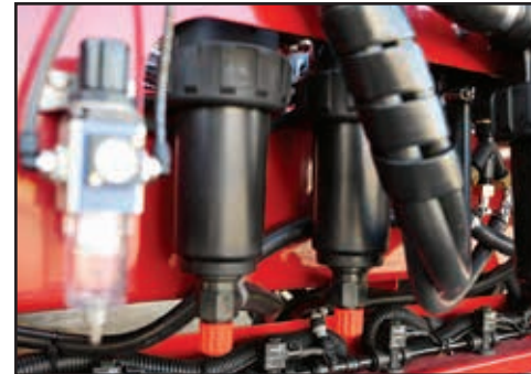
Check the Optical Blanket sprayline pressure filters are clean.
