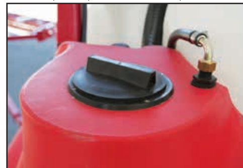
Replace Spot tank lids after inspection.
