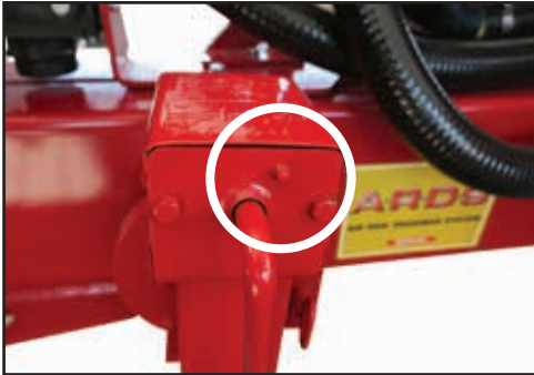
Hitch jack mechanism grease point.
