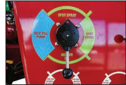
Rotate the Spot Spray valve to the "Spot Spray" position.
