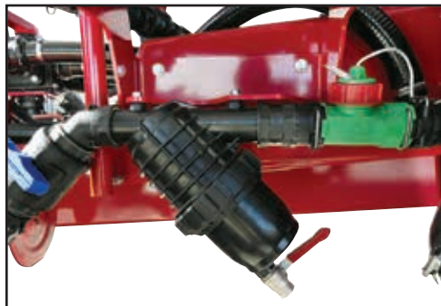
Clean the Remote Fill filter regularly.
