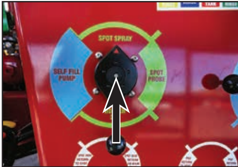
Rotate the Spot Spray Valve to "Spot Spray", then, open the "Agitators Main Tank" valve.
