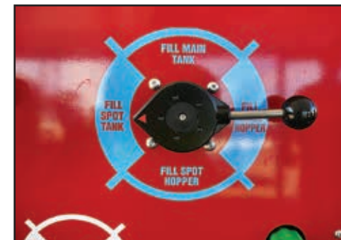
Rotate the Fill valve to "Fill Spot Tank" position.
