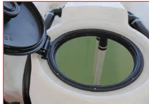
Open the Main tank lid for inspection.
