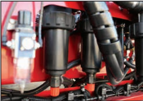
Clean the Blanket sprayline pressure filters regularly.
