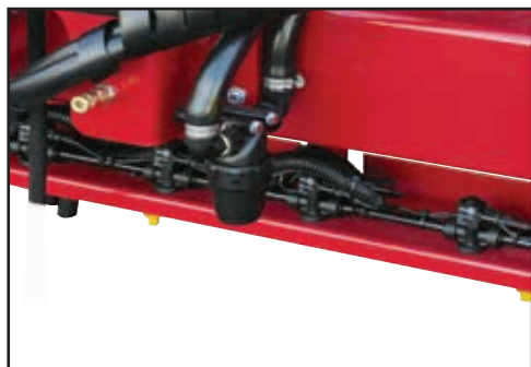
Clean the centre-section Spot Sprayline pressure filter.
