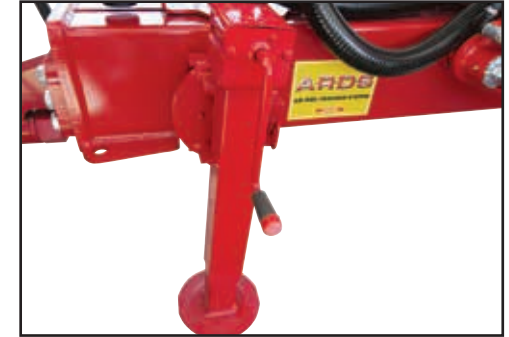
Using the hitch jack, adjust the hitch tongue to the level of the tractor drawbar.
