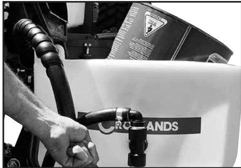
Open the hopper lid & place the container over the drum rinse valve.
