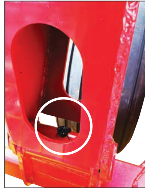
Castor wheel pivot grease point.
