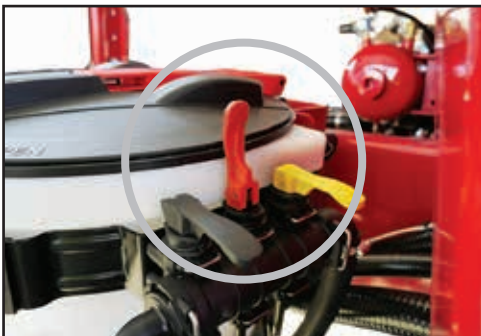
Close the lid & open the Fill valve to add water and mix the chemical.
