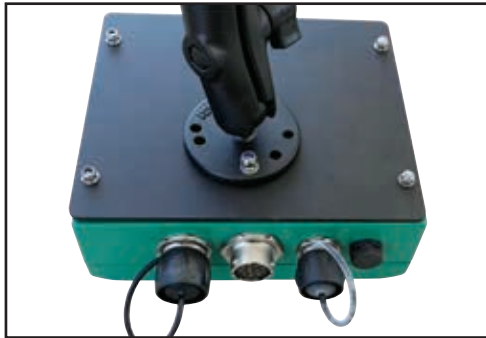
Fix the mounting plate to the Console.
