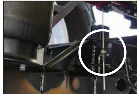
To adjust axle ride height loosen the hose clamp, slide the control rod up or down, then, retighten the clamp.
