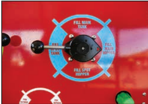
Rotate the Fresh Water Fill Valve to "Fill Main Hopper" position.
