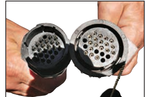
Align the Power loom connectors & push them together.
