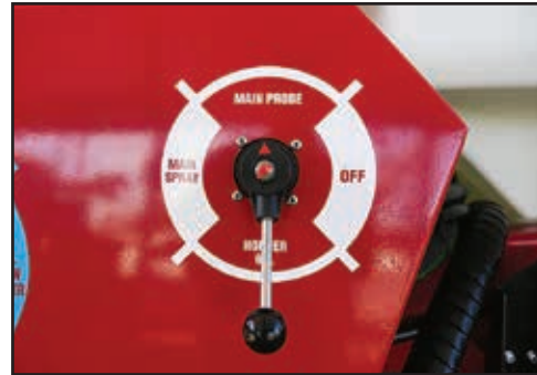
Rotate the Main Spray valve to the "Main Probe" position.
