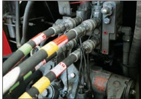
Disconnect hydraulic hoses.
