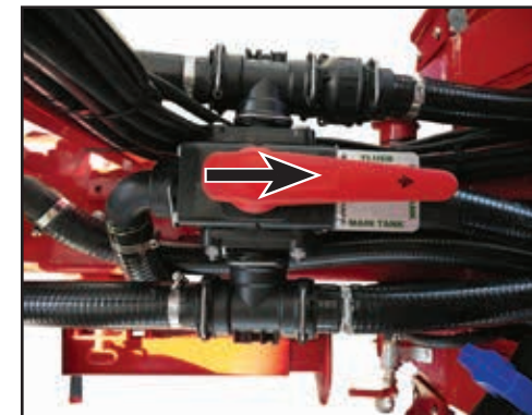
Place the suction valve in "Spot Tank" position.
