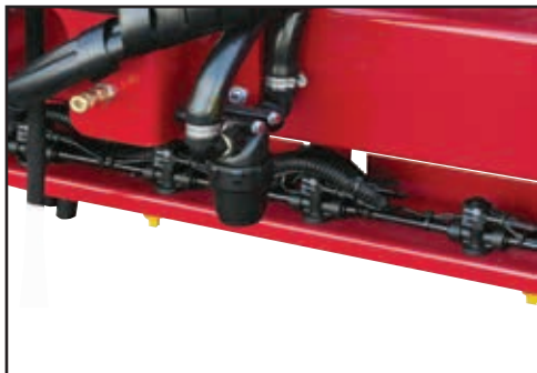
Clean the centre-section Spot Sprayline pressure filter.
