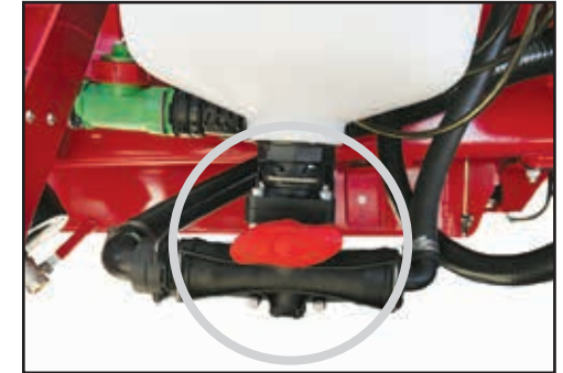
Close the Transfer valve at the base of the hopper.
