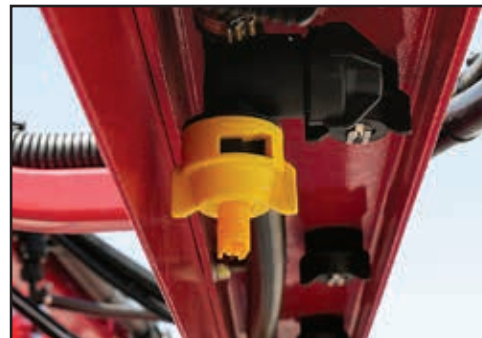
Clean Blanket sprayline nozzle filters regularly.
