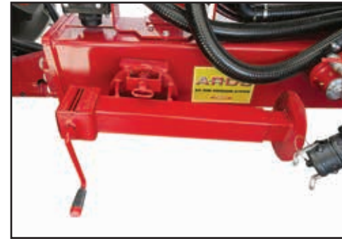
Unpin & rotate the hitch jack down.
