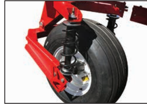
First set tyre pressures to 15 psi, then, adjust the shocker pressures to achieve 1100mm camera height.
