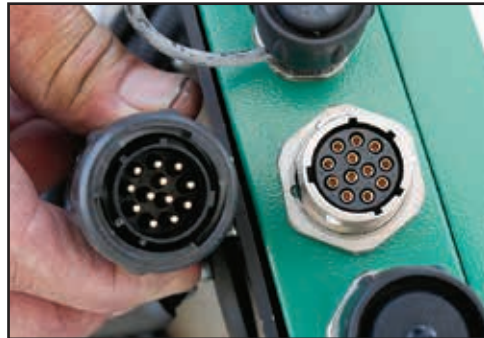
Align the loom connectors & push them together.
