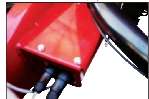
Camera sensor located on the chassis at the rear of the 7000 litre sprayer.
