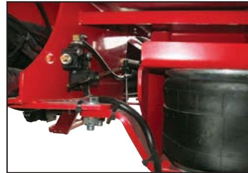
The ARDS drawbar inflatable airbag mechanism.
