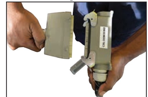
Align the female & male connectors & push them together.
