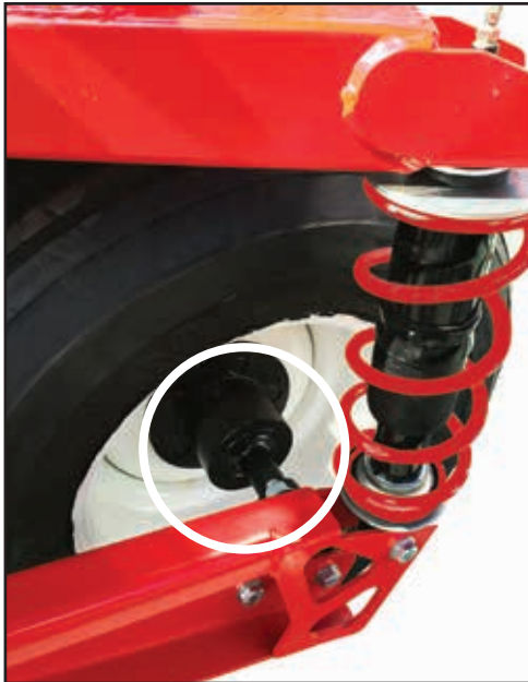
Fully sealed castor wheel hub bearings.
