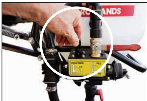
Lift the Drum Rinse valve to rinse the container.
