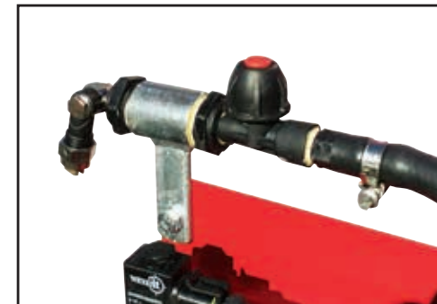
Clean Fenceline nozzle filters regularly (if fitted).
