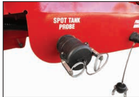
Refit the Spot Tank Probe connector cap.
