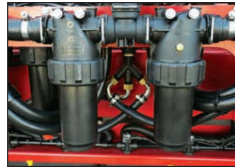
Clean the Optical Spot sprayline pressure filters regularly.
