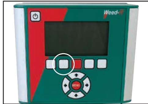
Press the Flush Button to flush & check pressure.
