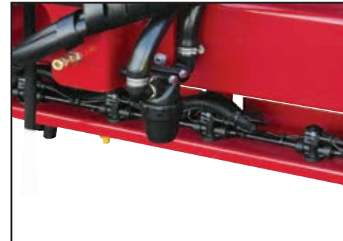
Check the Spot sprayline centre-section pressure filter is clean.
