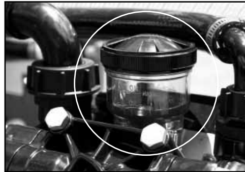
Check the pump oil level.
