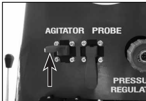
(3) Check the Agitator Valve is open.
