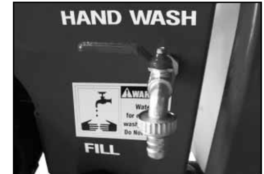
Fresh Water/Hand Rinse Tap - located above the Bottom Fill Inlet.
