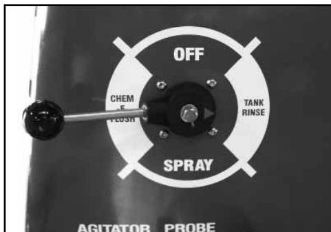
(5) Turn the Function Selector valve to "Tank Rinse".
