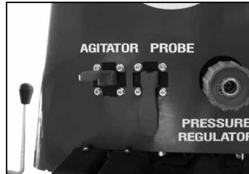
Tank Agitator & Probe Valves - located on lower left hand side of the manual control panel.
