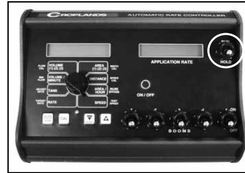
(8) Place the Master switch "On".
