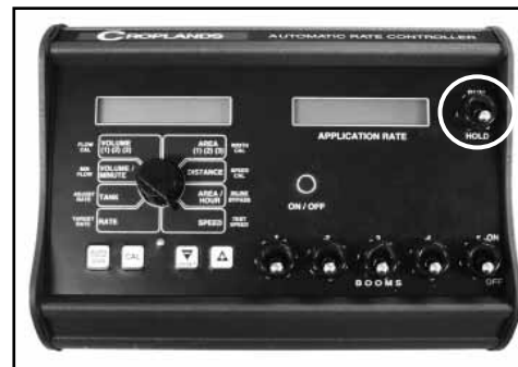
(8) Place the Master switch "On".
