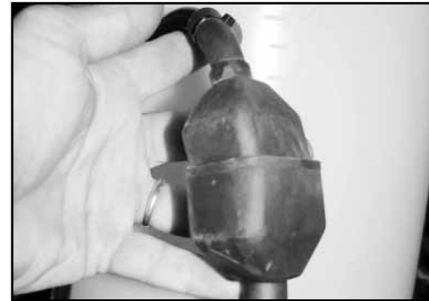
Connect the loom plugs.
