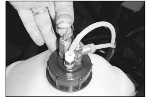
Always release air-pressure in the tank before undoing the cap to refill, and when finished for the day.
