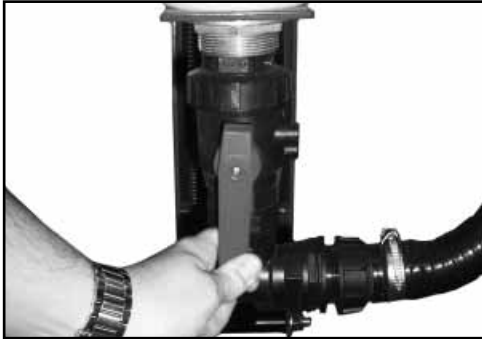
(m & o) Open Transfer valve to transfer mixture to the main tank.
