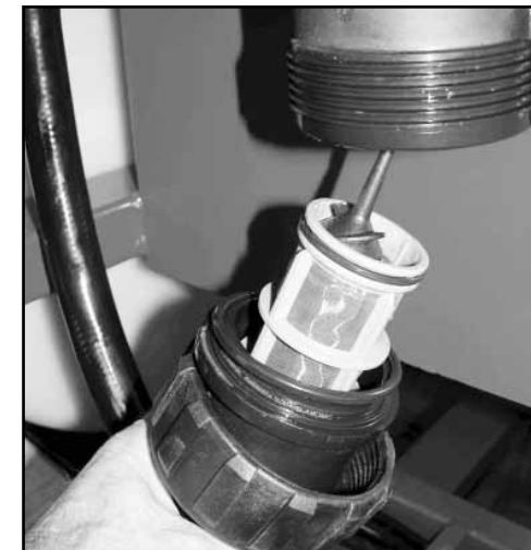
Clean the pressure line filter regularly.
