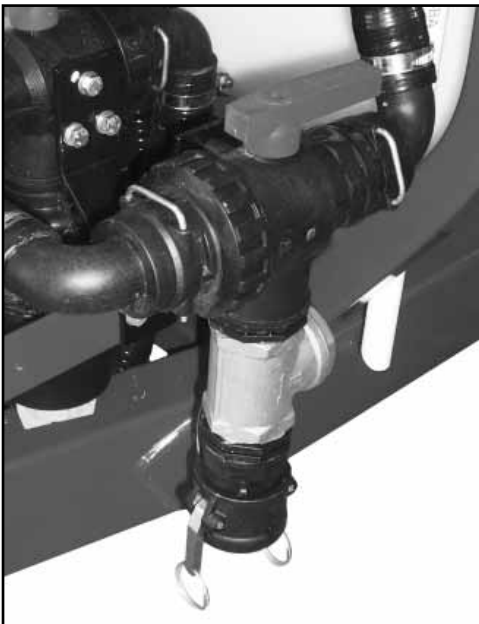
Bottom Fill Inlet - located at front of the main tank on the left hand side.
