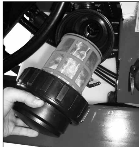
(3) Remove & clean the suction filter regularly.
