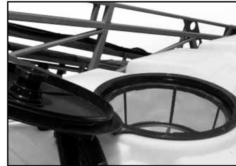
Open the main tank lid for top-filling.
