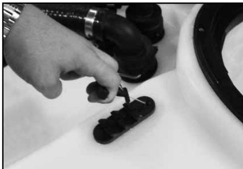
(2) Pull & lock the tank drain valve open to drain the main tank.
