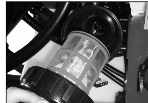
(13) Remove & clean the suction filter.
