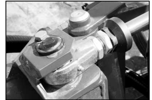
Adjust the cylinder rods.
