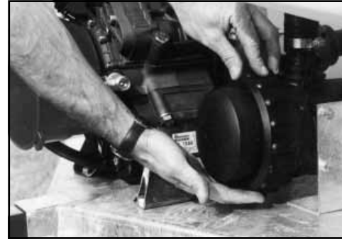
Reassemble & tighten the outer screw of suction filter..
