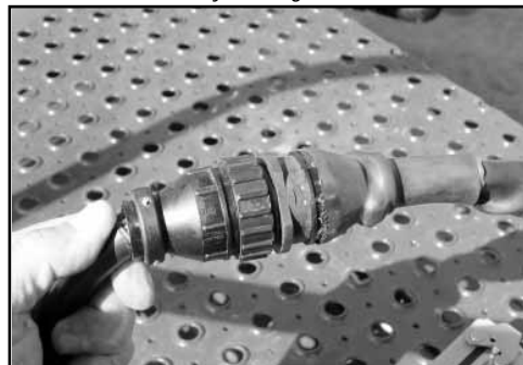
Push the electric/hydraulic connectors together until they lock together.
