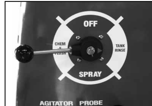
Function Selector Valve - located on top left hand side of the manual control panel - sets the following functions:
