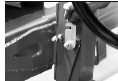
(b) Unlock the Chem-E-Flush dropdown leg lock.
