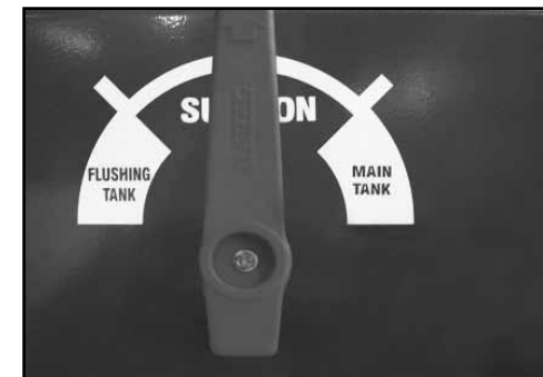
(12) Turn the Suction Selector valve to "Off" position.
