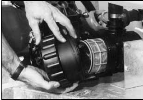
Remove the outer screw and bowl of suction filter.
