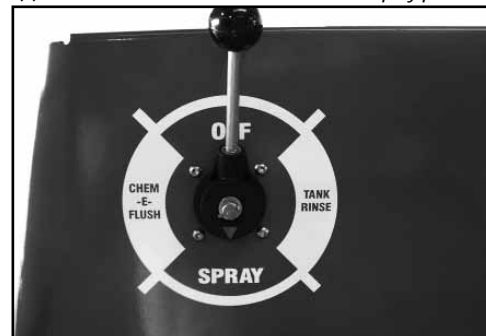
(4) Check the Function Selector Valve is in Spray position.
