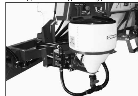
(c) Lower the hopper to filling position.
