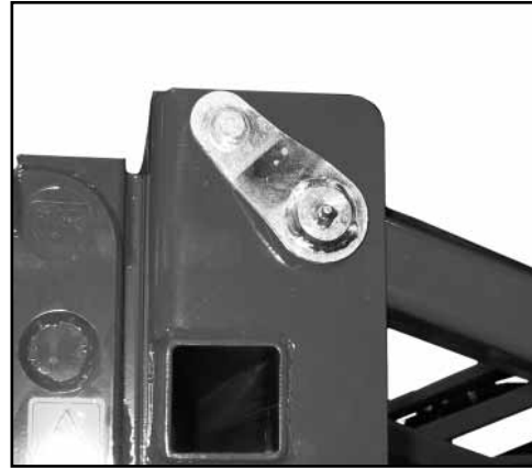
6 Grease the boom parallelogram lift & suspension pivot points.
