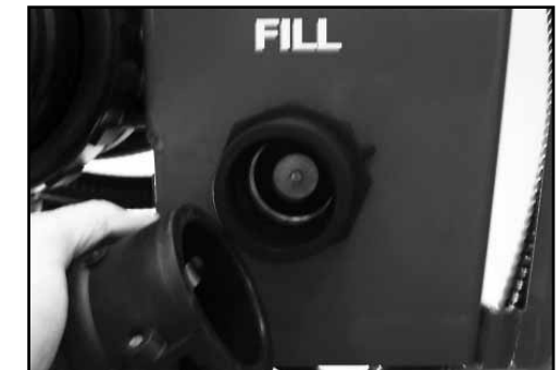
Bottom Fill Inlet - located beside the suction filter.
