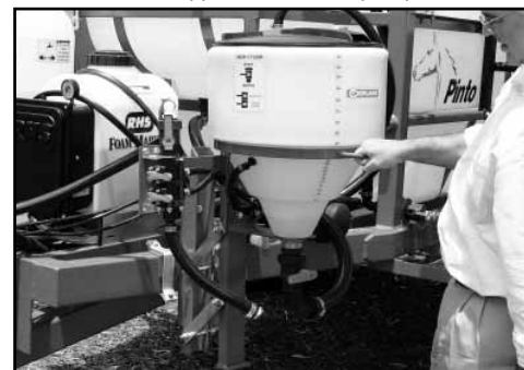
(r) Lift the hopper back to transport position.
