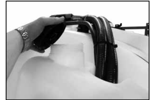
(1) Unscrew the tank lid for filling (3000 litre).
