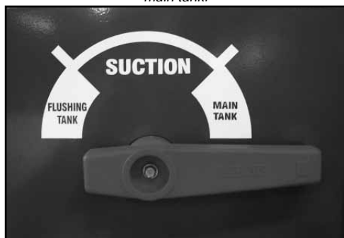
(3) Turn the Suction Selector Valve to source from the main tank.
