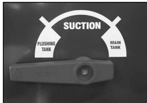
(3) Turn the Suction Selector Valve to source from the flush tank.
