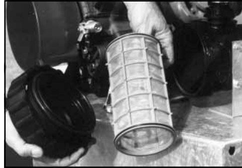
Remove & clean the filter element & components.
