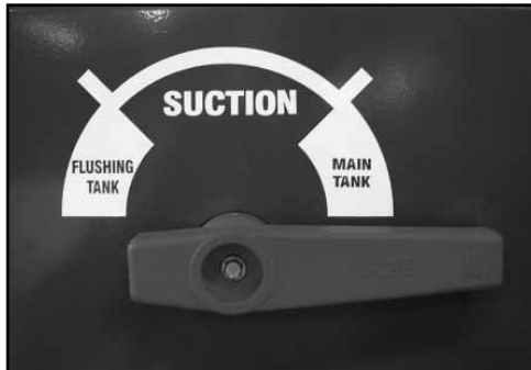
(b) Turn the Suction Selector Valve to source from main tank.
