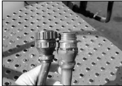
Connect the electric/hydraulic console cables at rear of the tractor.
