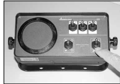
(7) Pressurise the system by placing the Master switch in ON position.
