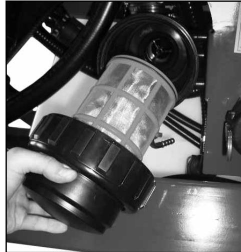
(3) Remove & clean the suction filter regularly.
