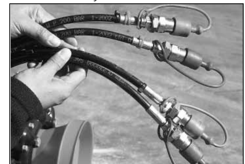
Disconnect hydraulic hoses & PTO shaft.
