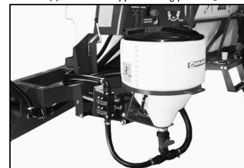
(c) Lower the hopper to filling position.
