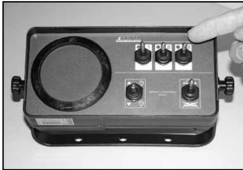
(10) Turn the boom switches On & Off to check operation.
