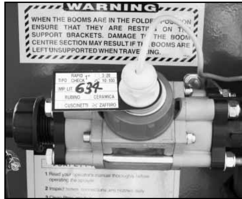
Clean the Rapid Check Flowmeter.
