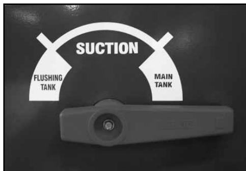
(e) Turn the Suction Selector Valve to source from main tank.
