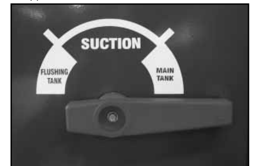
(2) Turn the Fill Selector Valve to the main tank.
