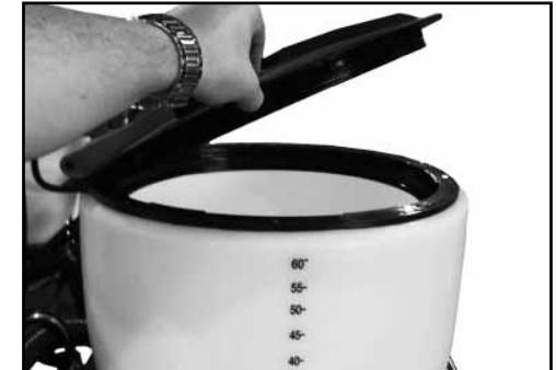
(i) Open hopper lid & add chemical powder or liquid.
