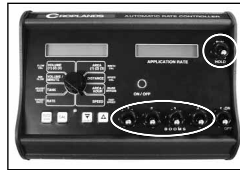
Boom switches Off; Master switch in Hold.
