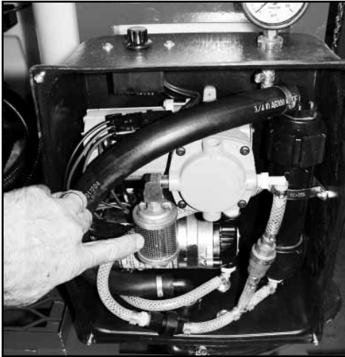
Clean the air filter regularly.
