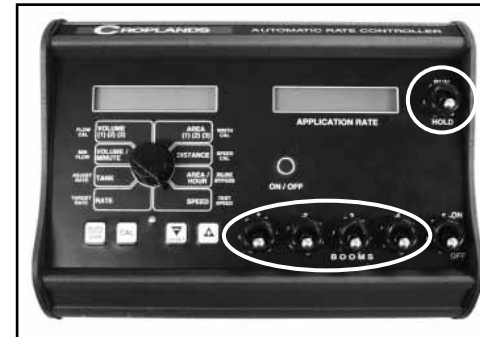
Boom switches Off; Master switch in Hold.
