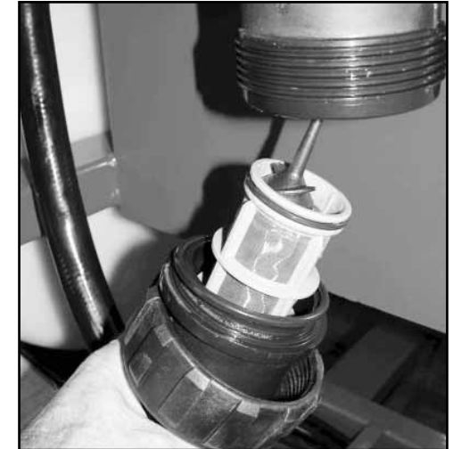
Clean the pressure line filter regularly.
