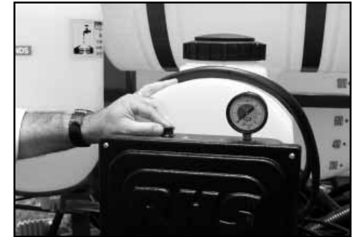
Check the foam marker operates correctly.
