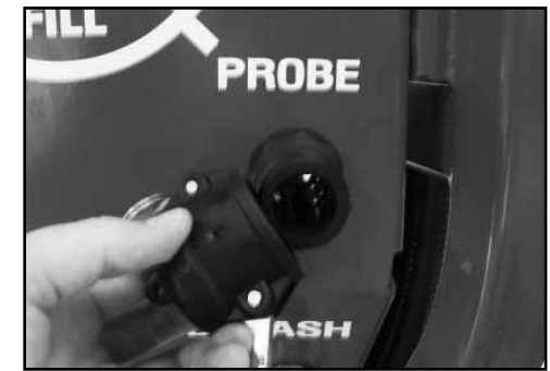
(b) Remove the end cap from the Probe inlet.
