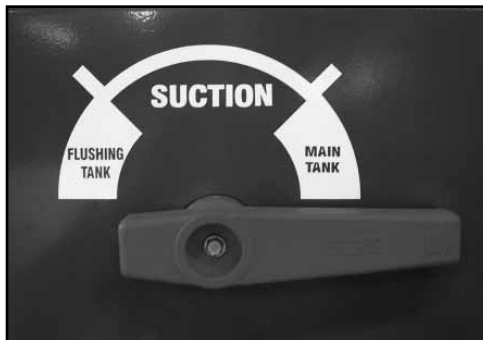
Suction Selector Valve - located on top right hand side of the manual control panel.
