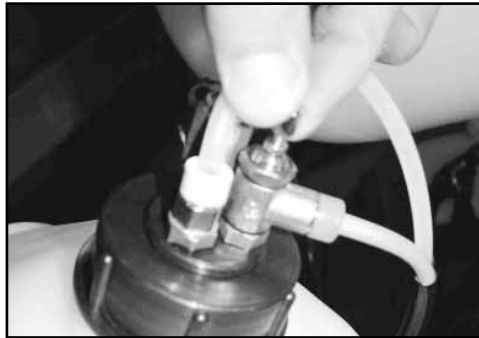
Adjust the foam output with the flow-rate regulating valve.
