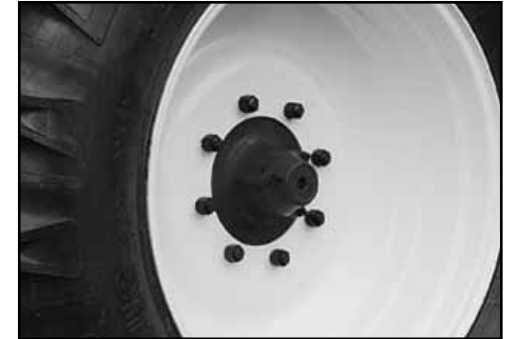
Repack the wheel bearings at 200 hours.
