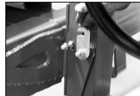
(b) Unlock the Chem-E-Flush dropdown leg lock.
