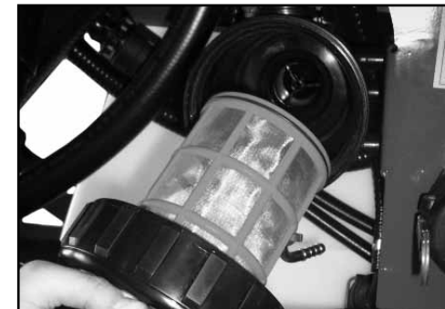
(13) Remove & clean the suction filter.
