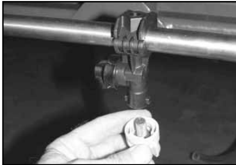
Clean the nozzle filters regularly.
