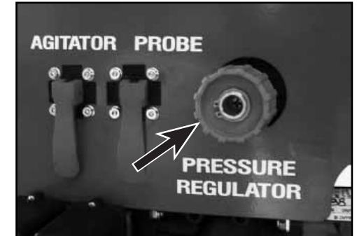
(8[d]) Adjust the Pressure Regulator valve.
