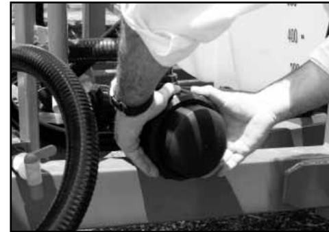
Check the suction filter is clean.
