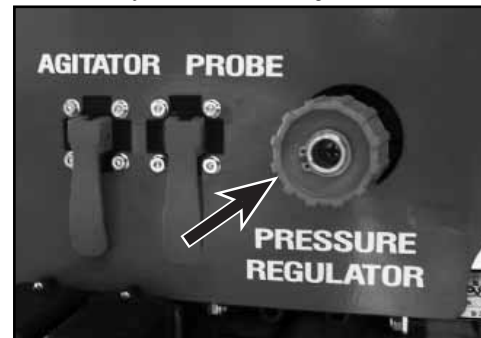
(8) Adjust the Pressure Regulator valve.
