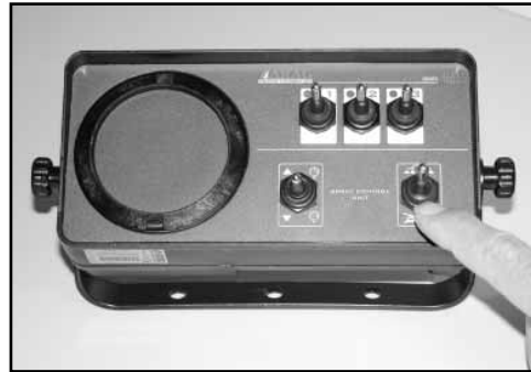
(13) Check & adjust the pressure with boom sections On.
