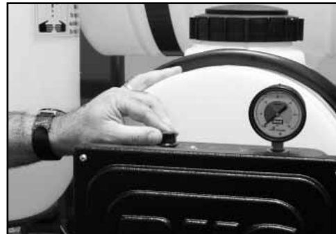
The foam marker adjustment knob & pressure gauge.
