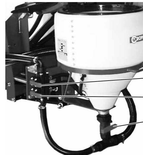
Fill Selector Valve - located on lower right hand side of the manual control panel.
