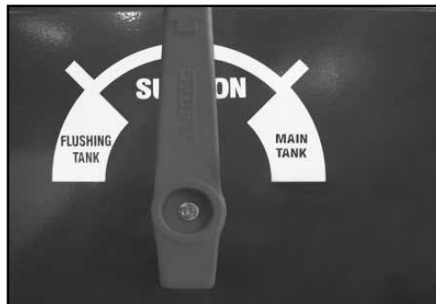
(2) Turn the Suction Selector Valve to "Off" position.
