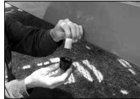
After cleaning, replace the screen & filter bowl.
