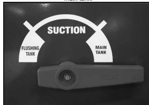
(4) Return the Suction Selector Valve to source from main tank.
