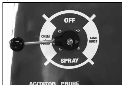
(4) Turn the Function Selector valve to "Tank Rinse".
