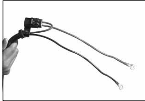
Connect the main harness cables to the battery.
