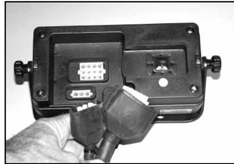
Connect the leads to the rear of the console.
