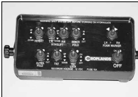
Electric/hydraulic control console.
