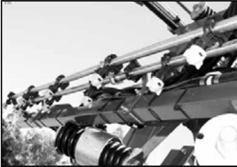
Dual lines on the boom.
