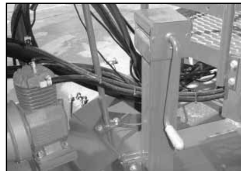
Adjust the hitch jack until the work platform is level.
