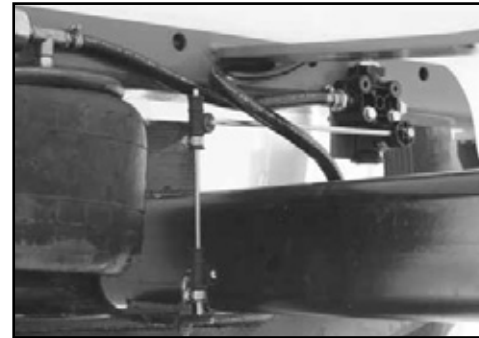
Air levelling valve with adjustable linkage.
