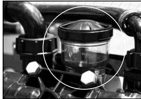
Check pump oil level.
