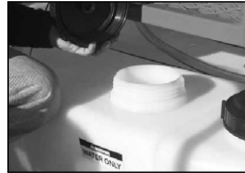
Open Flush tank lid for top-filling.
