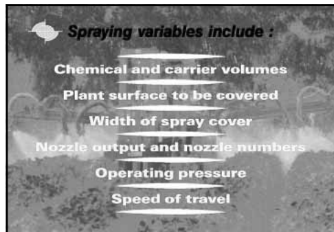
Proper calibration considers all spraying variables.
