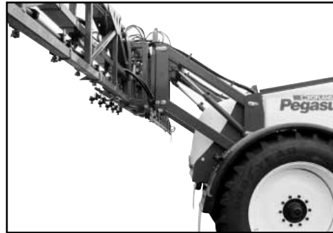
Unique parallelogram boom lift - high position.
