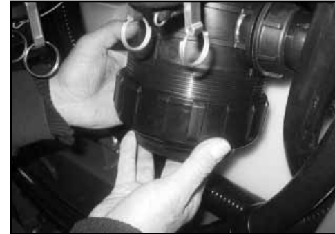
Reassemble & tighten outer screw of suction filter.
