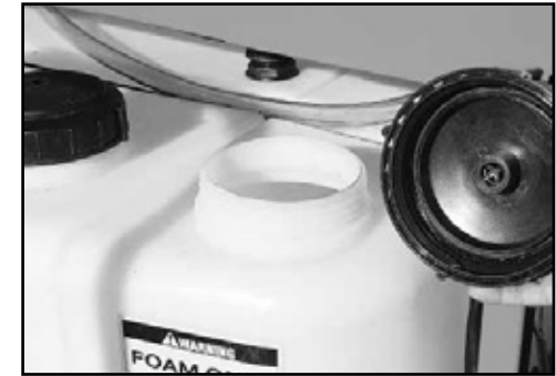
Open Foam tank lid for top-filling/adding concentrate.
