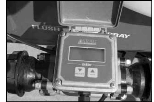
Orion filling flow-meter.
