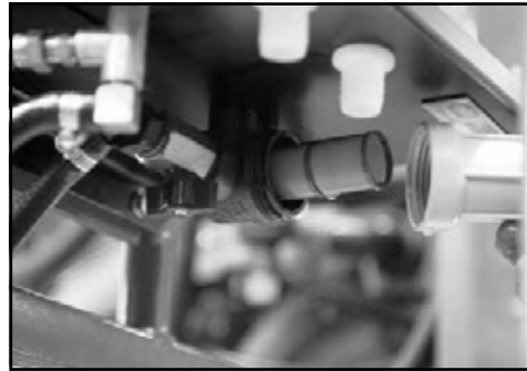
Regularly clean the foam marker filter.
