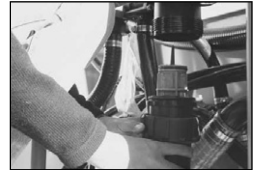
Remove and clean the pressure filter
