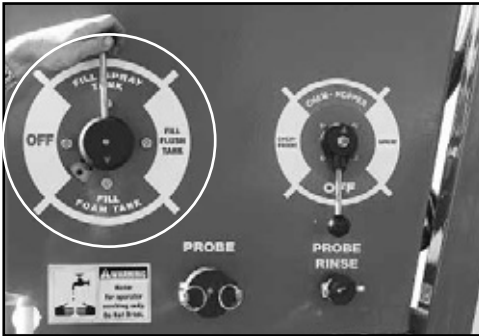
Rotate the Fill Control Lever to "Fill Foam Tank" position.
