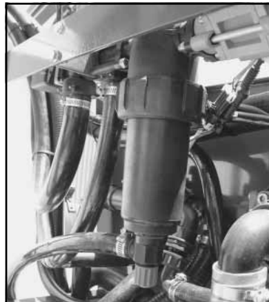
Pressure Filter (shown above on sprayer)
