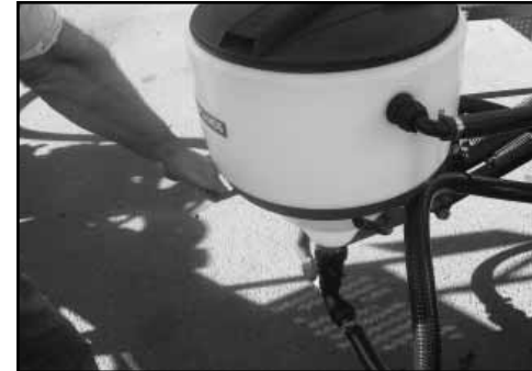
Lower hopper into the filling position.
