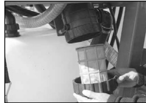
Remove and clean the suction filter
