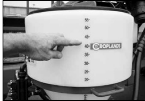
Watch the level closely - maximum fill is 50 litres.
