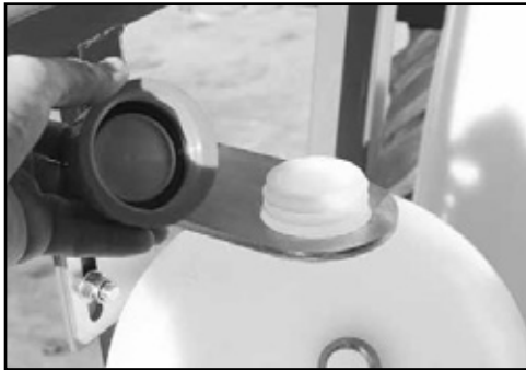
Open Fresh Water tank lid for filling.
