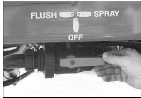
Place the suction valve in "Spray" position.
