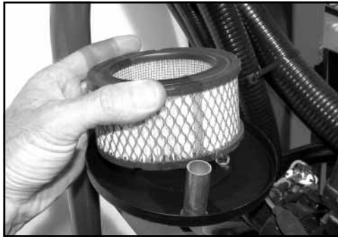
Regularly clean the air filter.
