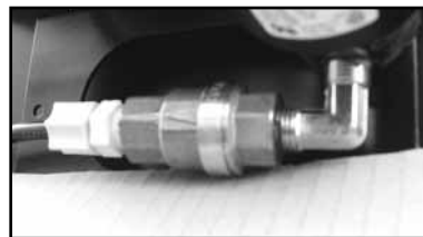
6 Check Valve P/N: RH69541
