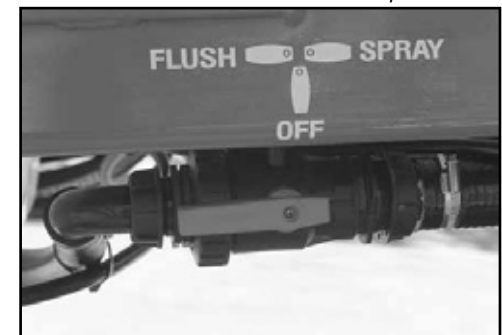
Turn the Suction Line Valve to "Flush" position.
