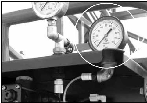
The foam marker pressure gauge.
