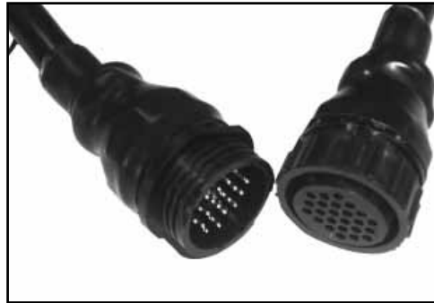
Connect electric/hydraulic console cables at rear of tractor.
