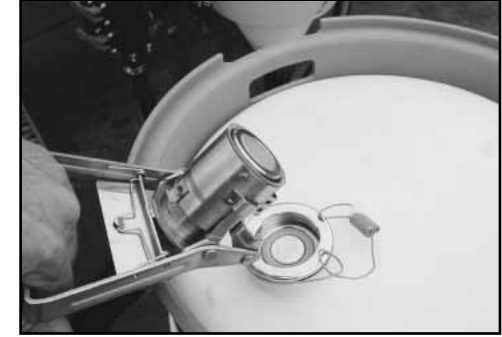
Unclip the Micromatic fitting from the Envirodrum.
