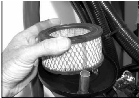
Make sure air filter is clean
