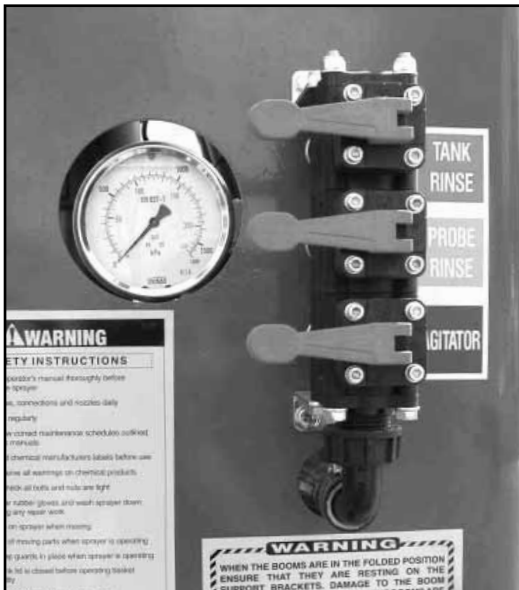
Shut-Off Taps - Tank Rinse, Probe Rinse & Agitators
