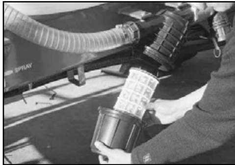
Clean bottom-fill filter regularly.
