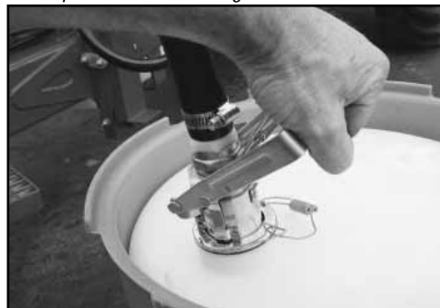
Clip the Micromatic fitting into the Envirodrum.
