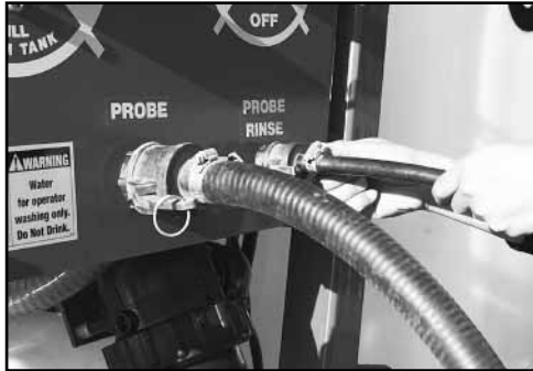
Connect Probe & Probe Rinse hoses.
