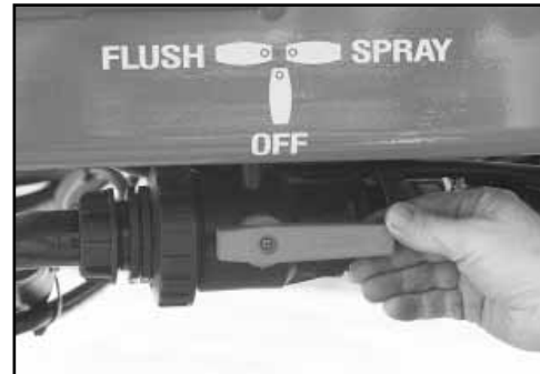
Place the suction valve in "Spray" position.
