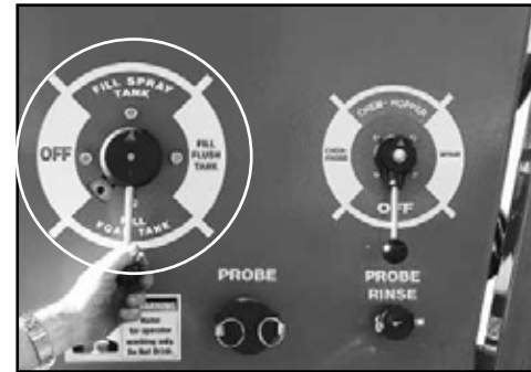
Rotate the Fill Control Lever to "Fill Spray Tank" position.
