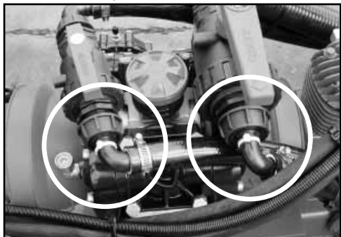
Note the two white cable tie which show the direction of the taps for the Enviro-transfer.
