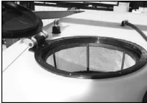
Open Spray tank lid for top-filling.
