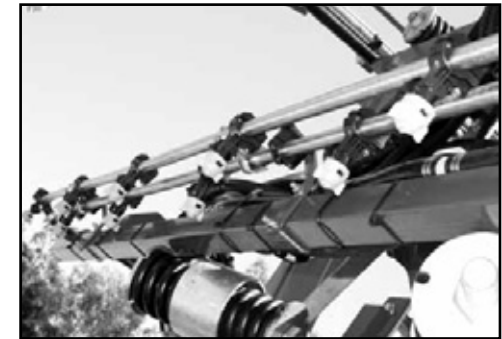
Dual lines on the boom.
