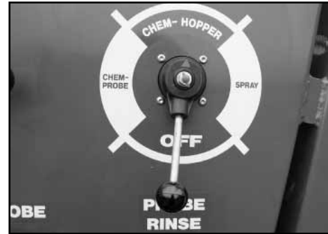
Turn the rotary selector to "Chem Hopper".
