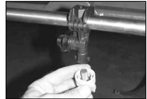
Regularly check and clean nozzle filters.
