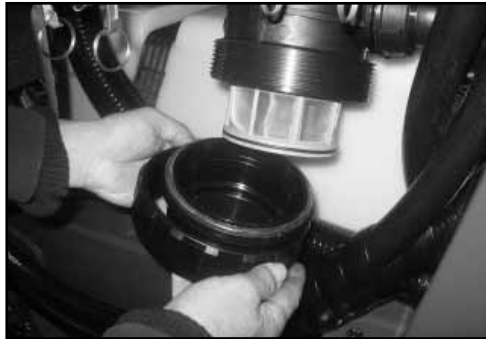
Remove outer screw & bowl of suction filter.
