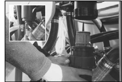
Clean pressure filter regularly (Inset shows valve).
