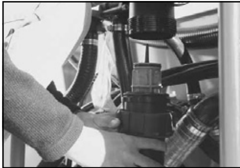
Check the pressure filter is clean.
