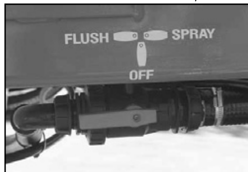
Turn the Suction Line Valve to "Flush" position.
