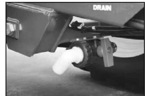
Close the Tank Drain valve.
