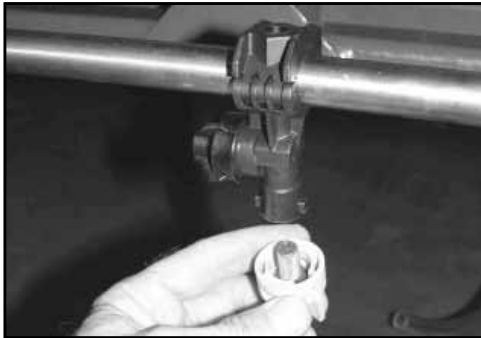
Clean nozzle filters regularly.
