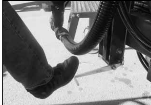
Unlock the Chem-E-Flush with the foot latch.
