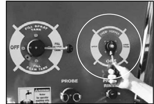
Rotate the Pressure Control lever to "CHEM-HOPPER".
