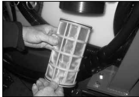
Remove & clean the filter element & components.
