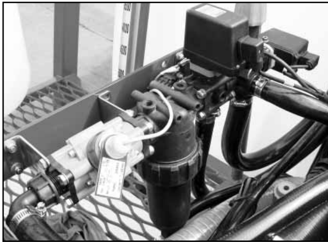
Liquid Control System - Complete Valve Assembly (Part No: A471CCRO01)
