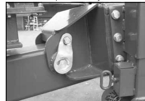
Ensure the pins are correctly reinstalled.
