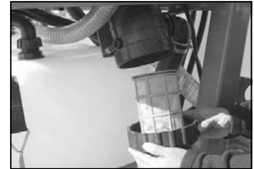
Check the suction filter is clean.
