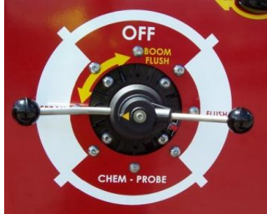
Pump suction valve (red arrow) to 'Flush' and Re-circ valve (yellow arrow) to 'Spray'
