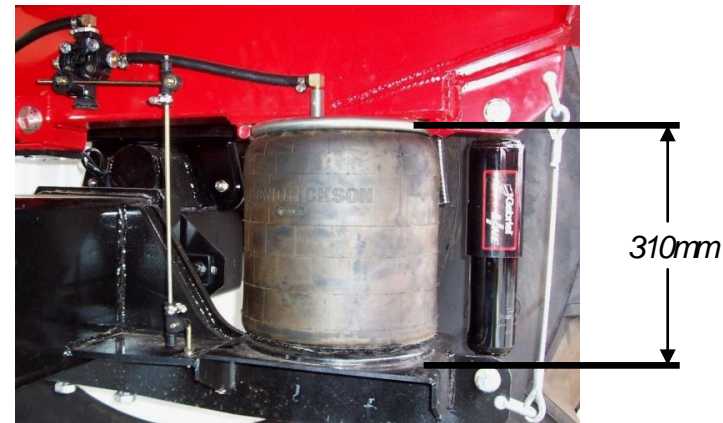
Adjust ride leveler valves as necessary to obtain correct Axle air bag ride height.
