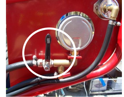
'SPRAY' gauge line flush tap
