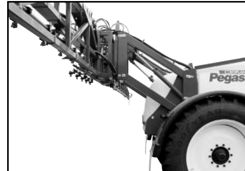
Boom in raised position.
