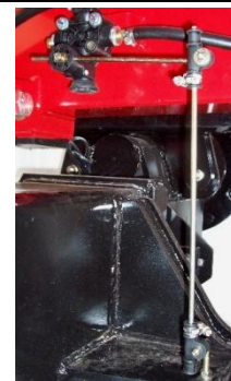
Axle air leveling Valve with adjustable linkage
