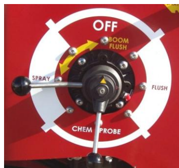
Suction valve to FLUSH, Re-circ to BOOM FLUSH
