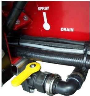
Open the tank drain valve to drain the main spray tank.
