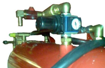
ARDS pressure control and drain valve
