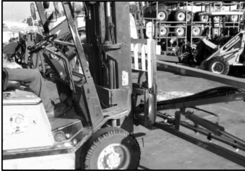
Take the pressure off the boom by nudging the boom forward.
