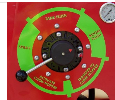
Operation Valve to BOOM FLUSH
