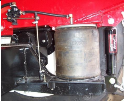
Axle Air-Ride Suspension System
