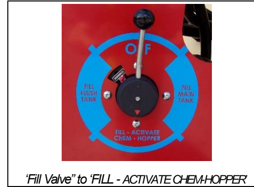
Adjust the 'Hopper Fill' valve as required
