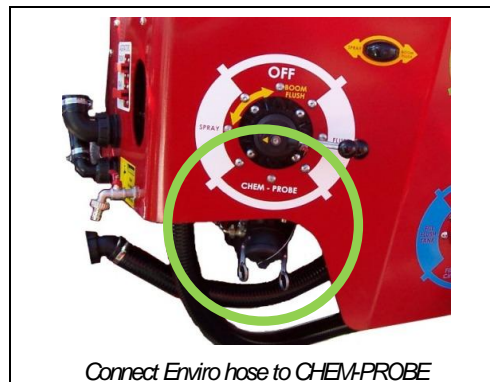
Connect Enviro hose to CHEM-PROBE
