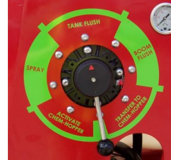
'Operation Valve' to 'Tank Flush' position
