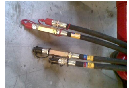
Disconnect hydraulic hoses
