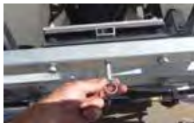
Fig 3: Shows the locking pin for use on sloping ground.
