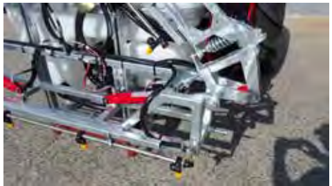
Fig 3: Hydraulic fold points are dangerous crush points. Keep hands clear at all times
