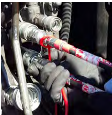
Fig 1: hydraulic hose connections to the tractor
