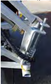
Fig 1: MAX boom breakaway - crush point.
