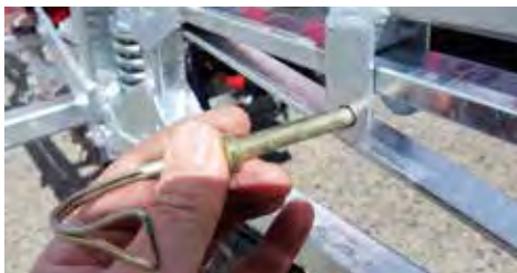
Outer wing pin in place to ensure outer arms are secure
