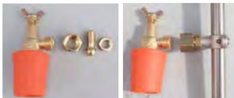
Nozzles assembled in this order and attached to boom tubes
