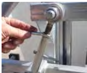
Fig 4: Undo the locking nut on the lower end of the strut.
