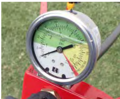
Pressure gauge for setting operating pressure during spraying
