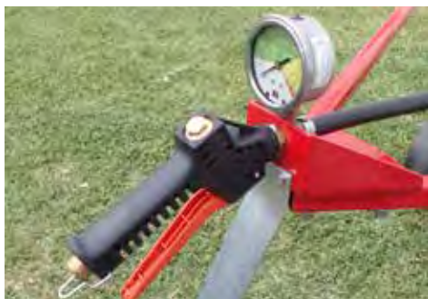
Connect your inlet spray hose to the fitting on the back of the trigger shut-off assembly
