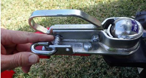
Figure 4b: Ensure pin can be secured
