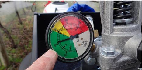
Figure 26: It is recommended not to exceed 30 bar spraying pressure
