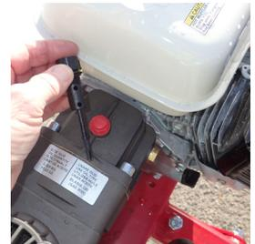
**Figure 12a: Install the dipstick in the AR303 or AR30 pump gearbox by removing the red plug**
