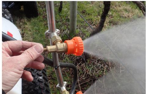
Spray pattern for vines should be adjusted for good spray coverage
