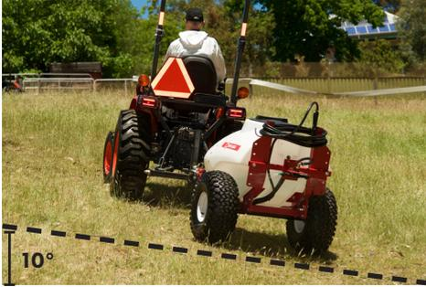
**Maximum recommended slope for safe operation is 10 degrees**
