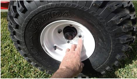
Figure 8: Check wheel nuts for tightness periodically
