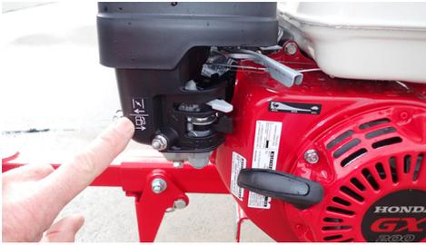
Figure 13: Choke & fuel on/off controls
