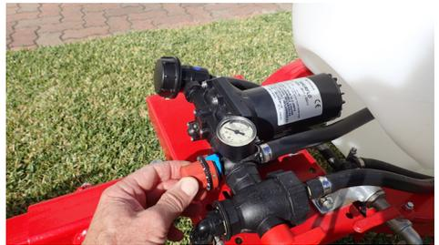
Figure 17: Adjust pressure
