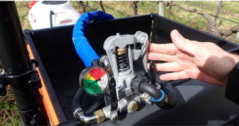
Figure 25: The remote PRV (Pressure control unit) should be fitted to the towing vehicle
