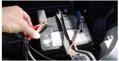
**Figure 6: Alligator clips - for connection to your 12-volt battery**
