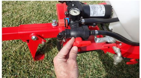
Figure 16: Ball valve in the hose reel position
