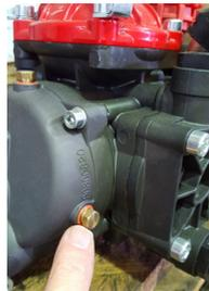
**Figure 12: Check gearbox oil level**
