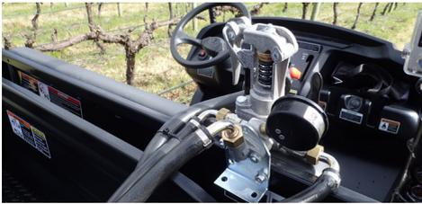
14a: Mount the remote ARG140 pressure regulator/control unit in a convenient location for the operator
