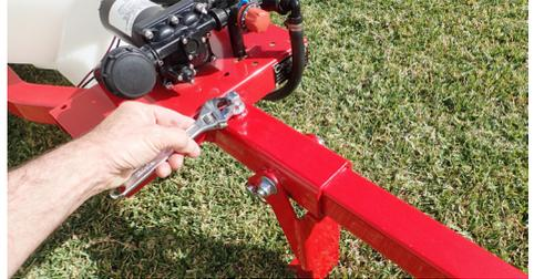
Figure 2: Undo locking bolt
