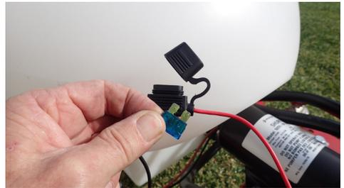
**Figure 7: Fuse - integrated into the loom**
