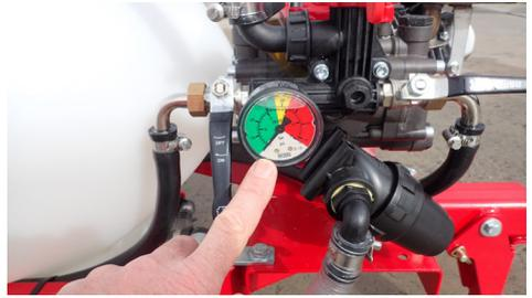
Figure 19: 10 bar maximum pressure for RL10 operation
