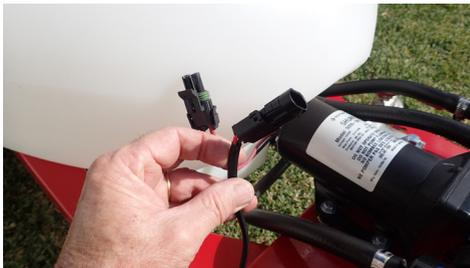
**Figure 5: Heavy duty loom and waterproof connections**
