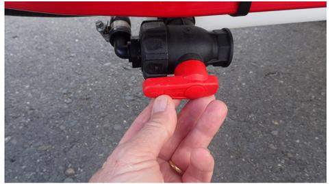
Figure 15: Ball valve in the suction position
