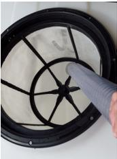
3. Put enough clean water into the spray tank to operate the pump and hand gun or boom (if fitted). The tank can be fully filled once your start up check is completed.
