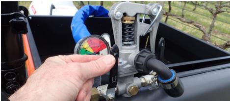
14b: Ensure the taps for left right control are accessible
