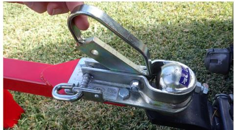
Figure 4a: Locking lever adjustment
