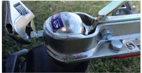
Figure 4: Adjust coupler for fit by adjusting bolt as pictured above. Tighten enough to ensure the coupler cannot jump off the towball when the lever is secure.
