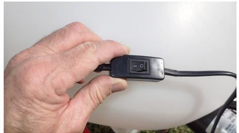
**Figure 7a: Rocker switch - for starting & stopping the pump on 12-volt models**
