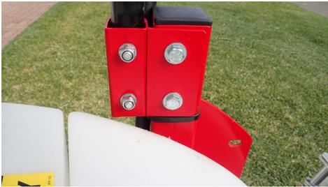
Figure 9: Check bolts & nuts
