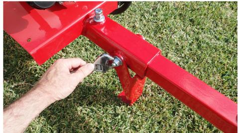
Figure 3: Undo stand and adjust length. Reverse steps 2 and 3 once length is decided.
