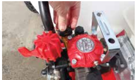
Figure 11: Check pump oil level.
