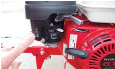
Figure 13: Choke & fuel on/off controls.
