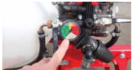
Figure 19: 10 bar maximum pressure for RL10 operation.
