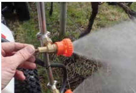
Spray pattern for vines should be adjusted for good spray coverage
