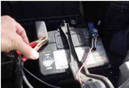
Figure 6: Alligator clips - for connection to your 12-volt battery
