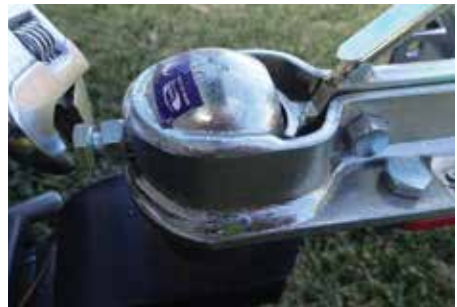
Figure 4: Adjust coupler for fit by adjusting bolt as pictured above. Tighten enough to ensure the coupler cannot jump off the towball when the lever is secure.
