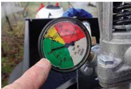
Figure 26: It is recommended not to exceed 30 bar spraying pressure.
