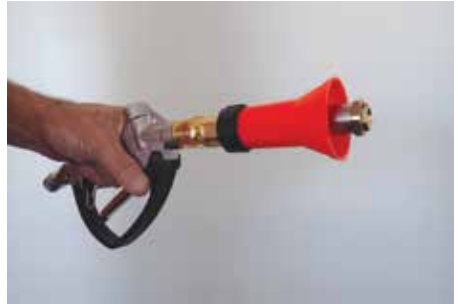
Figure 23: Pull back the orange cone cover for normal spraying
