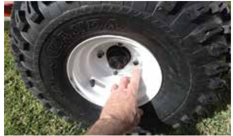
Figure 8: Check wheel nuts for tightness periodically
