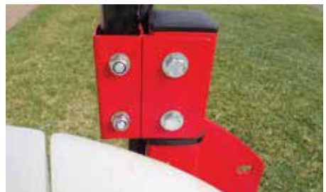
Figure 9: Check bolts & nuts
