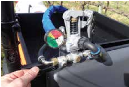
Figure 25a: Turn the left & right taps on individually to test spray pattern.
