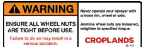
Figure 8: Check wheel nuts for tightness periodically
