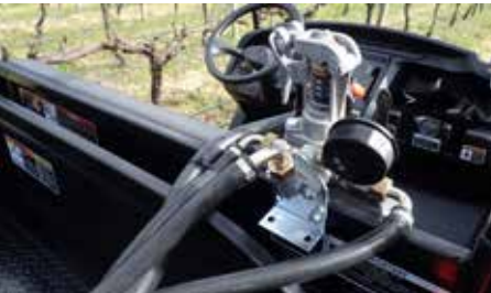
14a: Mount the remote ARG140 pressure regulator/control unit in a convenient location for the operator.
