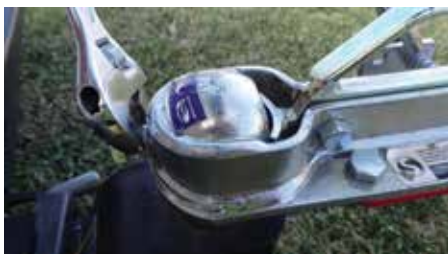
Figure 4c: Ensure lock nut is tightened once adjustment is complete.
