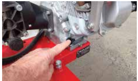
Figure 10: Oil level check.
