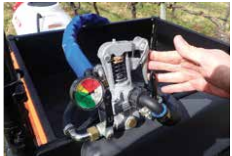
Figure 25: The remote PRV (Pressure control unit) should be fitted to the towing vehicle.
