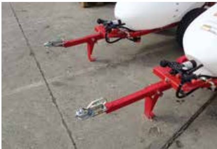
Figure 1: Drawbar position short and long
