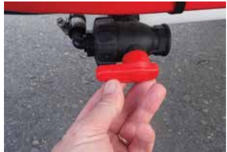
Figure 15: Ball valve in the suction position
