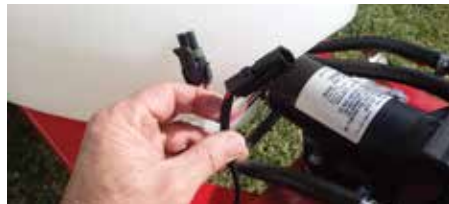
Figure 5: Heavy duty loom and waterproof connections
