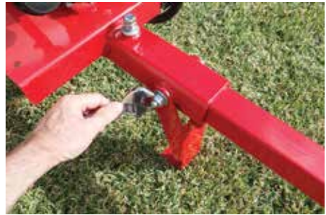
Figure 3: Undo stand and adjust length. Reverse steps 2 and 3 once length is decided.
