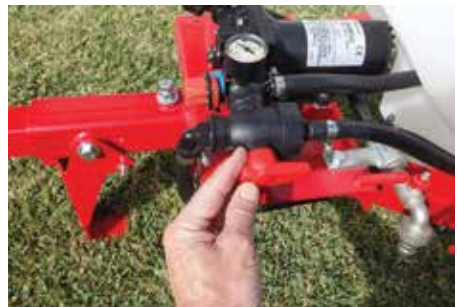
Figure 16: Ball valve in the hose reel position
