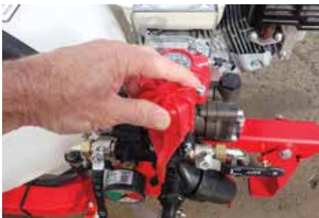
Figure 21: Adjust pressure as required.
