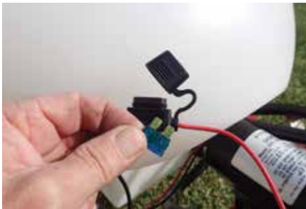
Figure 7: Fuse - integrated into the loom
