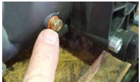
Figure 12: Check gearbox oil level.
