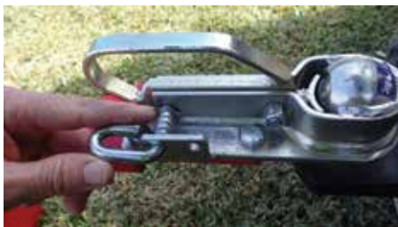
Figure 4b: Ensure pin can be secured.
