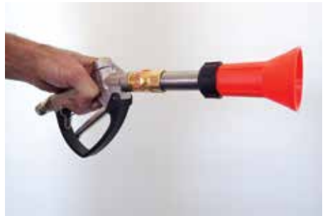
Figure 24: For creating a "fog" spray, pull the orange cone cover forward.
