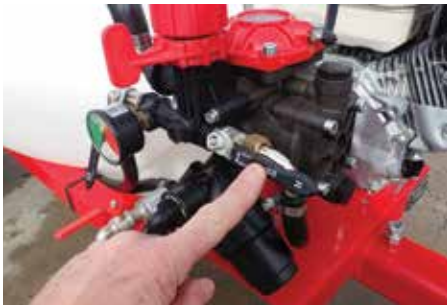
Figure 20: Turn valve on to reel.
