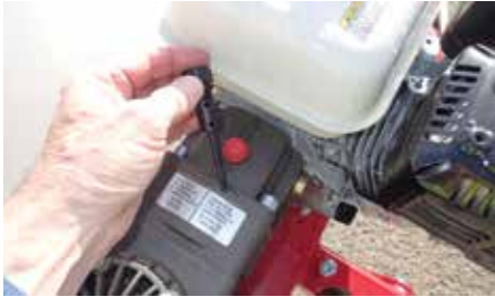
Figure 12a: Install the dipstick in the AR303 or AR30 pump gearbox by removing the red plug.
