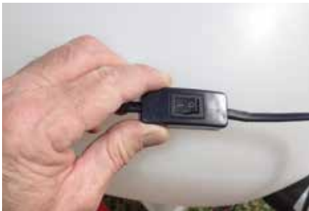
Figure 7a: Rocker switch - for starting & stopping the pump on 12-volt models
