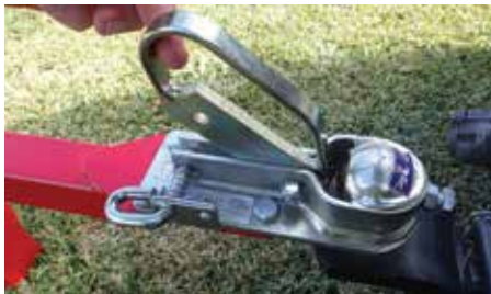
Figure 4a: Locking lever adjustment.
