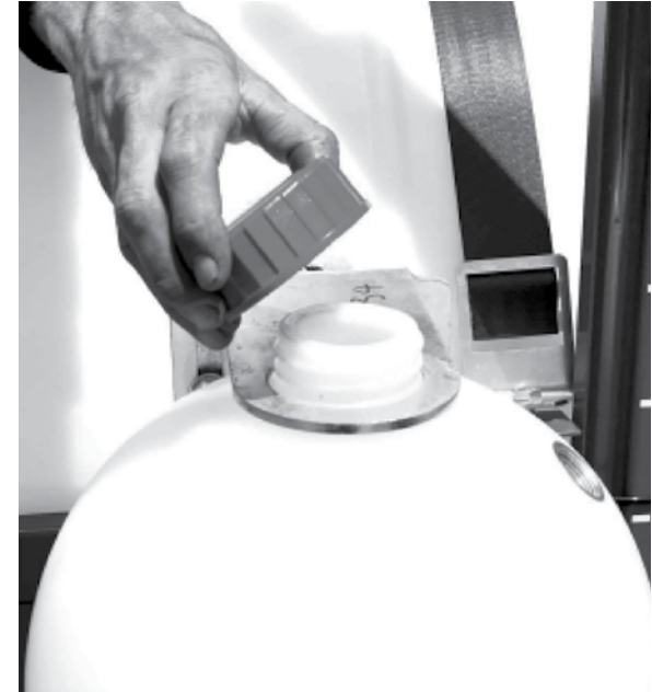
Open foam marker lid for filling
