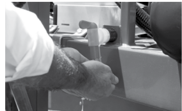
Fresh water tank for personal safety
