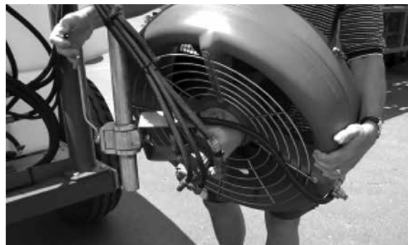
Spin mount to move fan closer to canopy, and to allow tilt adjustment
