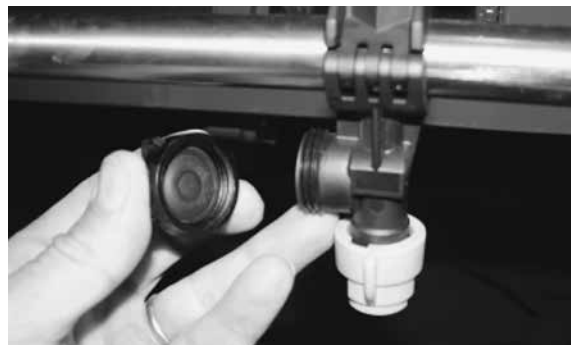
Remove & clean non-drip diaphragms regularly
