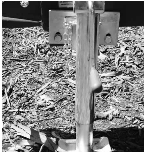
Grease the jack (if fitted)
