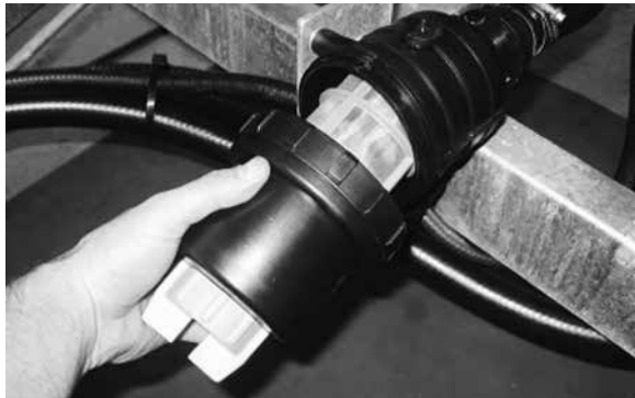
Check suction filter is clean
