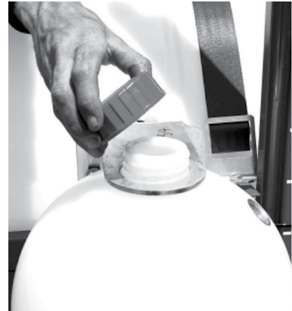
Open foam marker lid for filling
