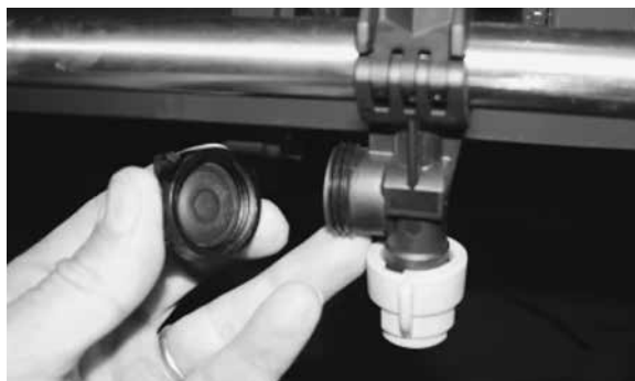
Remove & clean non-drip diaphragms regularly
