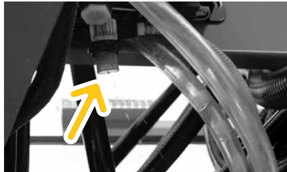
Remove foam marker filter bowl & 50 mesh screen
