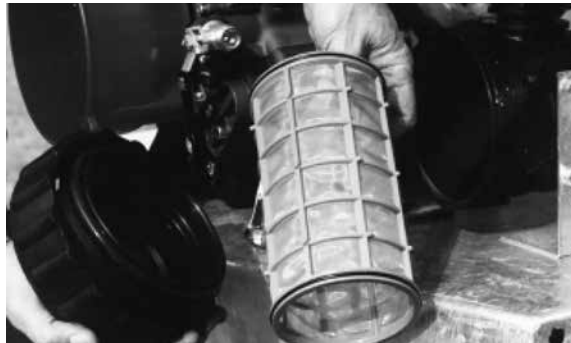
Remove & clean the filter element & components
