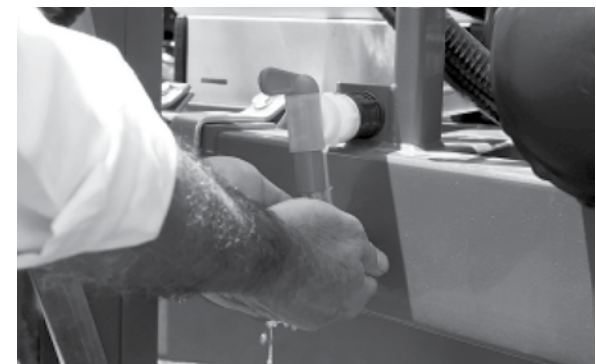
Fresh water tank for personal safety
