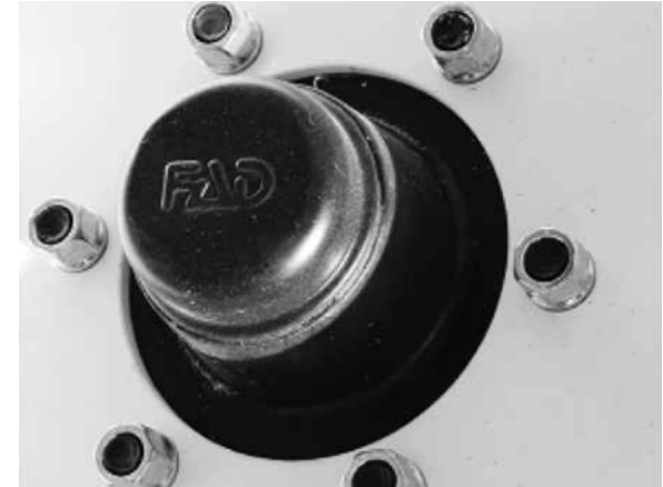
Repack the wheel bearings at 200 hours
