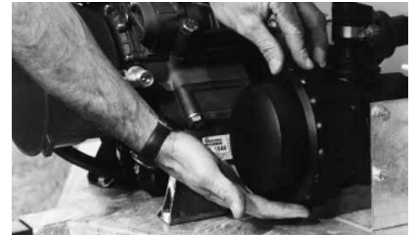
Reassemble & tighten outer screw of suction filter..
