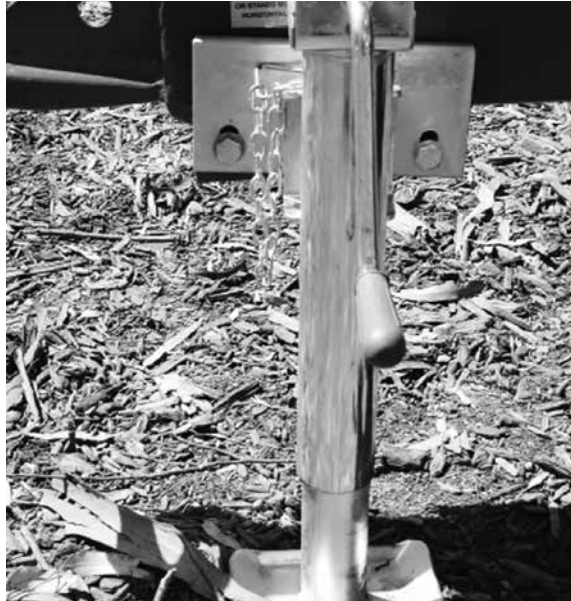
Grease the jack (if fitted)
