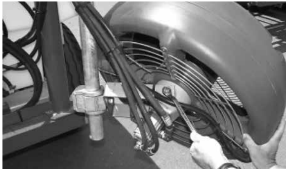
Adjust mount for forward/rearward fan adjustment
