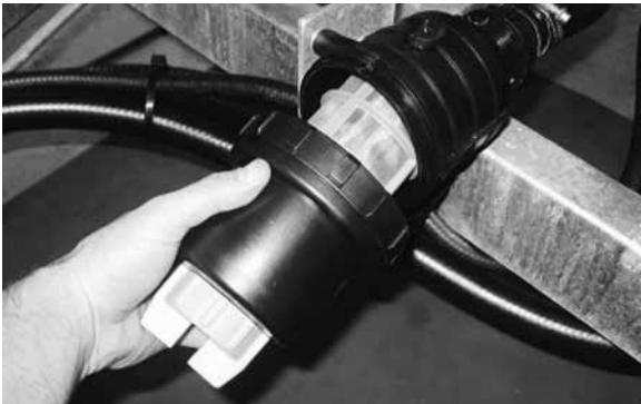
Check suction filter is clean
