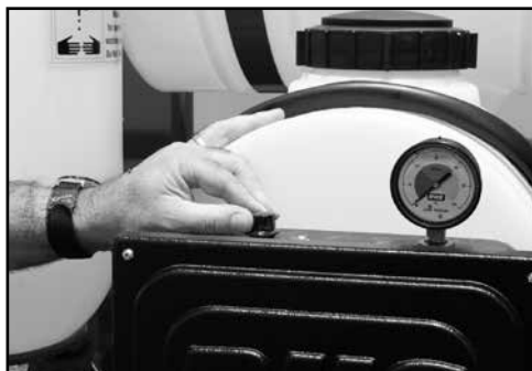
Foam marker adjustment knob & pressure gauge.
