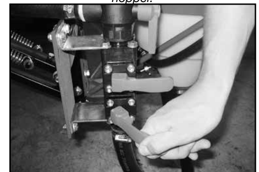
(n) Open the drum rinse valve to rinse the hopper.
