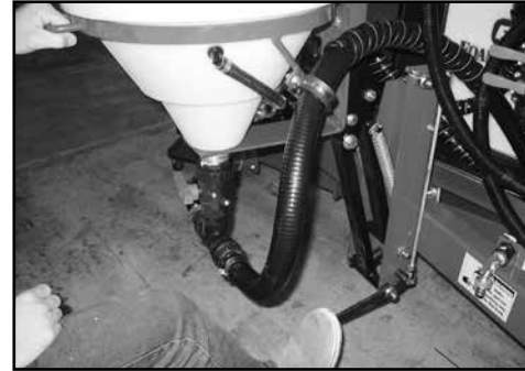
(b) Unlock the latch with the foot lever.
