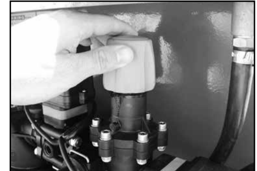
Adjust the manual pressure relief valve.
