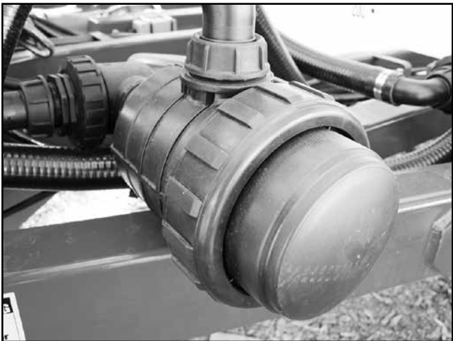
Suction Filter (shown above on sprayer) Pressure Filter (shown below on sprayer)
