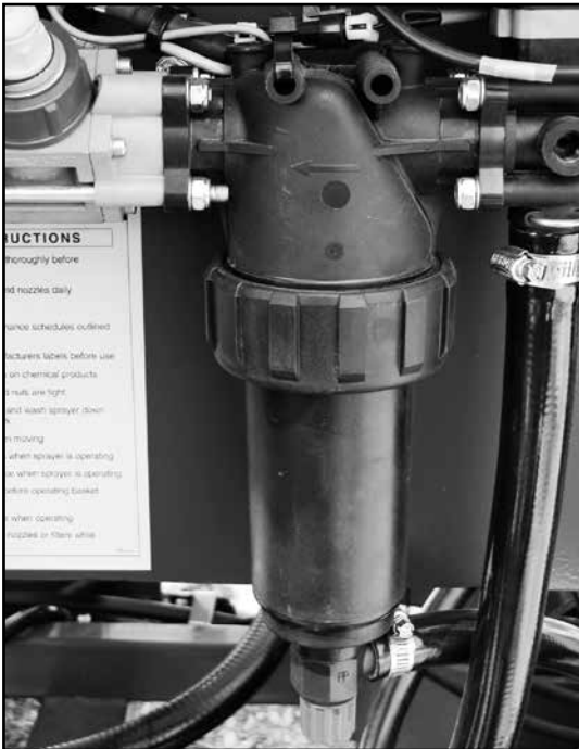
Suction Filter (shown above on sprayer) Pressure Filter (shown below on sprayer)
