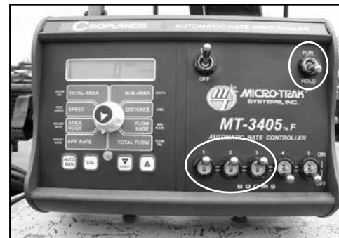
Boom switches On, Master switch On Hold.
