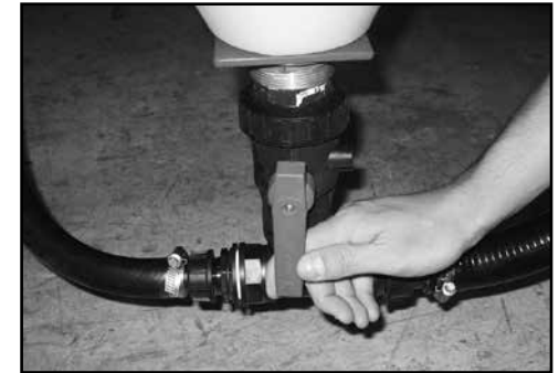
(m & o) Open transfer valve to transfer mixture to the spray tank.
