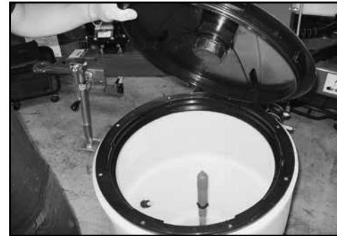
(j) Open hopper lid & add chemical powder or liquid.
