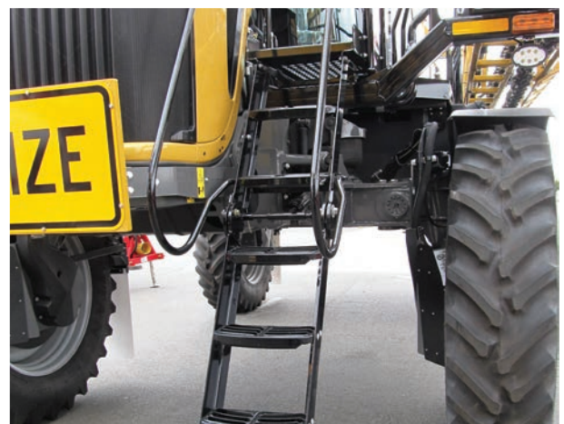
Steps provided to access the cab and platform on a self-propelled sprayer. Use both hand rails and avoid carrying items while ascending and descending.
