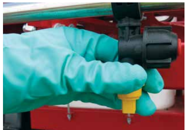
Ensure boom lines have no residual pressure before removing flushing caps or nozzles. Wear chemical resistant gloves.
