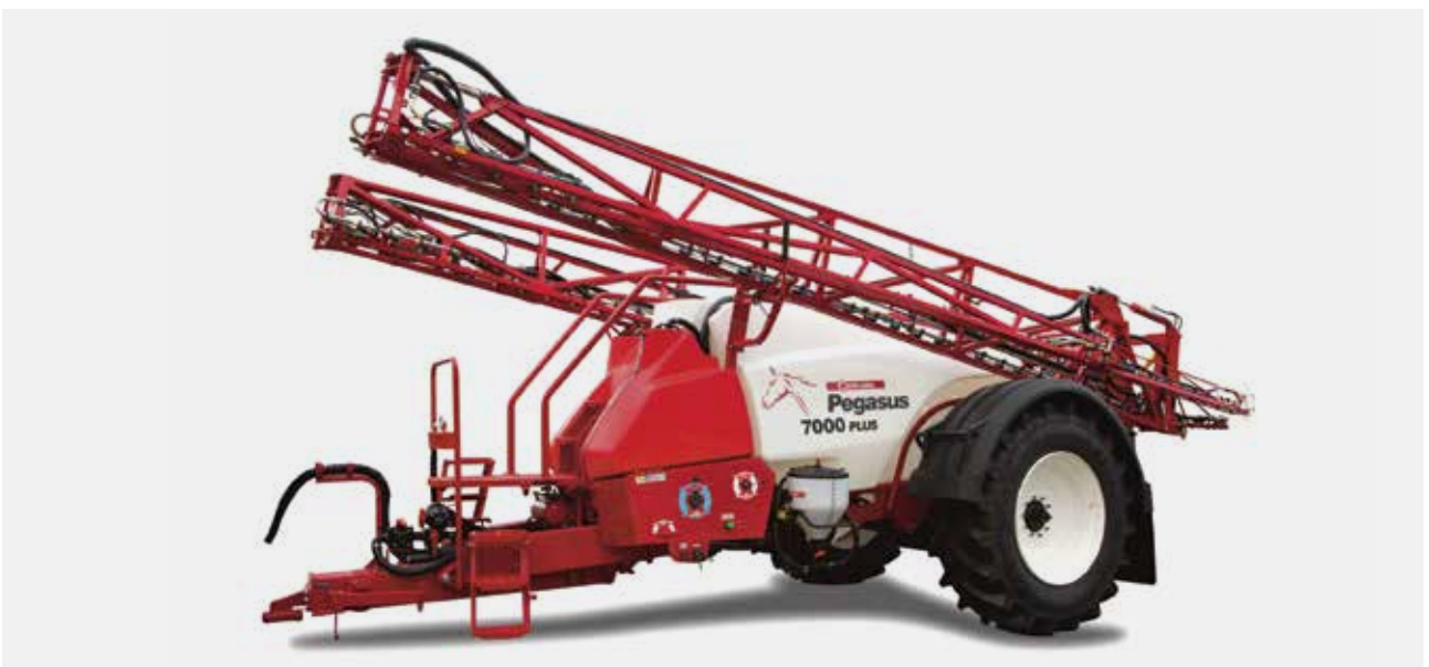
Steps provided to access a working platform on a trailed sprayer. These steps fold manually - Ensure steps are in the upright position before moving the sprayer.
