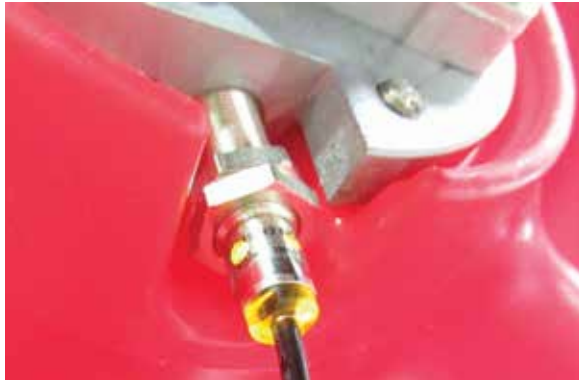
1. Hand fit to correct depth.
