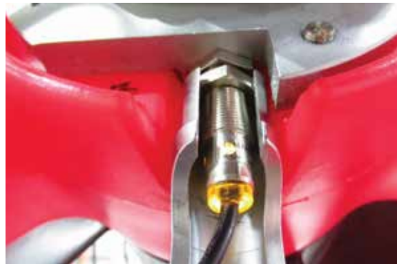
4. Tighten 2nd (locking) nut.
