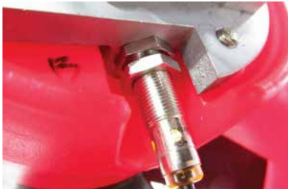
2. Screw first nut into place
