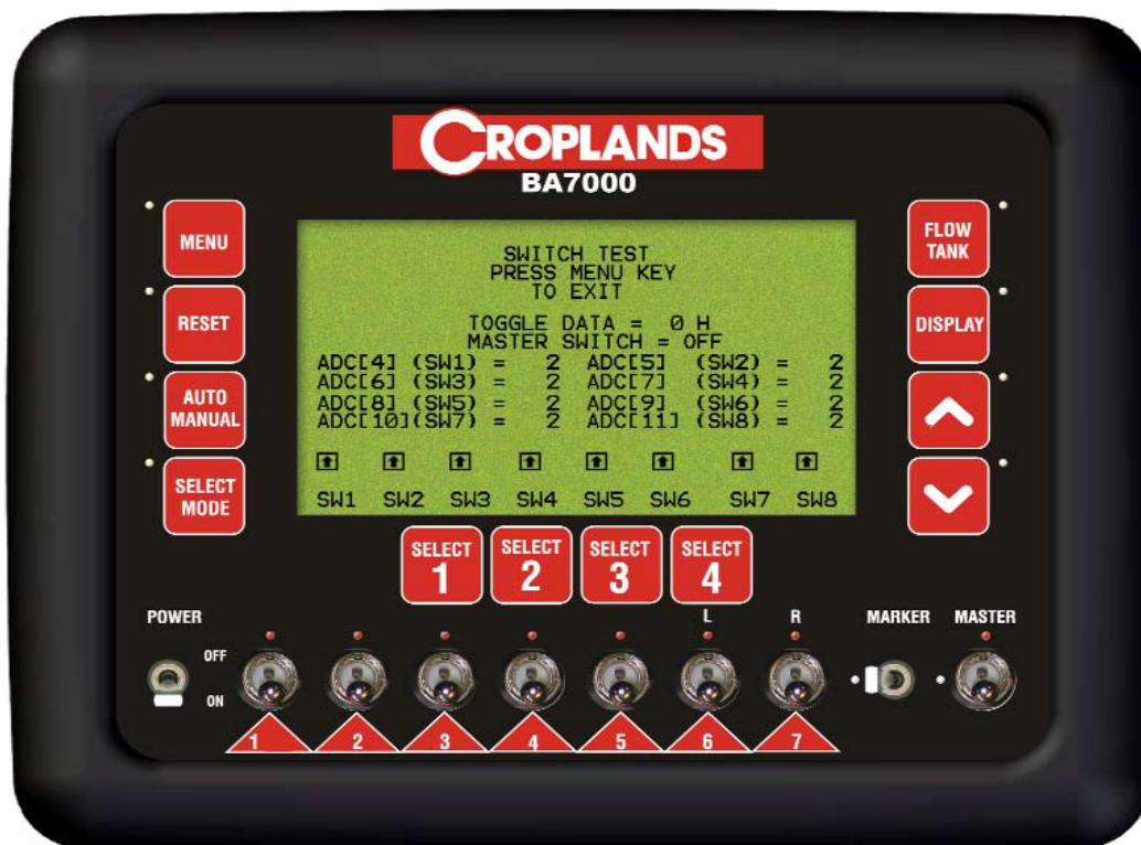
Switch Diagnostics Screen
