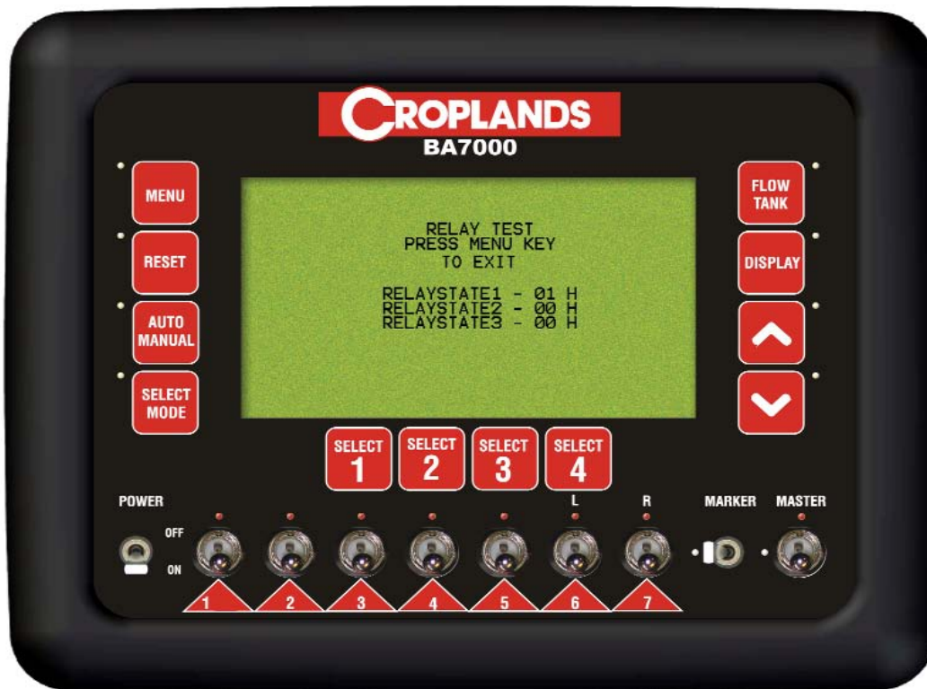
Relays Diagnostics Screen
