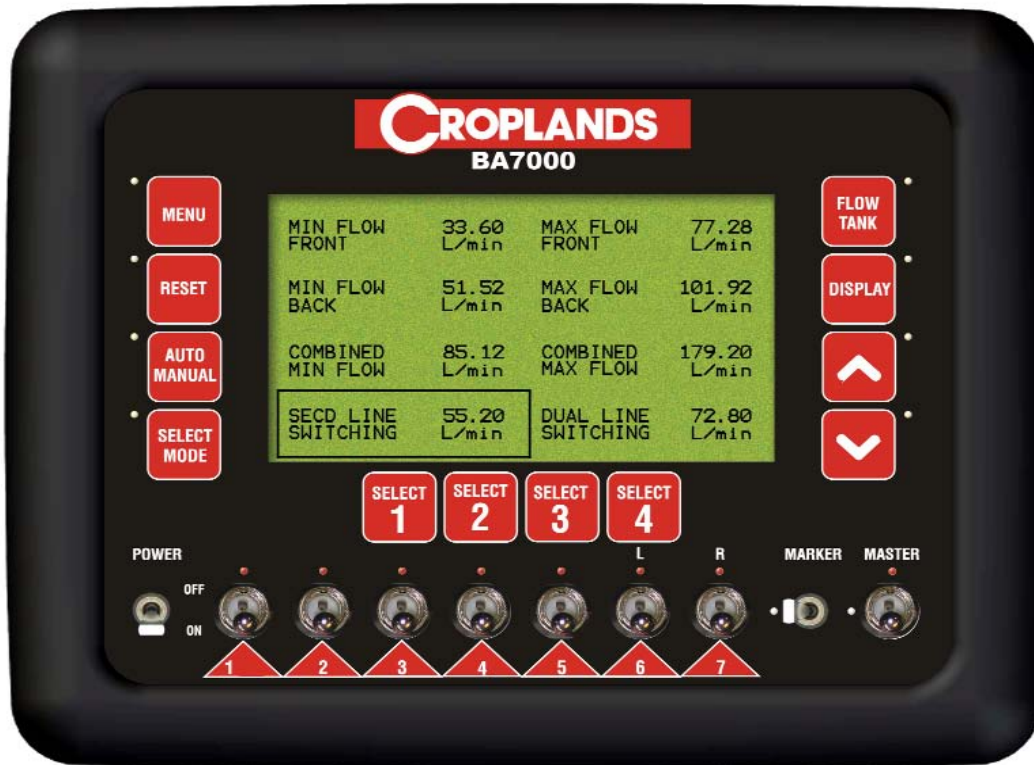
Dual Line Switching(Flow) Screen
