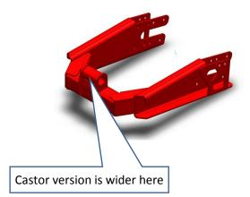
Retrofitting new v3 swing arm to original pivot / body. The extra width of the v3 swing arm means that the shock absorber mounts are 60mm wider than the original pivot/body shock absorbers mounting position. Rework the shock absorber mounts by using the "retrofit shock mount", MP-394 (supplied as a pair, LH & RH).
