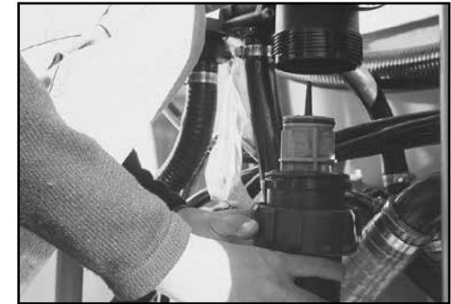
Remove and clean the pressure filter
