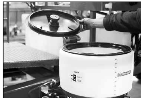
Open hopper lid & add chemical powder/liquid.
