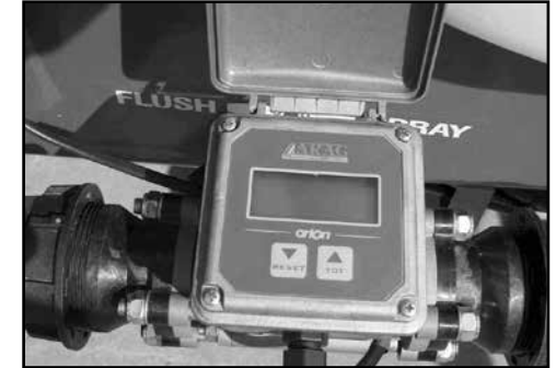
Orion filling flow-meter.
