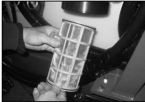
Remove & clean the filter element & components.
