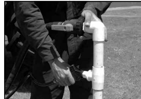
Use the Probe Rinse gun to rinse the container.
