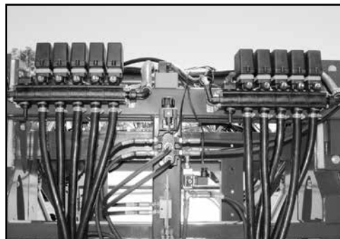
Dual line valves at the rear of the sprayer.
