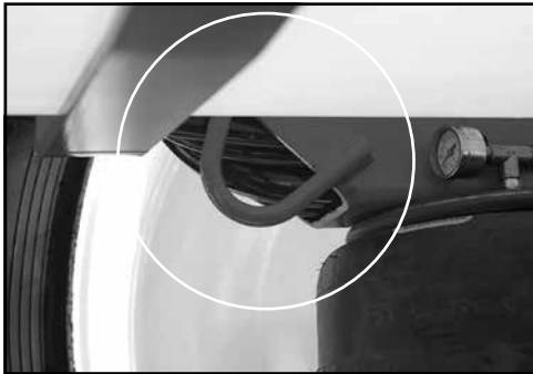
Use the tie-down points provided when transporting.
