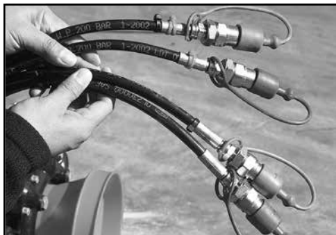
Disconnect hydraulic hoses & PTO shaft.
