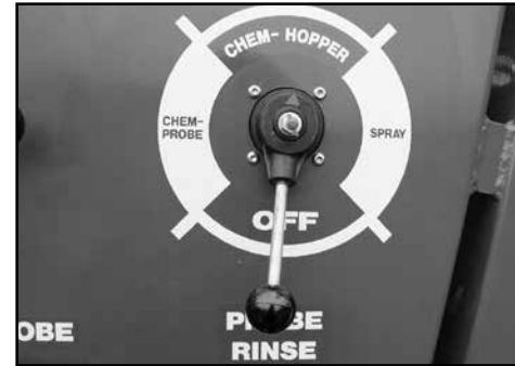
Turn the rotary selector to "Chem Hopper".
