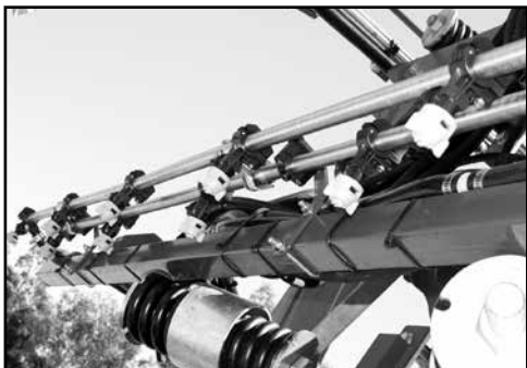
Dual lines on the boom.
