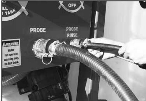
Connect Probe & Probe Rinse hoses.
