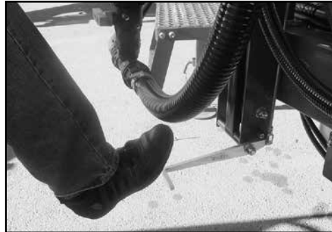
Unlock the Chem-E-Flush with the foot latch.
