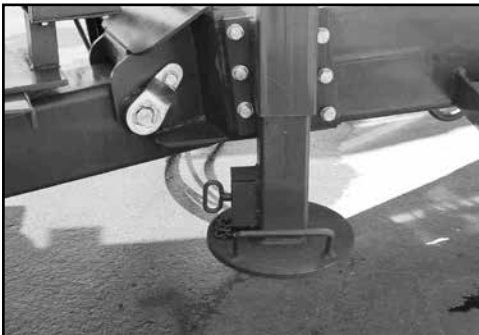
Pin the lift jack into position.
