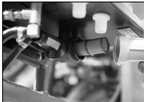
After cleaning, replace the screen & filter bowl.
