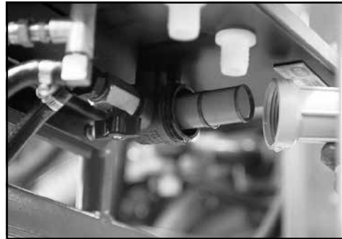
Regularly clean the foam marker filter.
