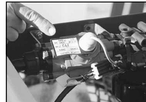
Enter the flow meter calibration factor.
