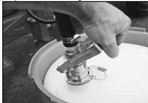
Clip the Micromatic fitting into the Envirodrum.
