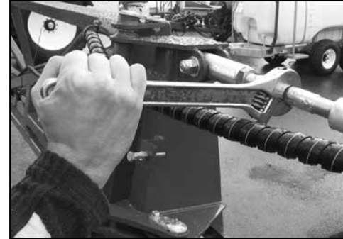
Adjust the sleeve until the boom is at the desired level, then re-lock the lock nut to secure in place.
