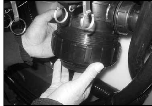
Reassemble & tighten outer screw of suction filter.
