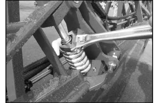
Finally, adjust the breakaway arm to the desired breakaway pressure.
