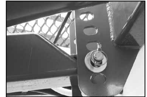
Remove the pin adjust the hitch height as required.
