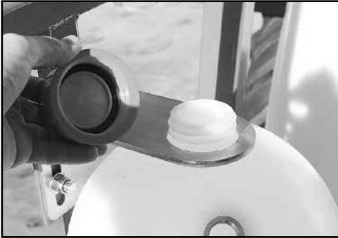
Open Fresh Water tank lid for filling.
