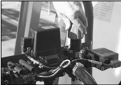
Adjust the manual pressure relief valve.
