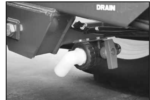
Close the Tank Drain valve.
