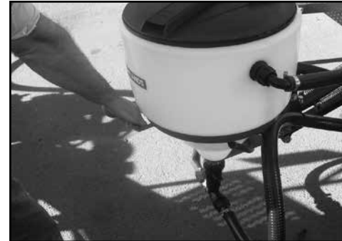
Lower hopper into the filling position.
