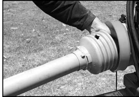
Correctly fit the PTO shaft to the Pegasus.
