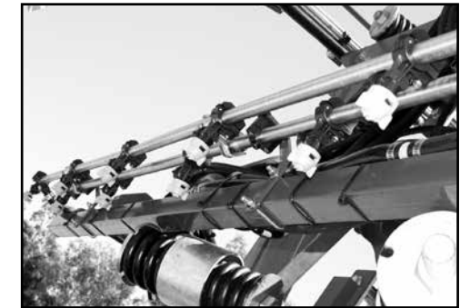
Dual lines on the boom.
