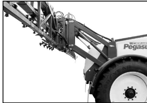
Unique parallelogram boom lift - high position.
