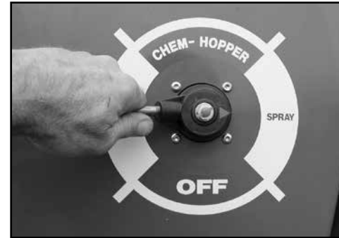
Return the main rotary selector to the "Spray" position.
