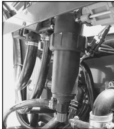
Pressure Filter (shown above on sprayer)
