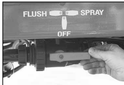
Place the suction valve in "Spray" position.
