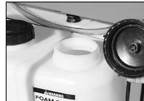
Open Foam tank lid for top-filling/adding concentrate.
