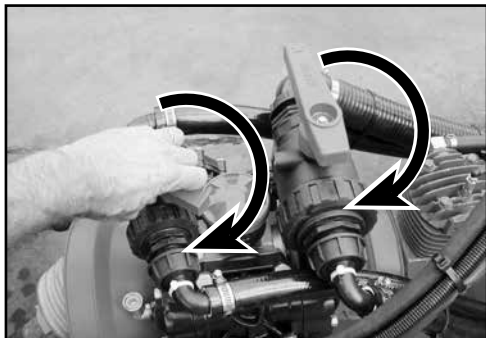
With the pump running, turn the two taps into the Enviro-transfer position.
