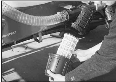
Clean bottom-fill filter regularly.
