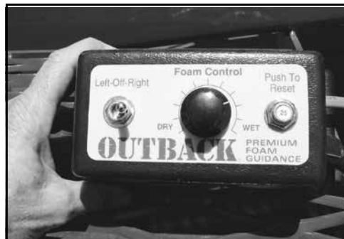
Mount the Foam Marker Controller in the cab.
