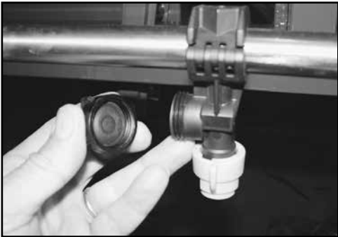
Remove & clean non-drip diaphragms regularly.
