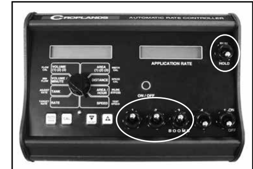
Boom switches on, master switch in hold.
