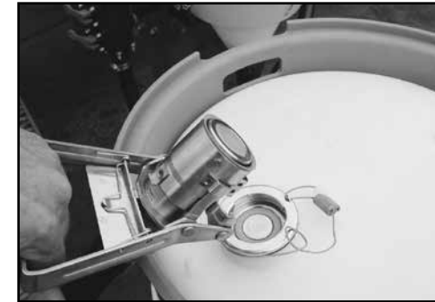
Unclip the Micromatic fitting from the Envirodrum.
