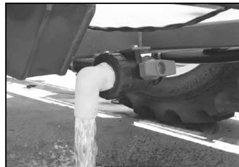
Open the Tank Drain valve to drain the tank.
