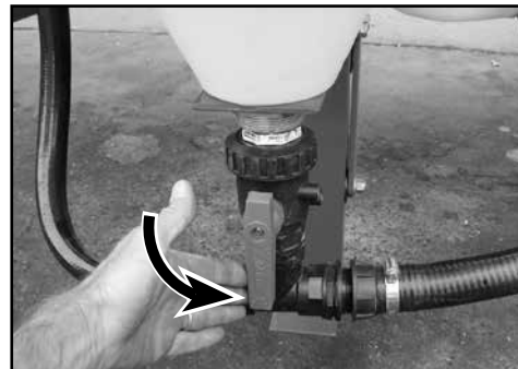
Turn the Chem-e-flush tap to introduce the chemical directly to tank (as shown).
