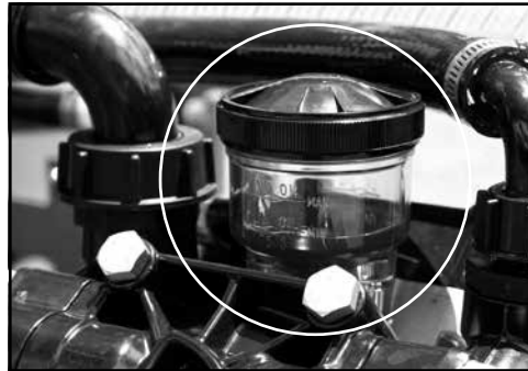
Check pump oil level.
