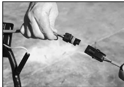
Connect the 4-pin plugs of the Foam Marker Controller.
