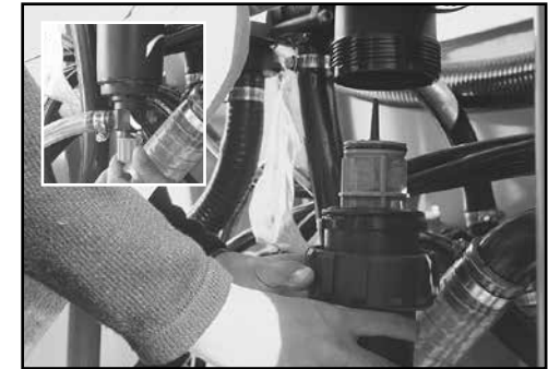
Clean pressure filter regularly (Inset shows valve).
