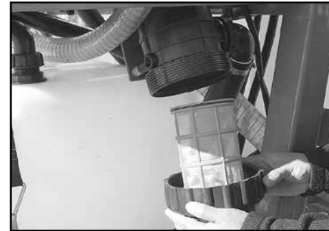
Remove and clean the suction filter
