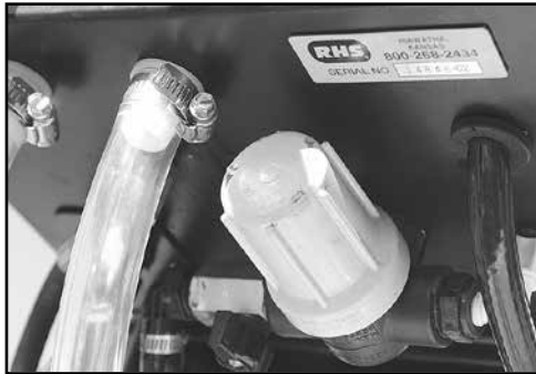
Make sure the foam marker liquid filter is clean.
