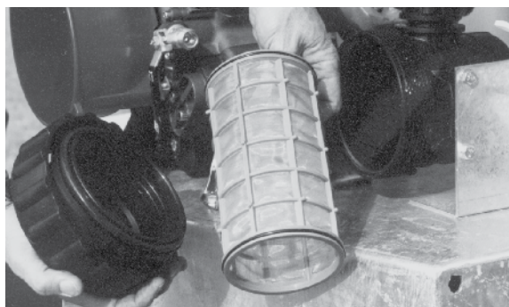
Remove & clean the filter element & components
