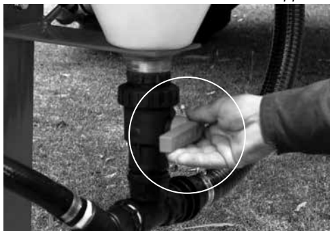
Close transfer valve at the base of the hopper.
