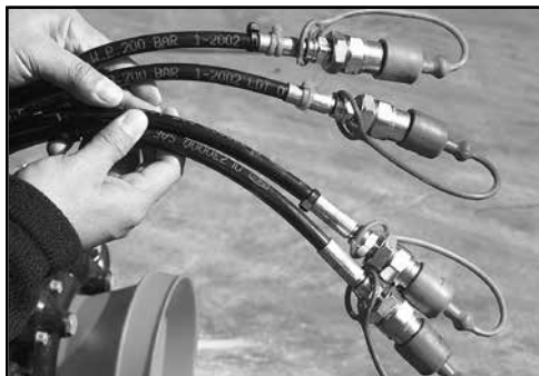
Disconnect hydraulic hoses & PTO shaft.
