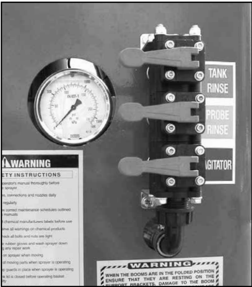
Shut-Off Taps - Tank Rinse, Probe Rinse & Agitators
