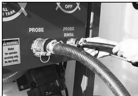
Connect Probe & Probe Rinse hoses.
