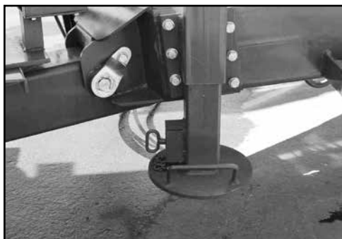
Pin the lift jack into position.
