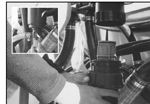
Clean pressure filter regularly (Inset shows valve).
