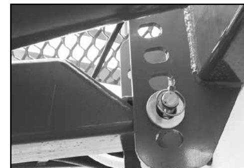
Remove the pin adjust the hitch height as required.
