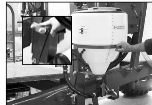
Lift the hopper & lock it back into transport position.
