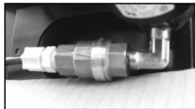
6 Check Valve P/N: RH69541
