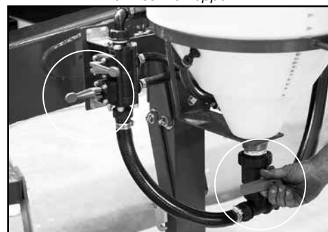
Close transfer valve & open the Drum Rinse valve to rinse the hopper.
