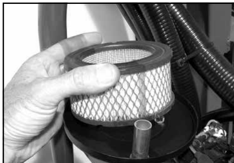
Make sure air filter is clean
