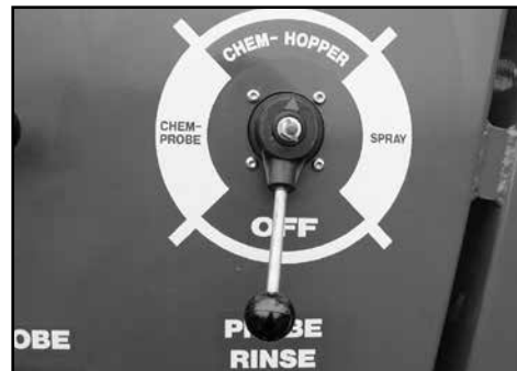
Turn the rotary selector to "Chem Hopper".
