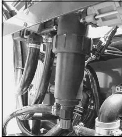
Pressure Filter (shown above on sprayer)
