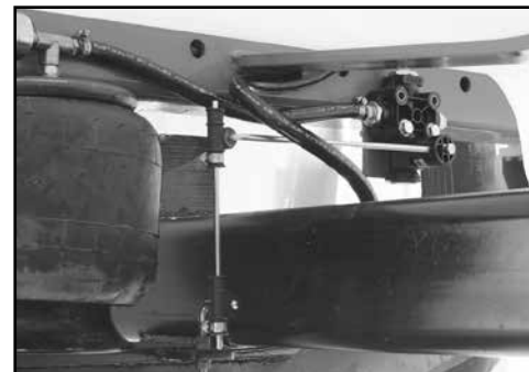
Air levelling valve with adjustable linkage.
