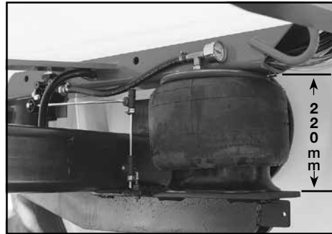
Unladen airbag ride height is pre-set to 220mm.
