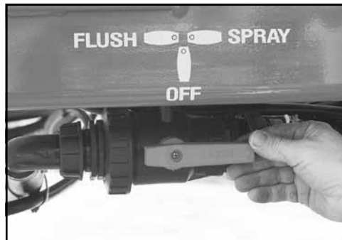
Place the suction valve in "Spray" position.
