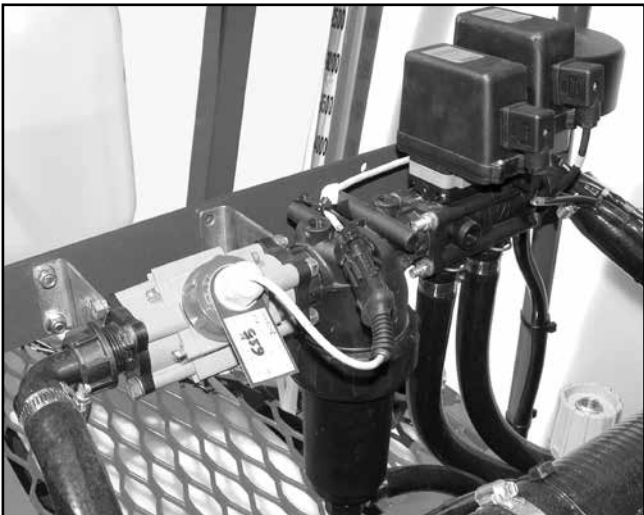
Liquid Control System - Complete Valve Assembly (Part No: A473CCRO01)
