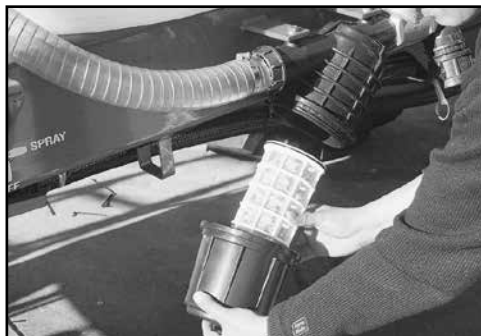
Clean bottom-fill filter regularly.
