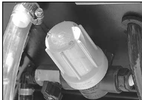
Close the filter tap & then remove the filter bowl.
