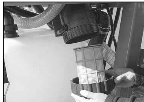
Remove and clean the suction filter
