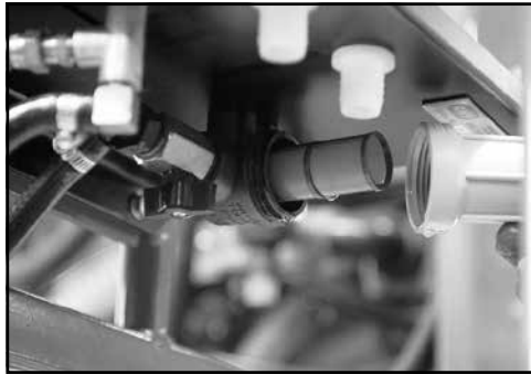
Regularly clean the foam marker filter.
