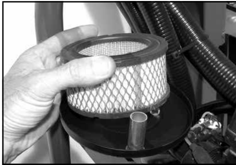
Regularly clean the air filter.
