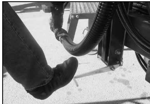
Unlock the Chem-E-Flush with the foot latch.
