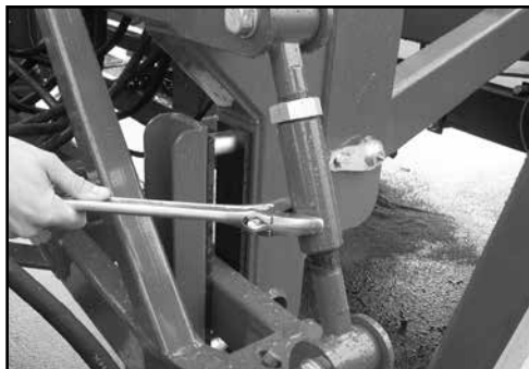
Adjust the turnbuckle sleeve until the centre section is level.
