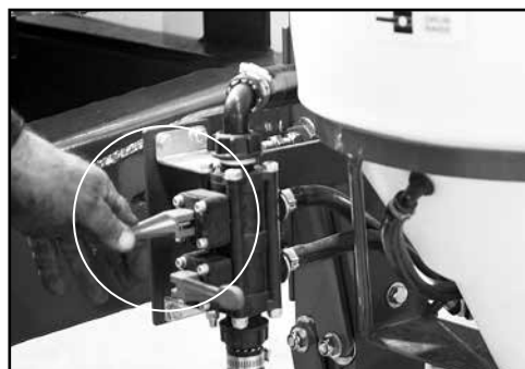
Close hopper lid & open the Chem-E-Flush Nozzle valve to mix chemical.
