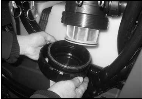
Remove outer screw & bowl of suction filter.
