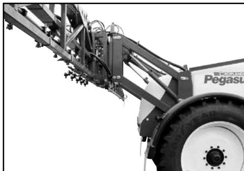
Unique parallelogram boom lift - high position.
