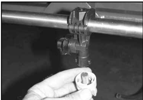
Clean nozzle filters regularly.
