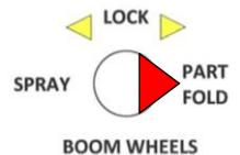
4. Drive forwards slowly below 5 KM/H. While moving forward, hold both the **LH WHEEL** & **RH WHEEL** switches **DOWN**, this will allow the booms to move approximately out half way
