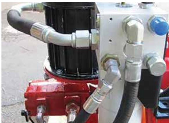
Version 1 "pot" with dual pump, "classic" version manifold and filter
