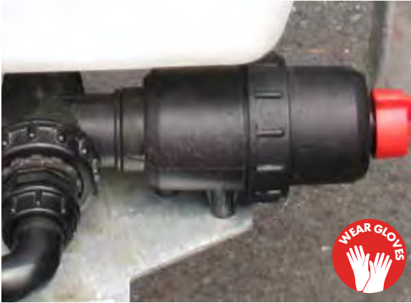
Reassemble and tighten the outer filter screw.
