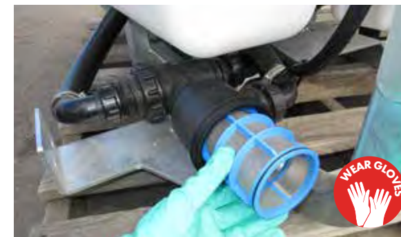
Remove & clean the filter element & components
