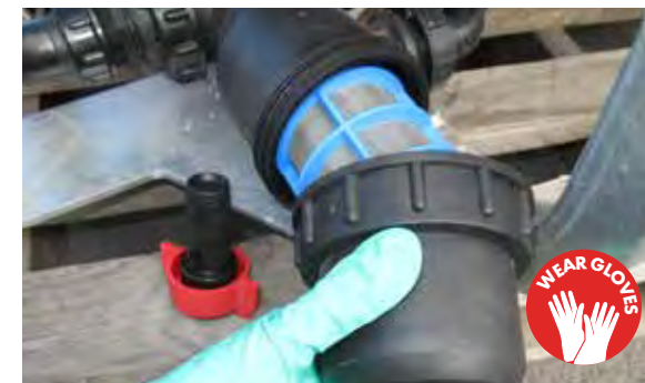
Remove the outer filter screw and bowl
