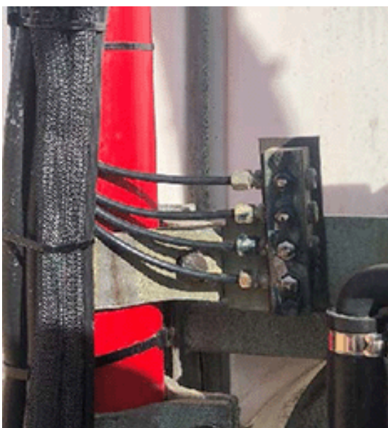
Common easy-reach grease point, one per side – fitted by the grower
