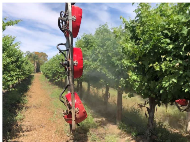
Final head set up – similar to factory default but top head dropped slightly. Note this is a longer frame than standard
