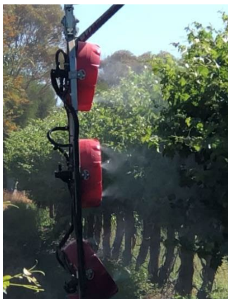
Evidence of some stripping between sectors 1 and 2 using 40-deg nozzle
