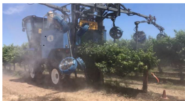
We thought head angles could have been adjusted to improve coverage – closer and flatter to canopy: time did not allow us to have a play.
