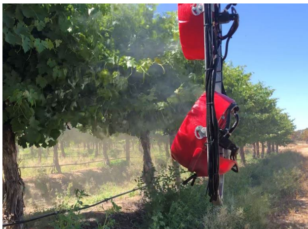
Bottom head adjusted slightly steeper – still some spray “lost” under the canopy. We will try 60-deg nozzles in next test
