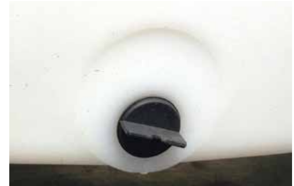
Adjust the variable cone nozzle for the required spray pattern
