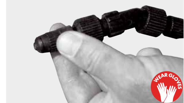
Adjust the variable cone nozzle for the required spray pattern
