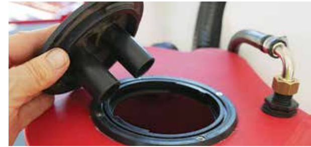
Open the Flush tank lids for inspection
