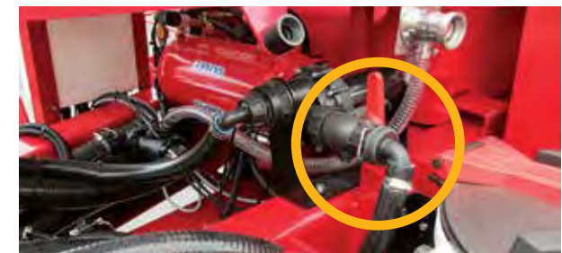
Close the Ag Runner tap to the hopper
