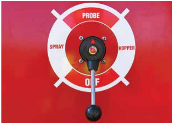
Rotate the Pressure valve to the "Probe" position
