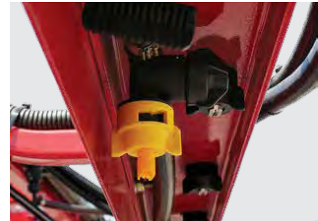
Clean nozzle filters regularly
