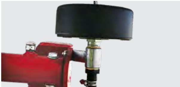
Clean the compressor air filter regularly
