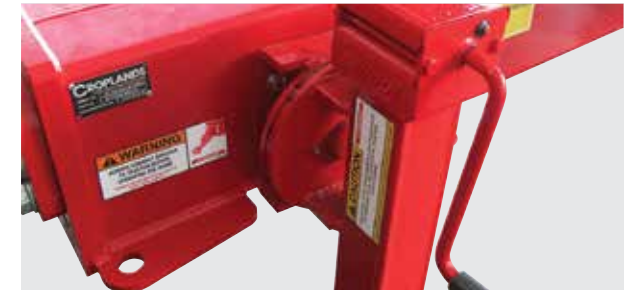
Lock the hitch jack in position, then adjust the hitch height
