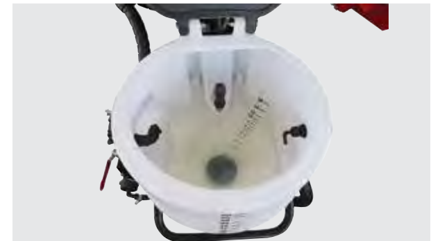
Open hopper lid & add chemical powder/liquid
