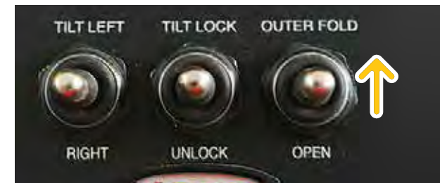
Push and hold to Outer Fold
