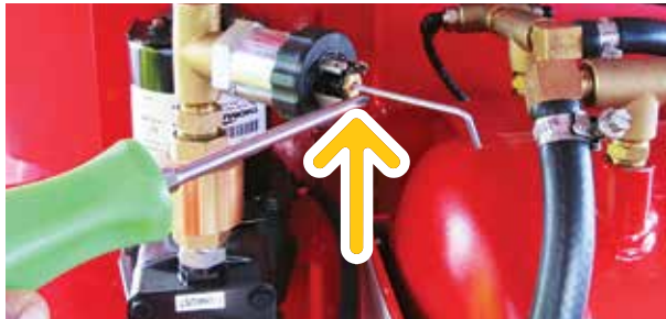
Adjust maximum pressure (100 psi) using the centre hole & allen key [shown]
