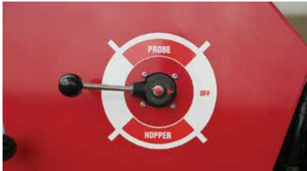
Rotate the Pressure valve to "Off" position
