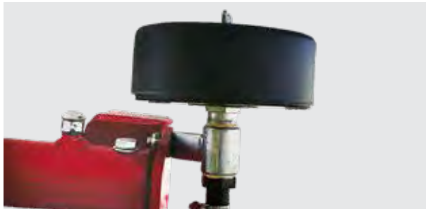
Clean the compressor air filter regularly
