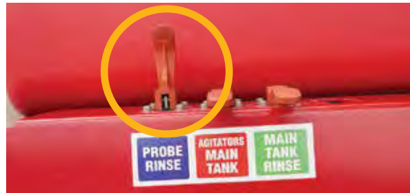
Open the "Probe Rinse" Valve
