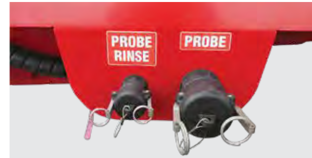
Connect the Probe Rinse & Probe" hoses
