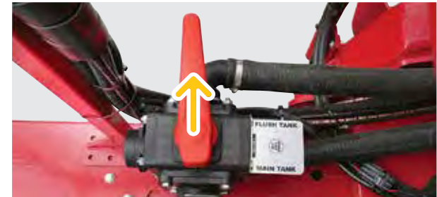
Rotate the Tank Selection valve to "Flush Tank" position
