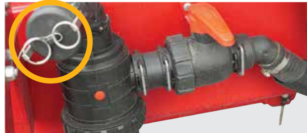
Remove the Camlock cap and connect the filling hose
