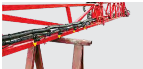
Reduce pressure on the inner boom springs by lowering the boom onto supports.
