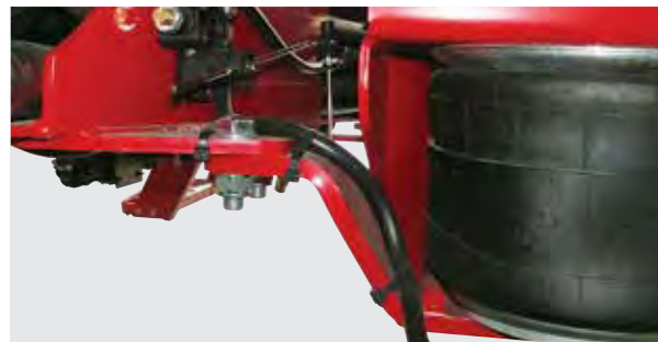
The ARDS drawbar inflatable airbag mechanism
