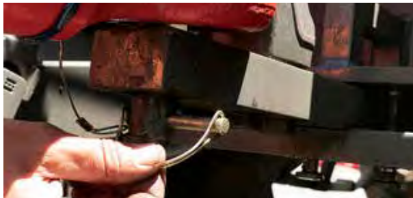
Ensure the drawbar pin is locked-in
