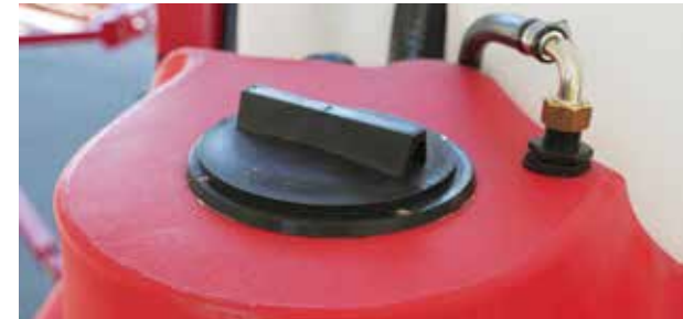
Replace Flush tank lids after inspection
