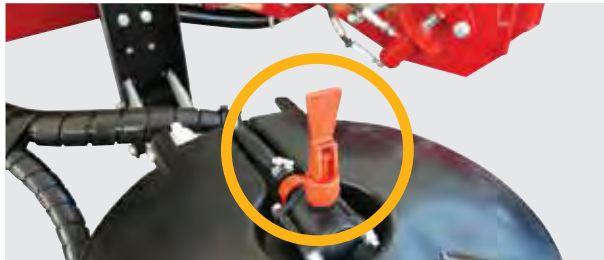
Lift the Hopper Rinse valve to rinse the hopper
