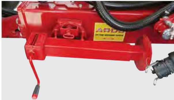
Rotate the hitch jack until it locks into the transport position
