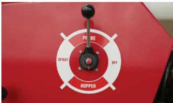
Rotate the Pressure Valve to "Hopper" position
