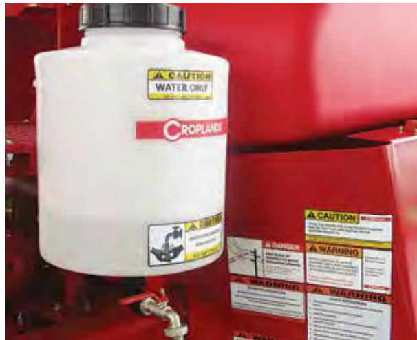
Fresh Water Tank: Fill Cap & Tap
