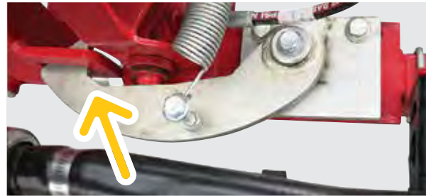
When locked the hook of the locking lever should be in contact with the front edge of the locking slot
