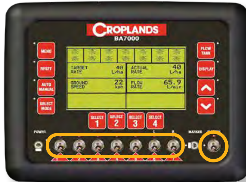
Switch Boom Sections On & Off several times.
