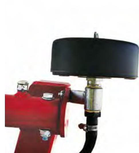
Compressor Air Filter (shown below on sprayer)
