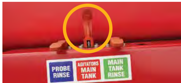
Open the Agitators Main Tank valve
