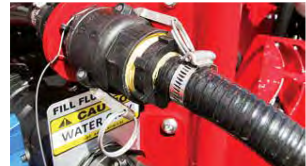
Connect the Envirodrum coupling to the flush fitting
