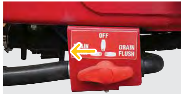
Open the "Drain Main" valve to drain remaining spray mixture from the Main tank
