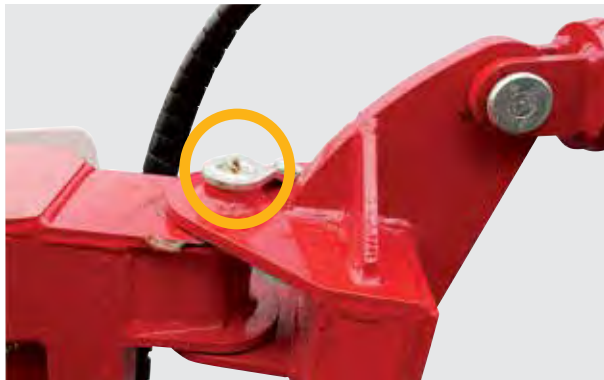
Grease all inner-fold pivot points
