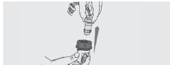
Separate the sensor from the Rapid Check unit
