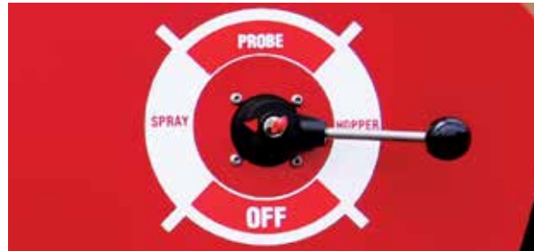
Rotate the Pressure valve to "Spray" position
