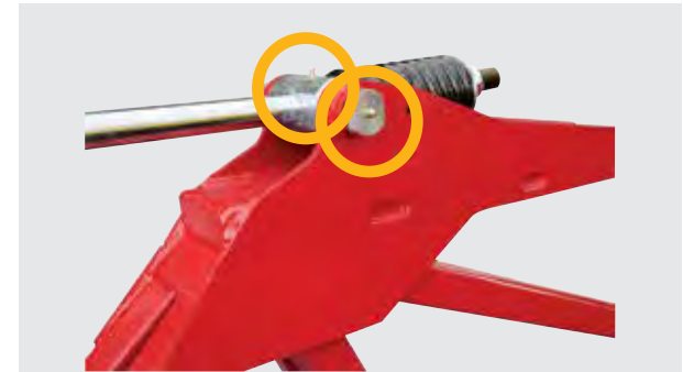
Grease the upper inner-boom hydraulic ram hinges
