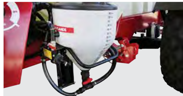
Return the hopper back to its transport position. Push the hopper inwards until the latch mechanism is engaged
