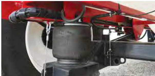
Air axle & levelling valve with adjustable linkage
