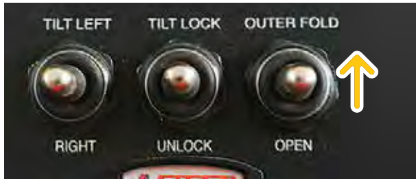
Push and hold to Outer Fold
