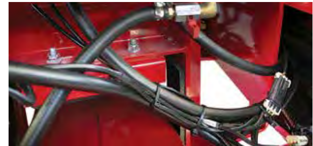
Start with 35mm gap between drawbar and the rubber stop plate above it.
