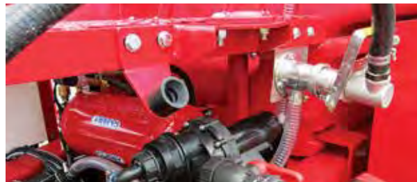
Open the ball valve to fill the hopper
