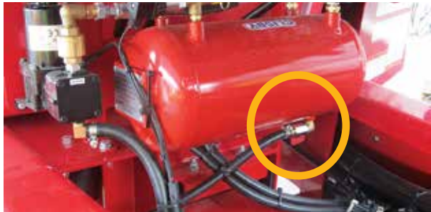
Drain moisture from the compressor tank regularly
