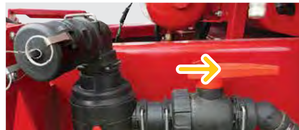
Open the Self-Filling valve
