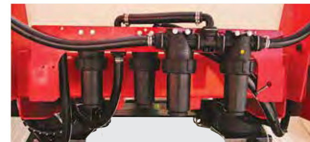
Clean the pressure filters
