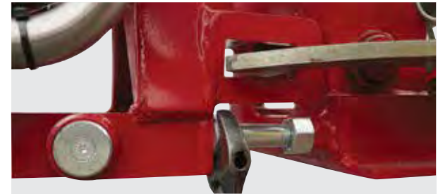
Adjust each bolt stopper to stop the boom at the position required
