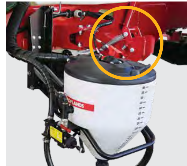
Release & lower the hopper
