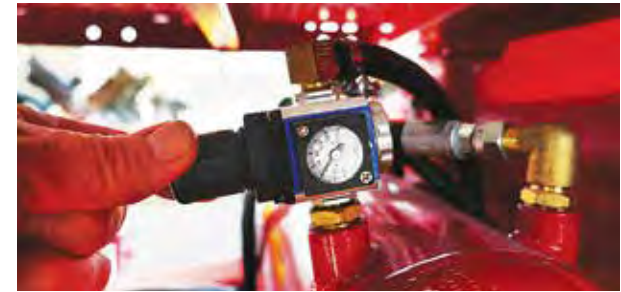
Adjust the ARDS drawbar airbag pressure to 40 psi using the pressure adjustment valve.
