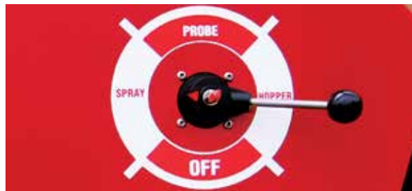
Rotate the Pressure Valve to "Spray" position
