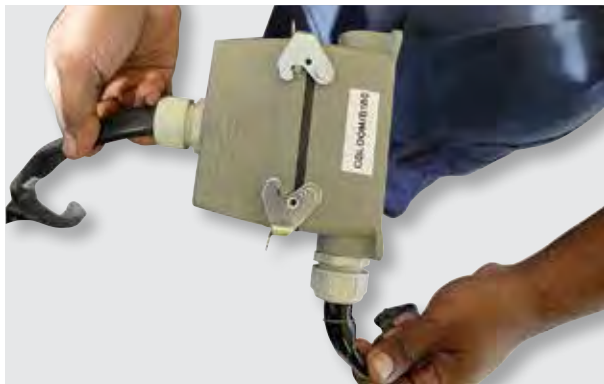
Rotate the clips & lock the connectors in place.
