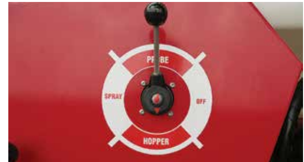
Rotate the Pressure valve to the "Probe" position
