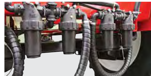
Remove & clean all pressure filters
