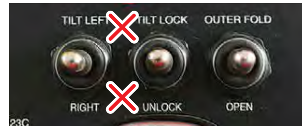
Push and hold to Right Wing to raise and down to lower
