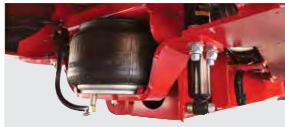
The ARDS drawbar airbag at the rear of the hitch
