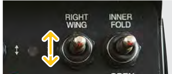
Push and hold to Right Wing to raise and down to lower
