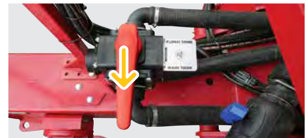
Rotate the Tank Selection valve to "Main Tank" position
