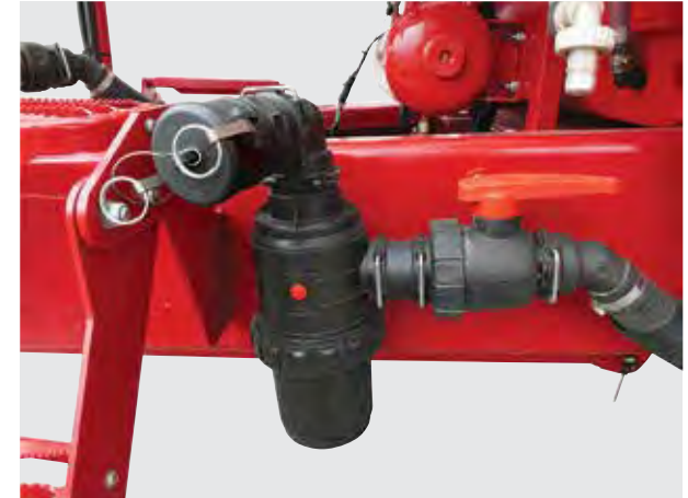
Main Tank Fill Connector (2")
