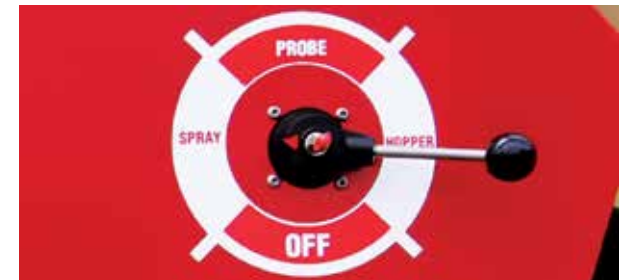
Rotate the Pressure valve to "Spray" position
