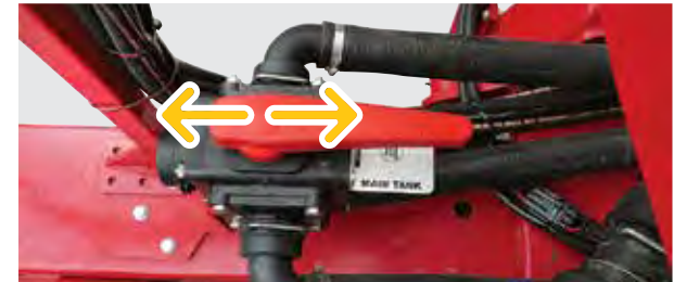
Rotate both Tank Selection valves to Off position (as shown - either direction)
