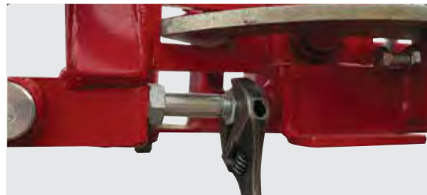
Unlock the bolt stopper lock-nut
