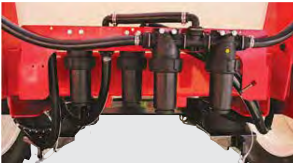
Clean the main pressure filters regularly
