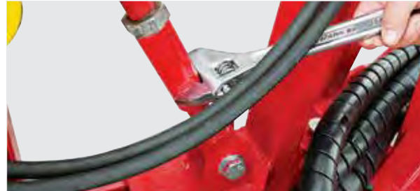
Adjust the turnbuckle sleeve until the centre section is level
