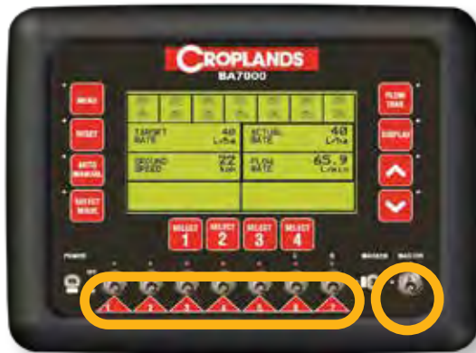
Switch ON the Boom Section toggle switches & Master switch
