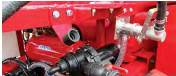
Attach the chemical transfer hose to the Camlock fitting
