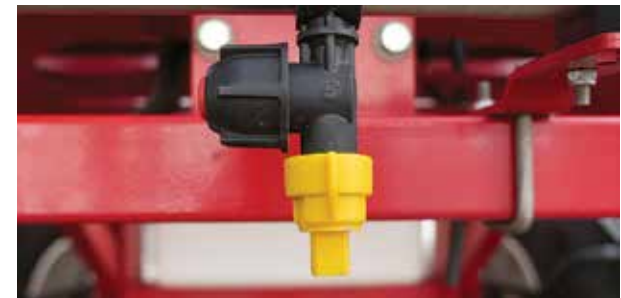
Remove & clean non-drip diaphragms
