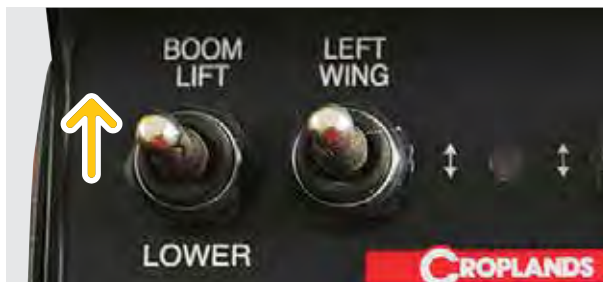
Push and hold to Boom Lift
