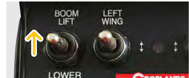
Push and hold to Boom Lift
