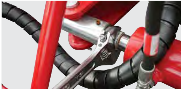
Inner-fold “Yaw” adjustment
