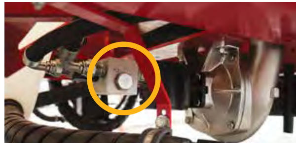
Hydraulic pump & over-run check valve assembly
