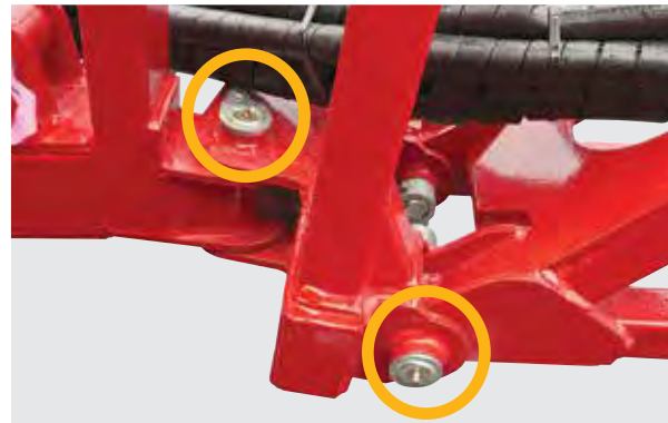
Grease the lower inner-fold pivot points
