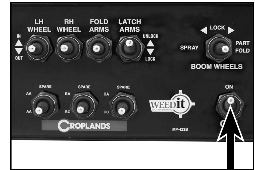
Move the MASTER switch up to ON position.
