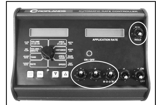
Boom switches on, master switch in hold.
