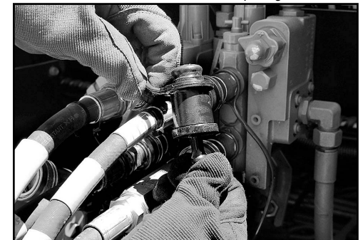
Join the male & female dust caps together.
