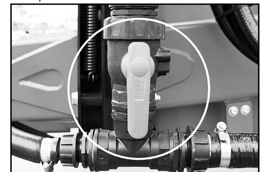
Open the Transfer valve to transfer the mixture.
