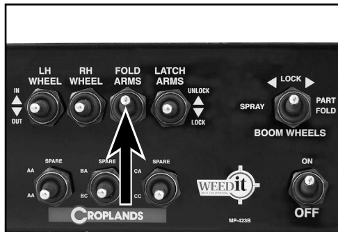
Hold UP the FOLD ARMS switch to fully close the stay arms.
