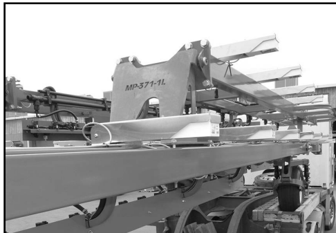
Outer booms on top of inner booms for transport.
