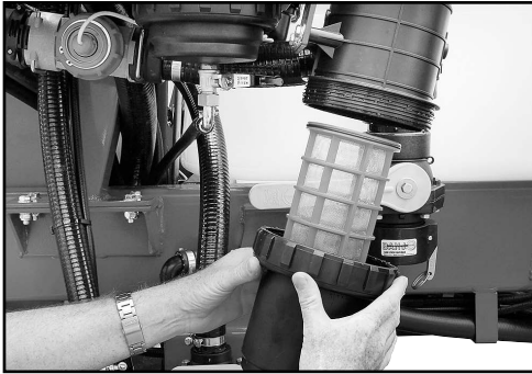
Clean the Fresh Water Fill filter regularly.
