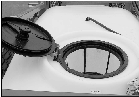
Open the Main tank lid for top-filling.
