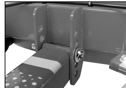
Remove the pin to adjust the hitch height as required.
