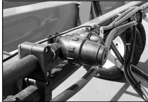
Clean Inline filters regularly (Dual Line Inline filter shown).
