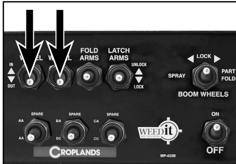
Hold DOWN both LH & RH WHEEL switches to rotate the main wheels to face forward in the direction of travel.
