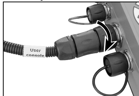
Rotate the ring-lock clockwise to lock the connectors.
