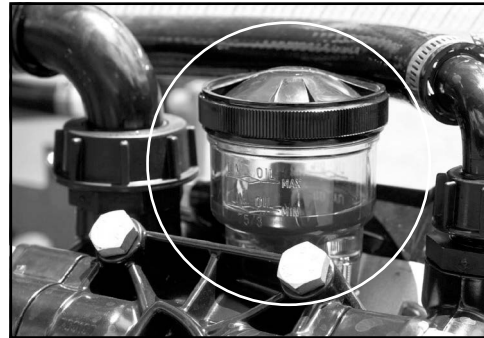
Check pump oil level.
