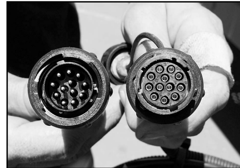
Align the Console cable connectors & push them together.
