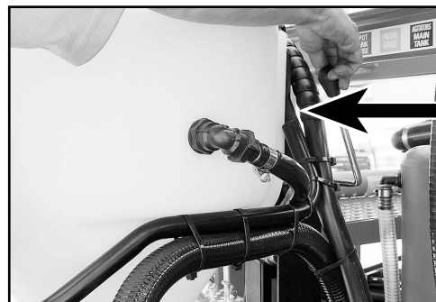
Pull the lever to unlock & lower the Chem-E-Flush.
