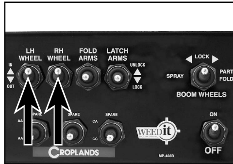
Hold UP both LH & RH WHEEL switches to rotate the wheels.
