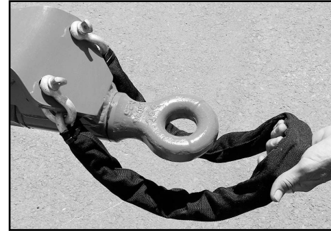
The transport safety chain must be fitted.
