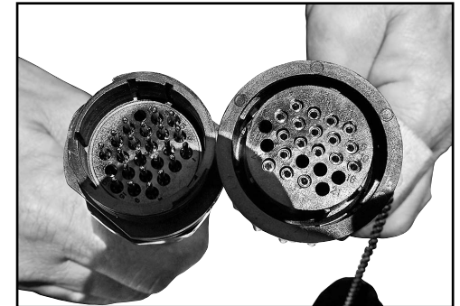
Align the Power cable connectors & push them together.
