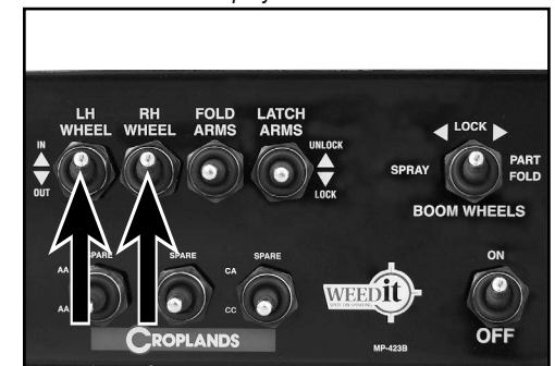
Hold UP both LH & RH WHEEL switches & slowly drive the sprayer forwards.
