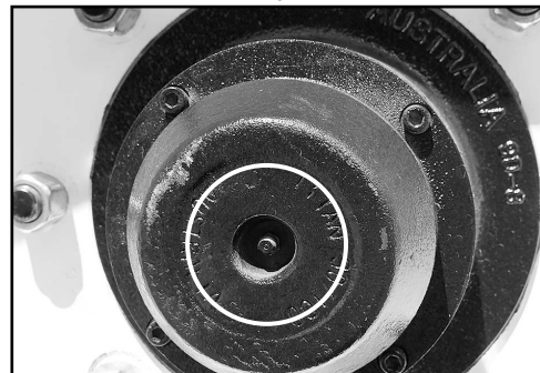
Main wheel grease point.
