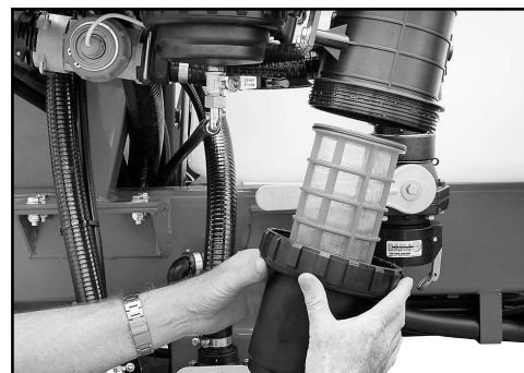
Clean the Fresh Water Fill filter.
