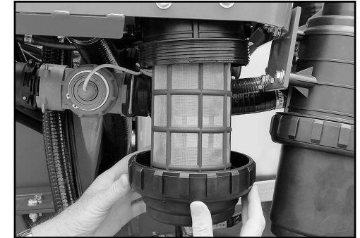
Check the Blanket Spray suction filter is clean.
