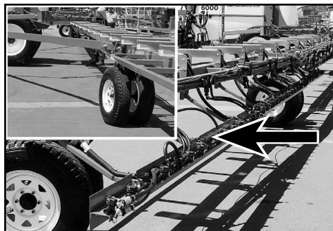
Inset: Main wing wheels in unfolding position. Rotate the wheels to face forward - in the direction of travel .
