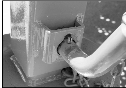
Rotate and align the pin & slot to remove the jack pin.
