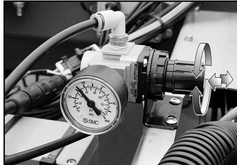
Adjust the air pressure at the rear of the Sprayer.
