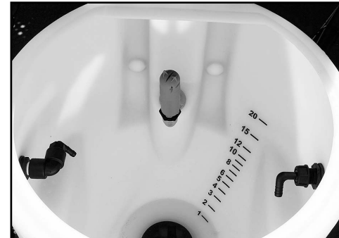
Open hopper lid & add chemical powder/liquid.
