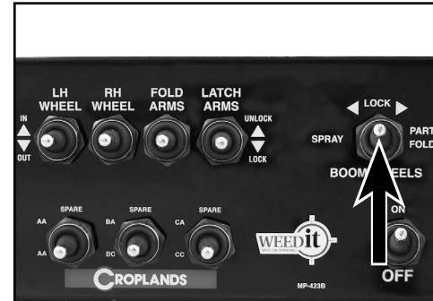
Move the BOOM WHEELS switch to LOCK position.
