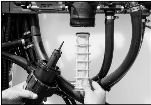
Remove and clean the pressure filter
