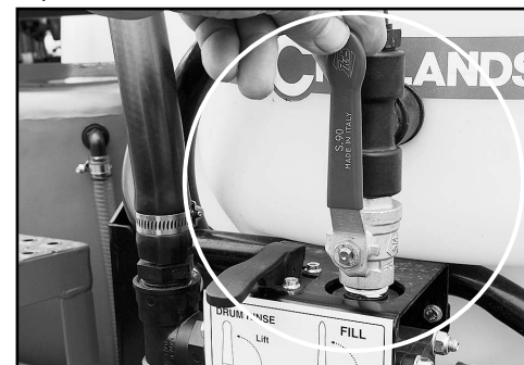
Open the Fill valve to add water and mix the chemical.
