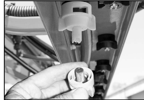
Clean nozzle filters regularly (Dual line nozzle filter only).
