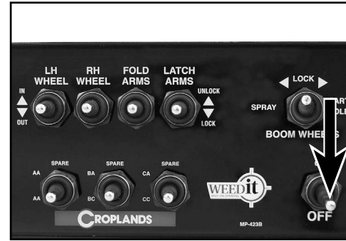
Move the MASTER SWITCH to OFF position to turn off the boom controller.
