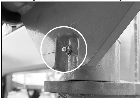
Lower grease point of the main boom hinge.
