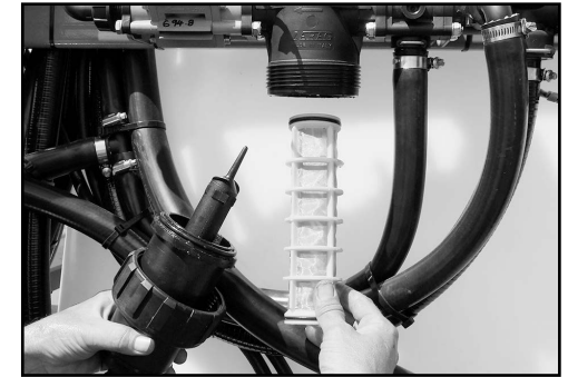
Clean the pressure filter regularly.
