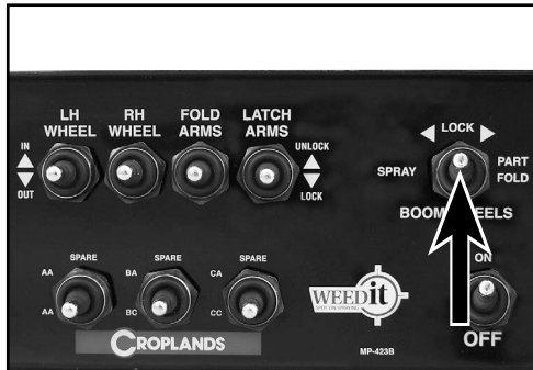
When the boom is half open, move the BOOM WHEELS switch to LOCK position.
