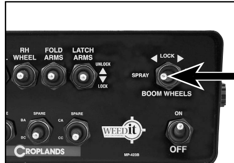
Move the BOOM WHEELS switch to SPRAY position.
