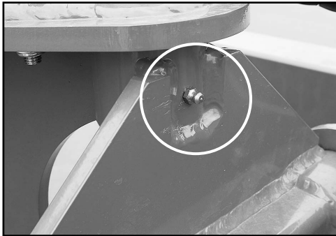
Upper grease point of the main boom hinge.
