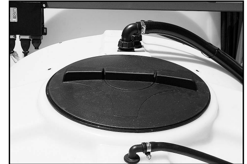
Open the Spot Water tank lid for top-filling.
