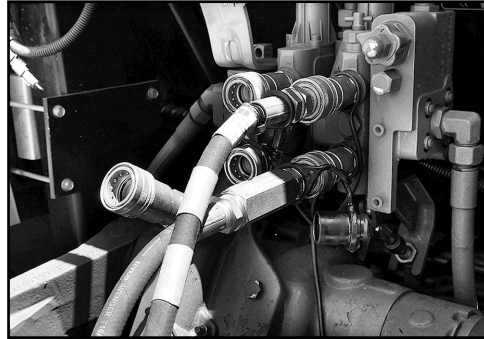
Connect the Trailing Boom hoses to the tractor.
