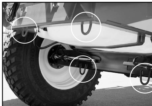
Use the tie-down points provided when transporting.
