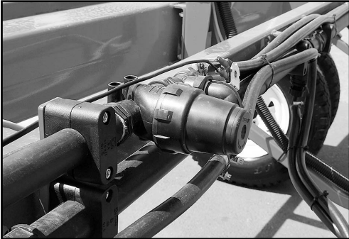
Clean Inline filters regularly (Dual Line Inline filter shown).
