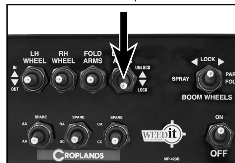
Hold DOWN the LATCH ARMS switch to lock the latches in place.
