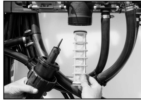
Clean the Blanket Spray pressure filter regularly.
