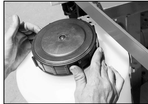
Open the Fresh Water tank lid for top-filling.
