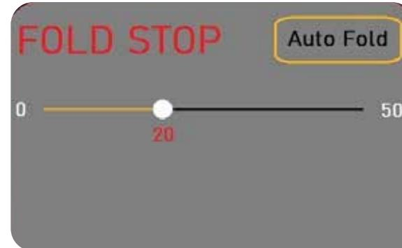
This can be a handy function when needing to part fold the Sprayer booms whilst performing tight headland turns.
