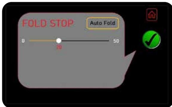
The AUTO FOLD button needs to be highlighted in Yellow to confirm the function is ON. The boom arms will now only fold out to the distance the row width is set to in the CAL screen.
