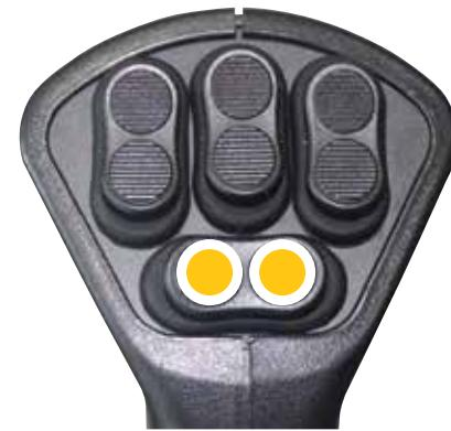
To change over or invert the Fan speed settings at the end of the completed row the operator will double click the left or right lower button on the Fusion Joystick control to perform the directional fan speed change.
