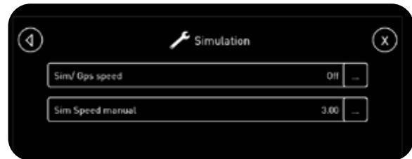
4. Press the SIM / GPS SPEED function and select ON.
