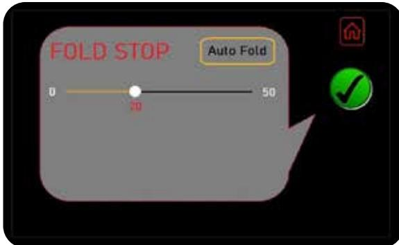
The AUTO FOLD button needs to be highlighted in Yellow to confirm the function is ON. The boom arms will now only fold out to the distance the row width is set to in the CAL screen.
