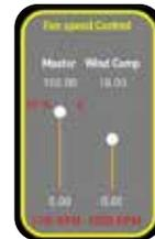
When satisfied with the Master Fan speed (MAX.) and Wind Comp Offset (MIN.) settings return to the Main Spray screen.
