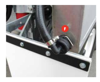
Each "boom" side (6mm) venturi requires around 24 L/min at 8 bar, and each "inner" (3.5mm) venturi requires 8 L/min at 8 bar system pressure (total of 64 L/min at 8 bar). The flow will vary up and down with pressure. Minimum recommended operating pressure is 5 bar.
