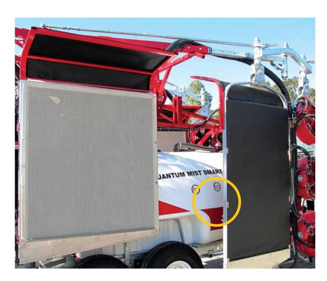
The photo left shows a Recapture sprayer in the maximum row width, parked position - there is none of the recommended screen angle (refer sketch on the previous page) in order to have some parked clearance between screen and tank (circled).
