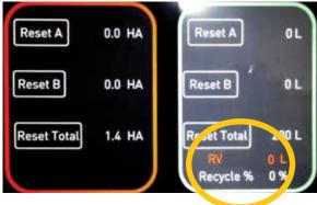
RV means Remaining Volume and this is what the tank level sensor is reading.
