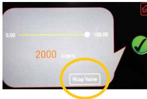
Remember to reset the tank volume value at the start of a spray session / after each filling. To set, slide the bar and watch the value. With a full tank the value should match the value presented by the load cell.
