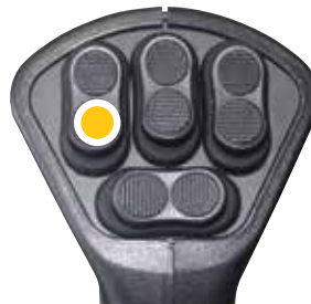
Section L is turned on/off with SW4
