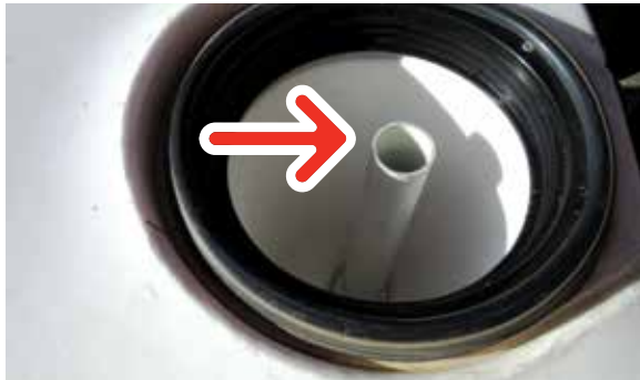
All sprayers have a Handwash tap positioned near the main filter (see orange arrow).
