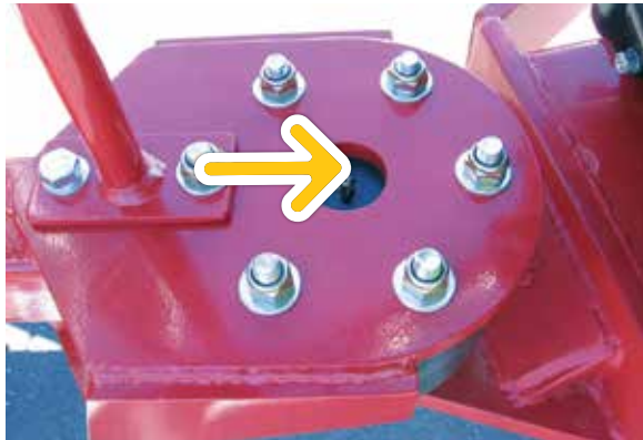
Grease the self-steer ball assembly regularly
