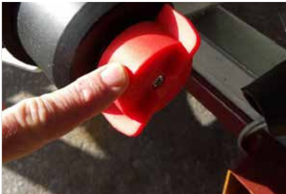
Twist plug to shut off liquid flow.
