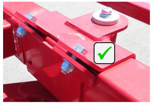
together. See above photo. Minimum torque for the pivot pin is 85 Nm.
