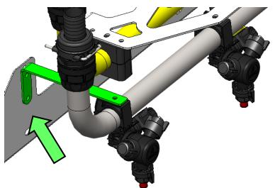
• Note the drawing assemblies incorporating the variable combinations of extra stiffening brackets and removal of unrequired tip guards have not yet been published. For dual line sprayers extra rigidity can also be achieved by using extra Stauff clamps (UP-434).
