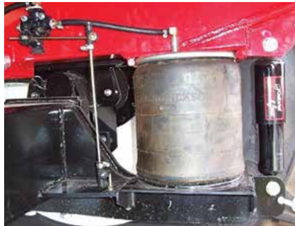
Adjust to ride height with main tank 50% full
