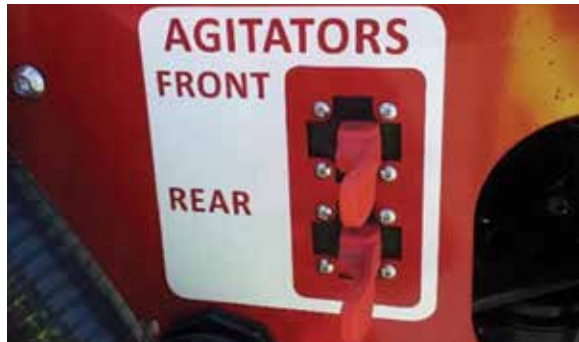
Agitators in the 'ON' position
