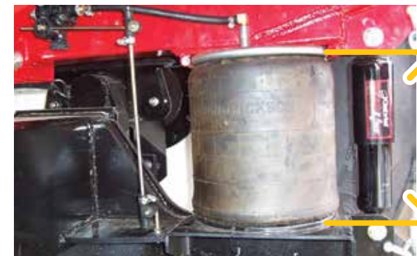
Adjust ride leveler valves as necessary to obtain correct Axle air bag ride height.
