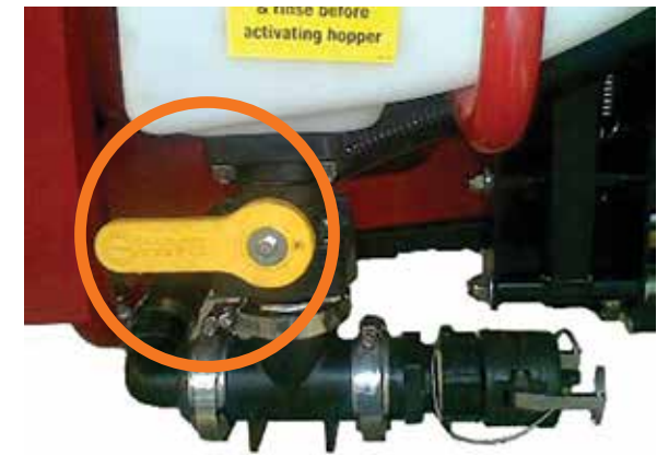
Chem-hopper drain valve
