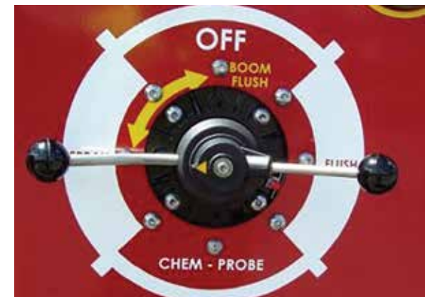
Pump suction valve (red arrow) to 'Flush' and Re-circ valve (yellow arrow) to 'Spray'
