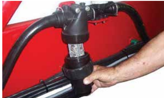
Clean pressure filter regularly
