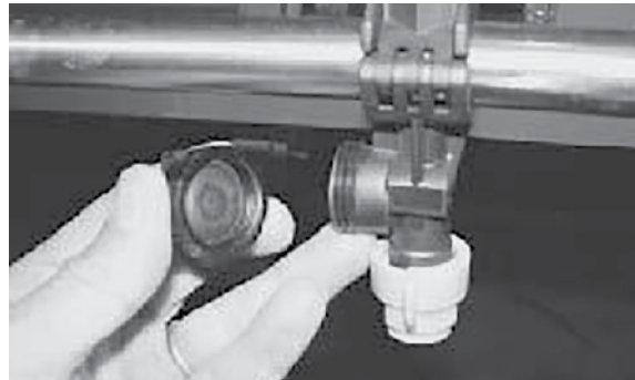
Remove & clean non-drip diaphragms
