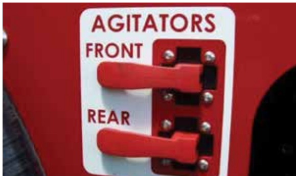
Tank Agitator valves in the "OFF" position
