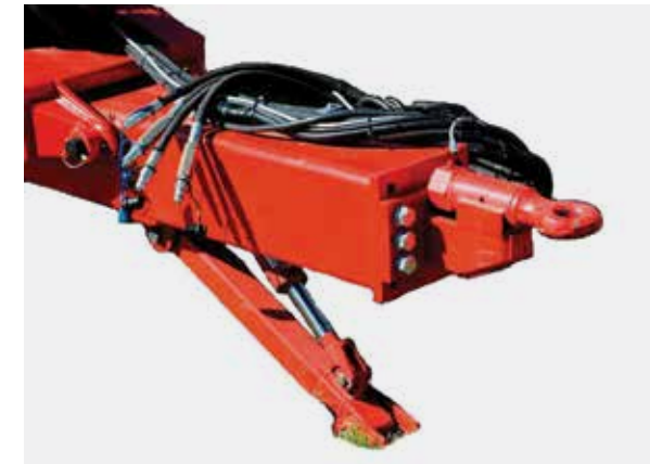
Adjustable height tow hitch
