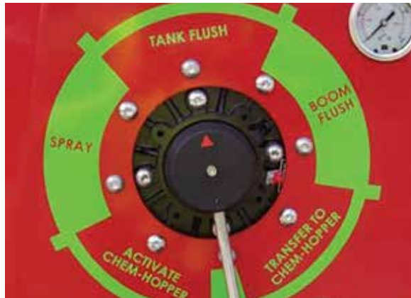
'Operation Valve' to 'Tank Flush' position
