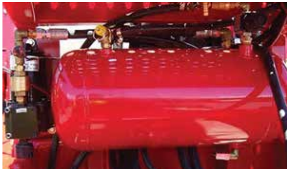
Air Reservoir and Compressor
