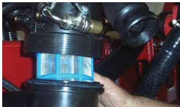
Clean suction filter
