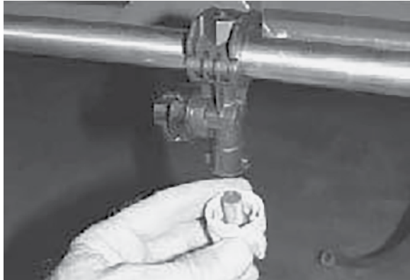
Clean nozzle filters regularly
