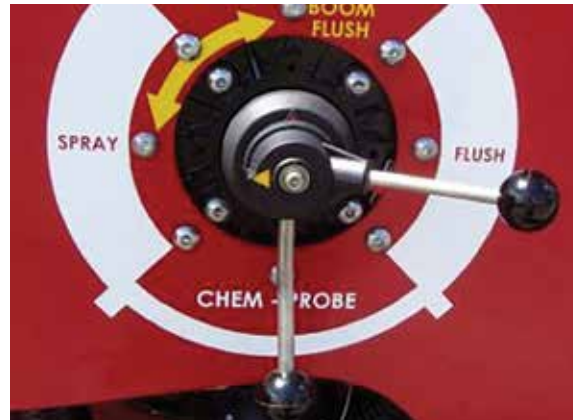
Spray mode lever to Boom Flush isolates sparge tube and diverts flow to the pump suction
