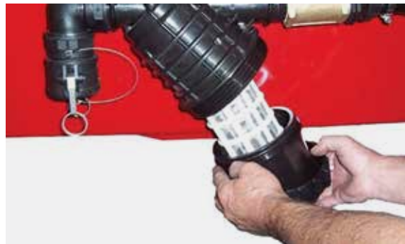
Clean the bottom-fill filter regularly
