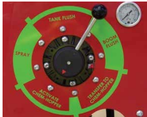
Operation Valve to Activate Chem-Hopper
