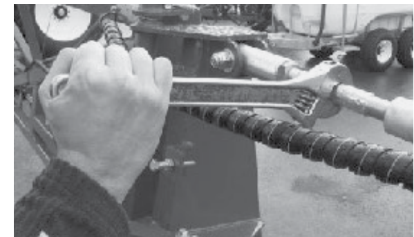
Adjust the sleeve until the boom is at the desired level then re-lock the lock nut to secure in place.
