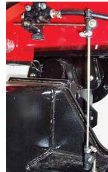
Loosen clamp on vertical rod to adjust
