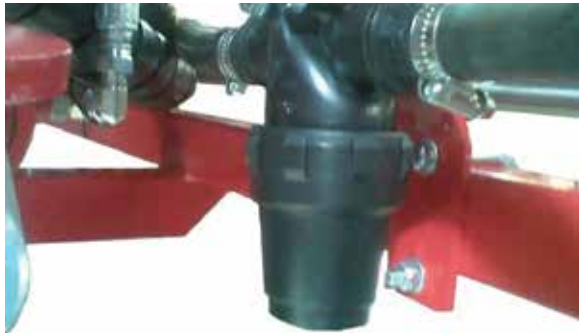
Remove and clean boom section filters
