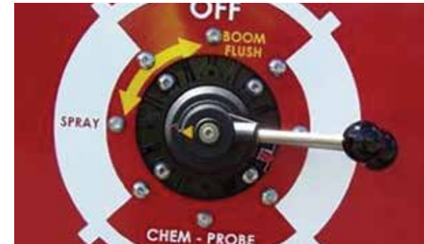
Pump suction valve (red arrow) to 'Spray' and Recirc valve (yellow arrow) to 'Spray'
