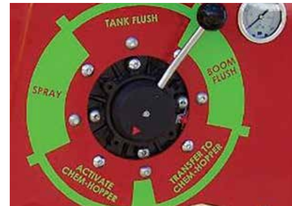
'Operation Valve' to 'ACTIVATE CHEM-HOPPER' position
