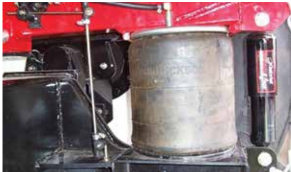
Axle Air-Ride Suspension System
