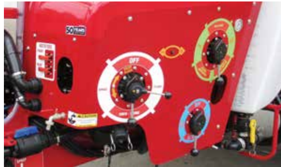
Sprayer control panel
