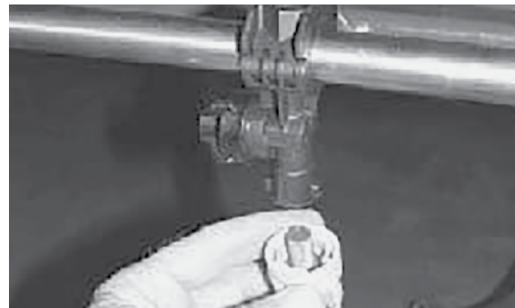
Ensure nozzle filter size suits nozzle
