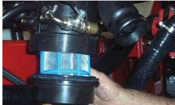
Drain Filter housing before opening
