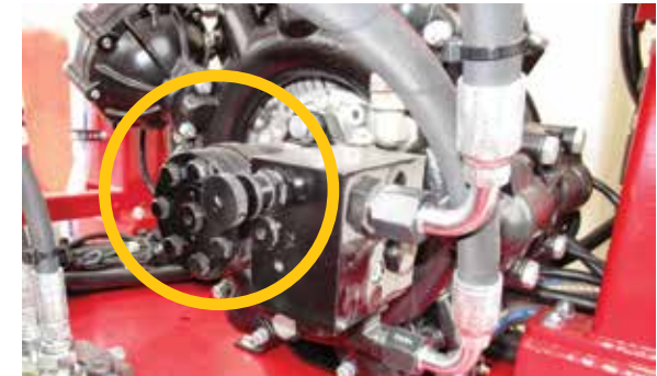
Spray pump rpm flow control valve
