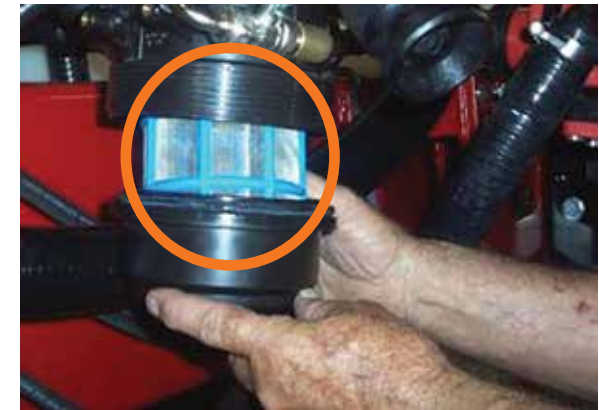
Clean the suction filter regularly
