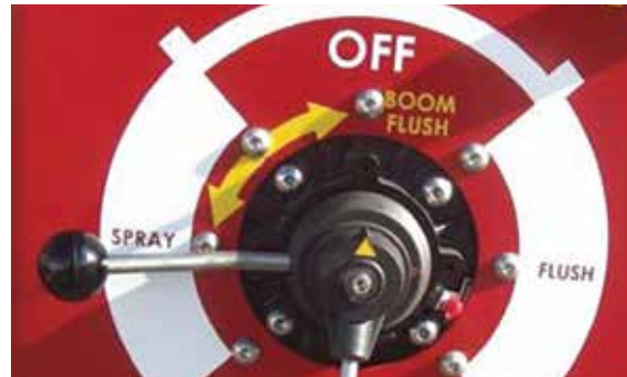
Suction valve to FLUSH, Re-circ to BOOM FLUSH
