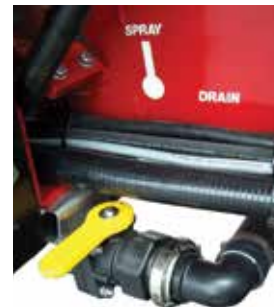
Tank drain valve in spray position
