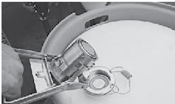
Unclip Micromatic coupler from Envirodrum
