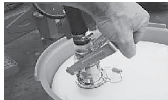
Clip the Micromatic coupler to the Envirodrum
