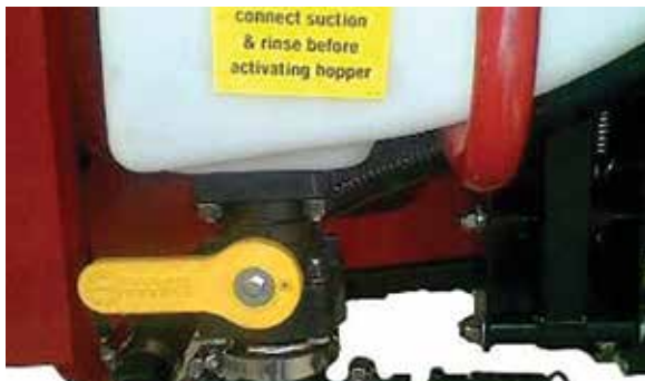
Open chem-hopper transfer valve
