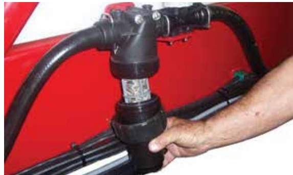
Clean main pressure filter
