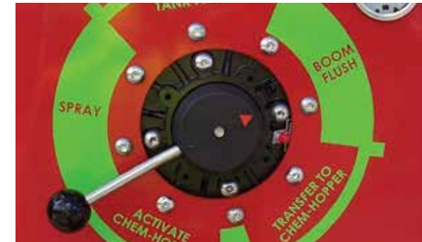
Operation Valve to BOOM FLUSH
