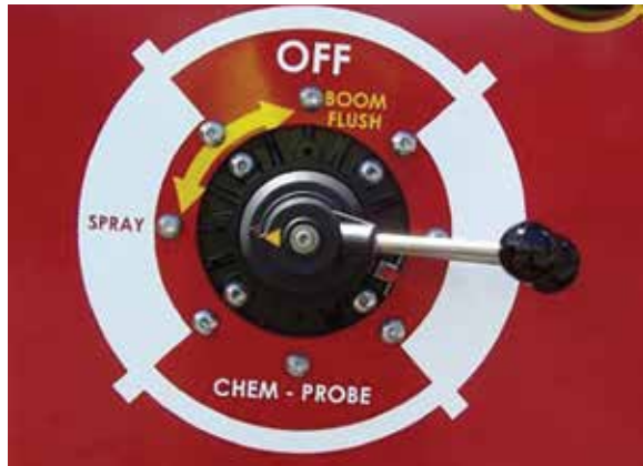
Spray mode with re-circ lever (yellow arrow) to Spray diverts flow to the Sparge Tube
