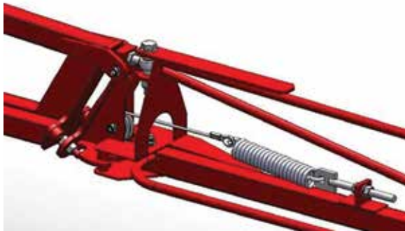
Adjust breakaway spring tension as necessary
