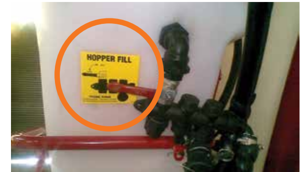
Fill Chem-hopper Valve
