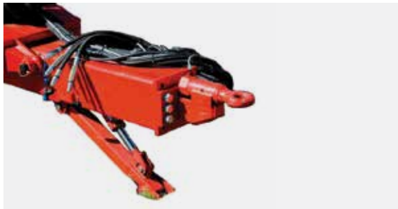
Lower Jacking leg for parking
