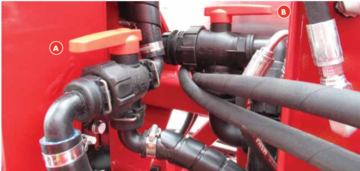
A Ball valve A (bleeders) is shown in the prime / recirculate / flush to main tank position. B Ball valve B (metering) is shown in the prime / recirculate / flush to main tank position.
