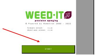
It takes approximately 10 seconds before the WEED-IT console is started. During this time, the WEED-IT ECU and the WEED-IT console exchange data, like the number of connected sensors, the selected spray mode and nozzle, the selected preset and the selected margin.
