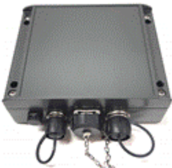
Figure 4-15 Section Communicator box
