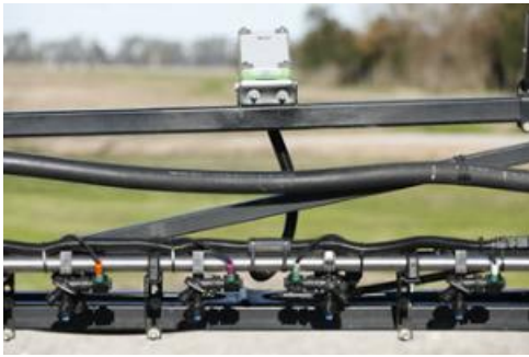
Figure 4-10 WEED-IT detection sensor; the sensor window must face down.
