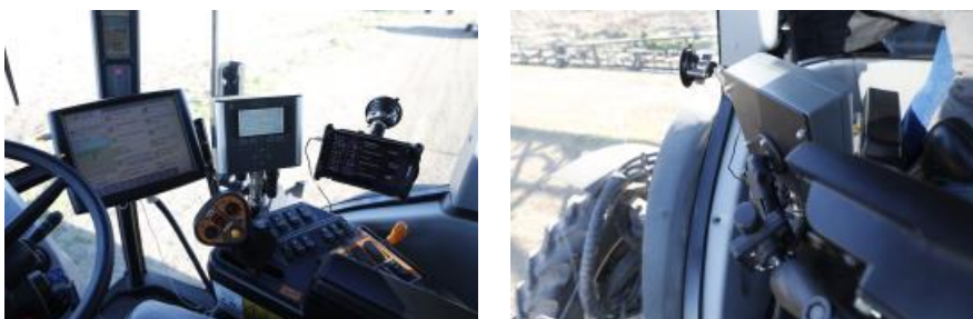
Figure 4-5 Use the mounting kit, including the RAM mount, for installing the User console in the cabin
