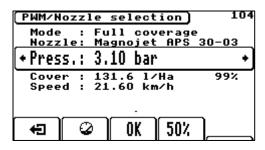
9. Use the **Left/Right** navigation keys to select the preferred pressure. If you press the gauge icon (F2), the nominal pressure that belongs to the nozzle will be set. For most nozzle types this is 3.00 bar.
