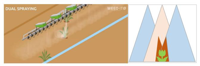
The Dual Spraying mode is an unique spray tech feature. It combines full coverage spraying with spot spraying by applying a low cover application rate, like 30 l/ha, followed by a spot application rate, like 100 l/ha, when a plant is detected. Unique is that both cover and spot application rates are regulated via PWM.
