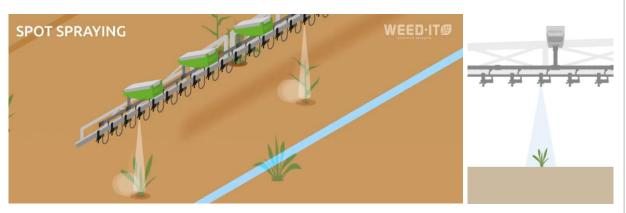
In Spot Spraying, the WEED-IT Quadro only sprays the green plants that are detected with the chlorophyll fluorescence principle. WEED-IT regulates the application rate via PWM, considering a constant pressure. The spot spraying application can be seen as a band application with a single nozzle. Therefor the spot spraying application rate is calculated as:
