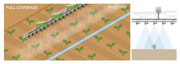
In Full Coverage spraying mode, the WEED-IT Quadro operates like a normal sprayer. The only difference is that the WEED-IT Quadro regulates the application rate via PWM, considering a constant spray pressure. The cover application rate is calculated as:
