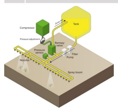
Figure 3-2 Flow in a standard WEED-IT installation
