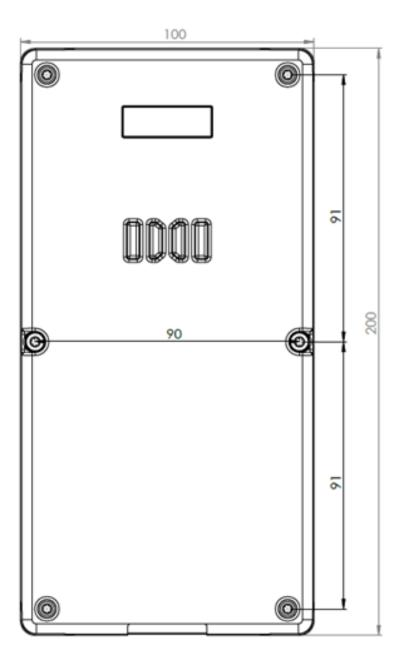
Figure 9-1 Sensor back housing dimensions [mm]
