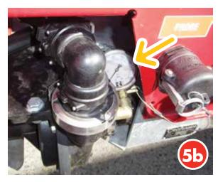
6. Adjust the Spray pressure via the pressure regulator a. whilst monitoring the main pressure gauge
