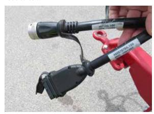
Connect the rectangular plug to the Switch Box.
