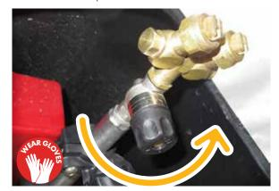
Clean the filter before or after running the spray system. **Wear GLOVES and appropriate PPE.**
