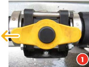
1. Main tank ball valve set to the Pump / Spraying (left)
