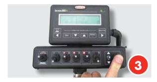
3. Go to the Arag controller, turn on the master on/off switch and all three boom sections. Hold the manual pressure switch up for 5 seconds to set maximum pressure with all boom sections spraying. Note the photo above is of a 5 section controller (using middle 3 sections).
