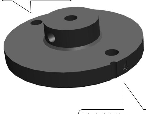
Link rod to the Right boom arm mounts this side - note the small cut-away and number 4 stamped into the edge.
