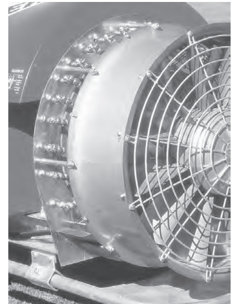
820SV fan assembly with stainless steel air straightening vanes - 20 roll-over nozzle assemblies - 10 each side.
