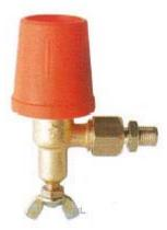
For use on vineyard orchard sprayers. Spray pattern adjustable via wing nut rotation. With the "TURBO" protection allows an excellent micronization and the complete and even foliage coverage. The spray tip can be easily cleaned and replaced with out tools. Fast nozzle orientation with the adjustable connection.
