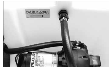
Refit the filter & suction line (UM70 only).
