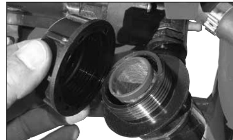
Remove & clean the suction line filter, then reassemble.
