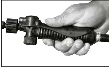
Hold down the hand grip lever to activate & prime the pump.
