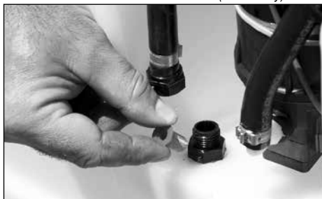
Remove and clean suction filter (UM70 only).
