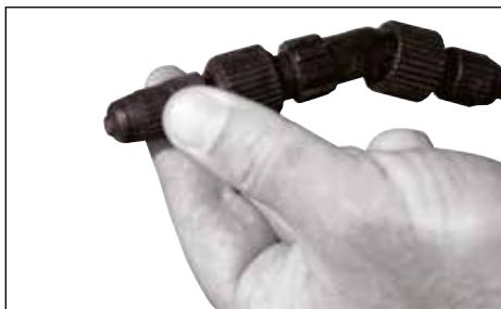
Adjust the variable cone nozzle for the required spray pattern.
