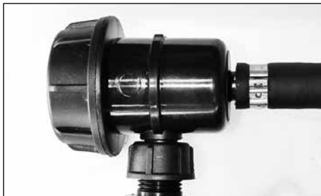
Check & clean the suction filter.
