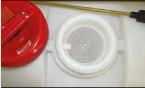
Fill the spray tank with the lid filter in place.
