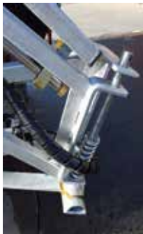
Fig 1: MAX boom breakaway - crush point.
