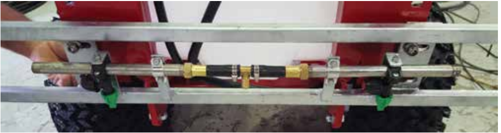
Mount the centre section to your sprayer using the bolts & brackets supplied.
