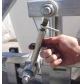
Fig 5: Rotate the adjustment sleeve with through-pin to adjust the strut either longer or shorter to level the boom.
