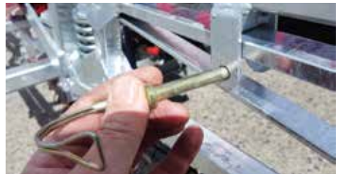
When folding up outer arms, ensure the pins are used to secure the outer arm in the folded position
