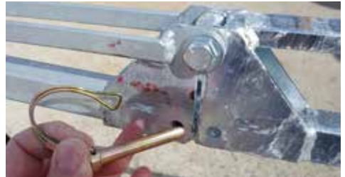
Use pins supplied on GEX boom to secure manual-fold outer wings
