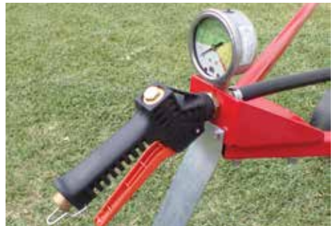
Connect your inlet spray hose to the fitting on the back of the trigger shut-off assembly
