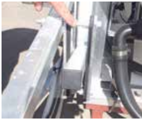
Fig 2: Shows a side view of the channel the boom runs in and the adjustable guides that keep the boom in the correct plane during operation.
