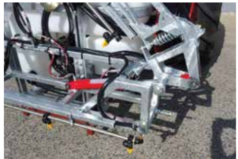
Fig 3: Hydraulic fold points are dangerous crush points. Keep hands clear at all times
