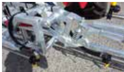
Fig 2: GEX boom fold point - keep hands clear during folding
