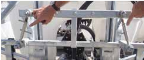
Fig:1 Shows the self-lever with the adjustable struts in place of the hanging points.
