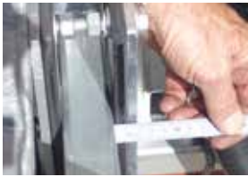
Fig 8: Adjust the gap accordingly – ensure the guides do not “bind” the boom. Ideal clearance is around 1mm.
