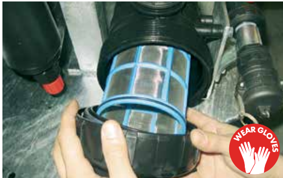
Remove the outer filter screw and bowl
