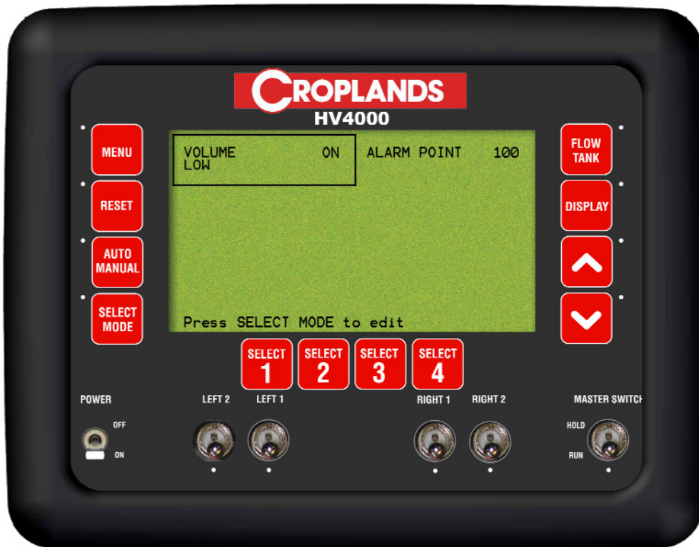
Tank Alarms Screen
