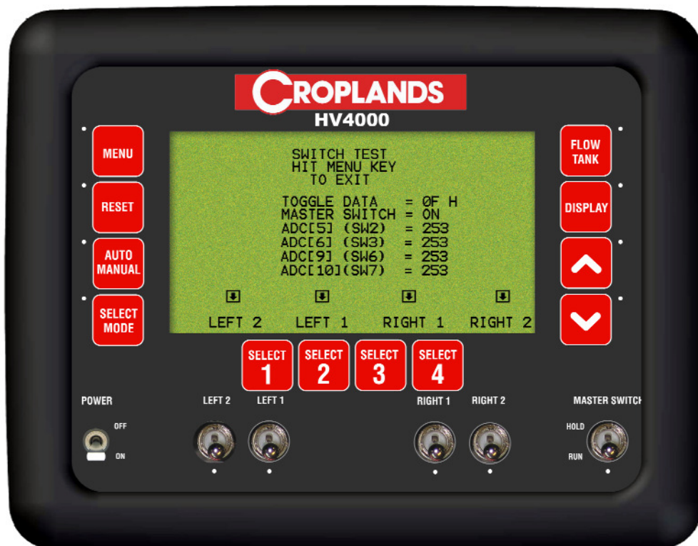
Switch Diagnostics Screen
