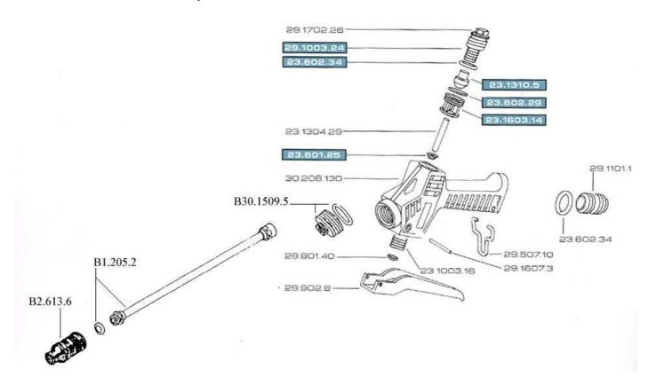
A valve kit for the RL10 spray gun is available under the following part number **B23.302.12** A complete repair kit for the spray gun is also available under the following part number **B30.302.25**.
