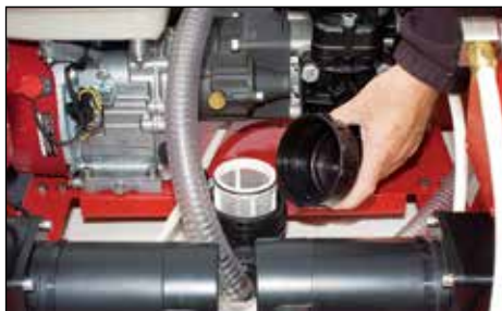
Check & clean the suction filter.
