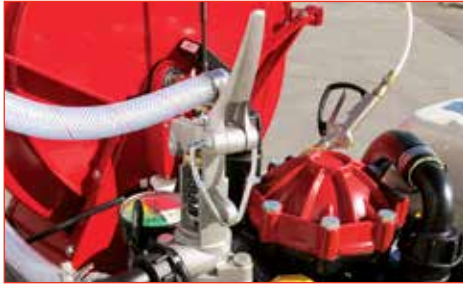
Pump in by-pass & closed position (levers up).
