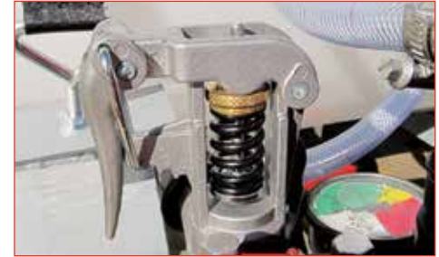
Pressure controller lever - pressure adjustment.
