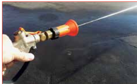
Turbo400 spray gun with narrow cone adjustment for spraying targets further away, such as down a bank or gully.
