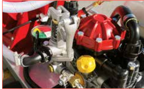
Pump in operating & open position (levers down).
