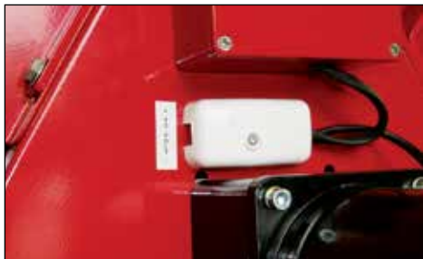
Hard wire to the reel's connector box.
