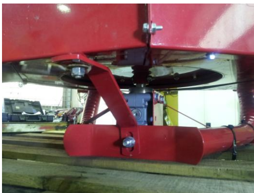
Above – bottom rear support bracket bolted in place
