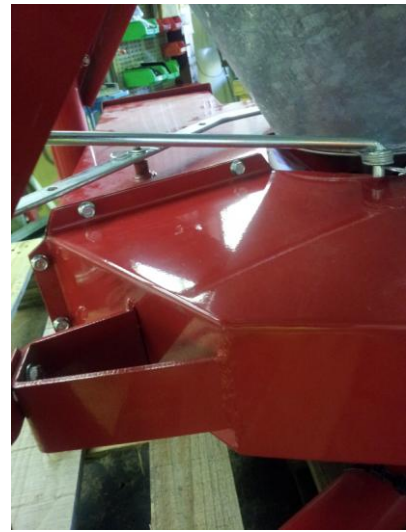
Right – front shot of 2 halves of conveyor bolted together
