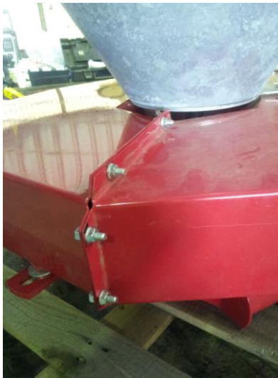
Left – back shot of 2 halves of conveyor bolted together
